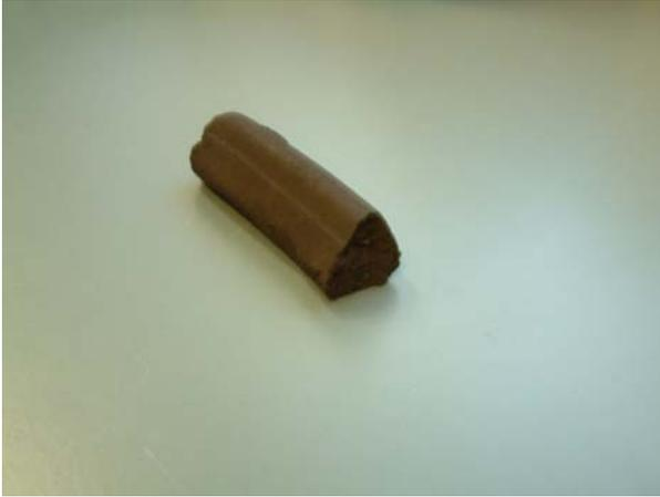
**Figure 22 Coal Specimen for deformation test**
