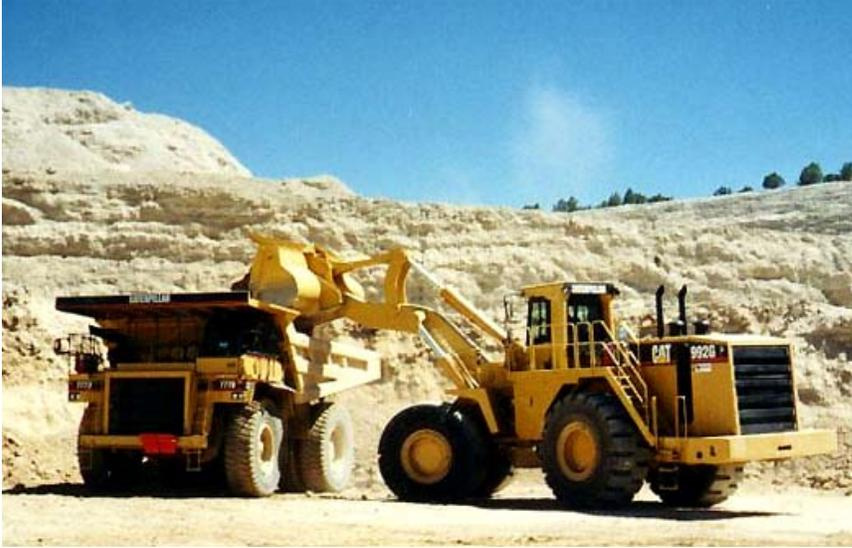
**Figure 10 Coal being filled into a rear dump truck**
