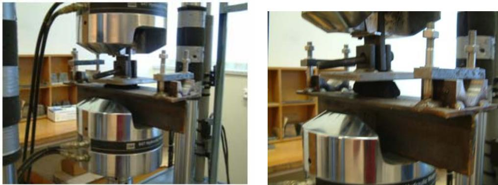
**Figure 23 Multi Purpose Hydraulic Wedge Grip, model MTS 647**
