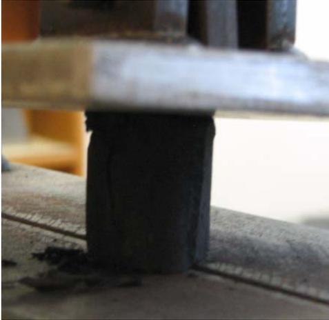
**Figure 27 Vertical Cracks in Coal Specimen**
