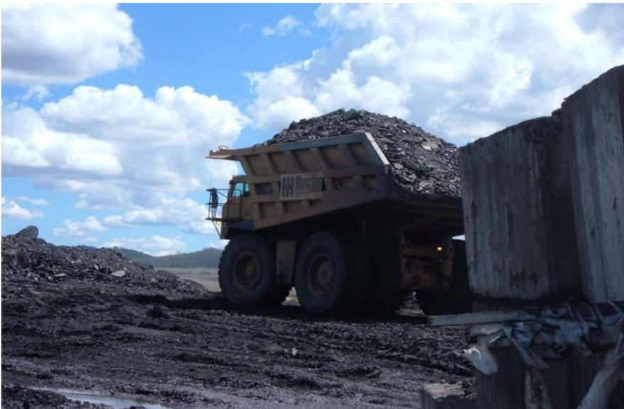
**Figure 11 Truck dumping coal into grizzly**
