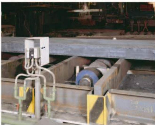
▲ Extreme operating conditions exist in steel making plants – the WT 45 photoelectric proximity switch is ideal for many applications, such as detecting metal sheets before they are wound onto coils.
