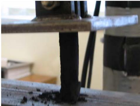
**Figure 26 Vertical Coal Deformation Test Procedure**
