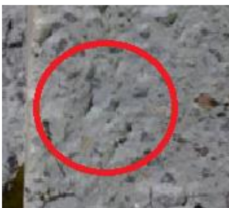
Figure4.2.11; image of mark left after bond between mortar and aggregate fails
