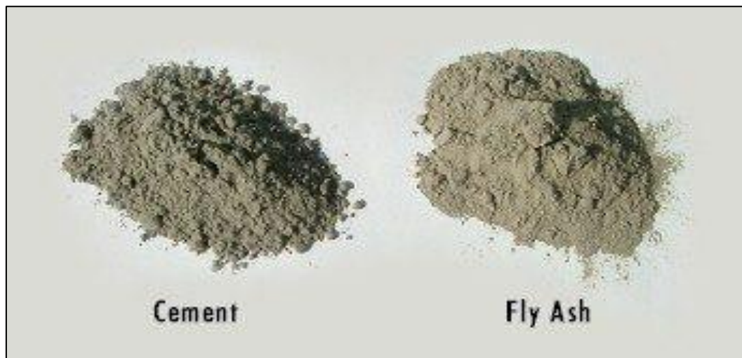
Figure 2.2.2; Portland Cement versus Fly Ash (visual Similarities')
