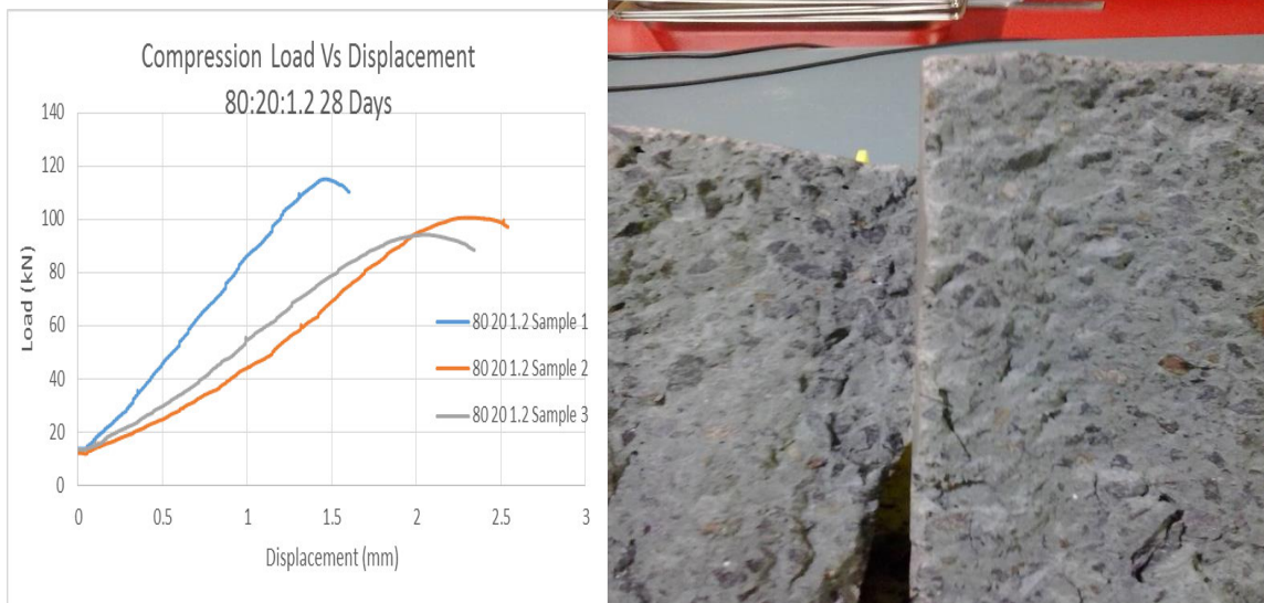
Figure 4.2.10; 80:20:1.2 28 DAY compression Results with sample photograph
