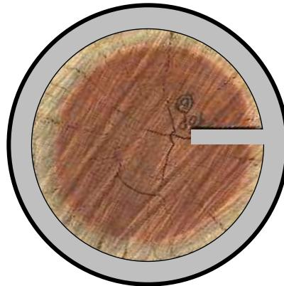
Figure 3-12 - 2/3 Radius defect with underwater cementitious grout and FRP wrapping
