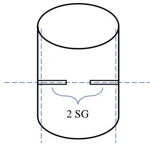
Figure 3-26 - Wrapped horizontal strain gauges
