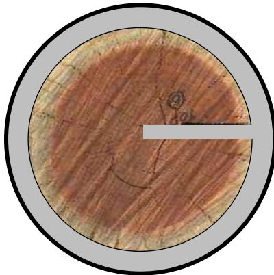
Figure 3-11 - Radius defect with underwater cementitious grout and FRP wrapping
