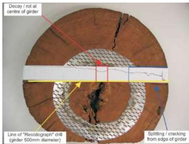
Figure 2-8 – Resistograph scan (a) (Timber Bridge Maintenance Manual 2005)
