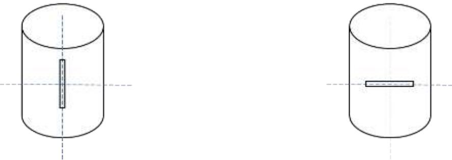
Figure 3-27 - Wrapped duplicate sample vertical strain gauge
