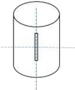
Figure 3-25 - Wrapped vertical strain gauge
