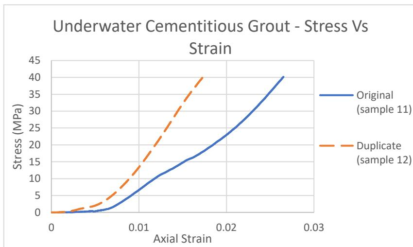
Figure 4-28 - Underwater Cementitious Grout - 1/3 radius defect
