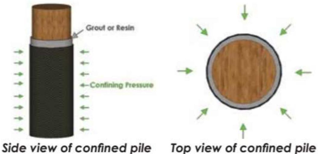
Figure 2-12 - Schematic view of rehabilitation technique
