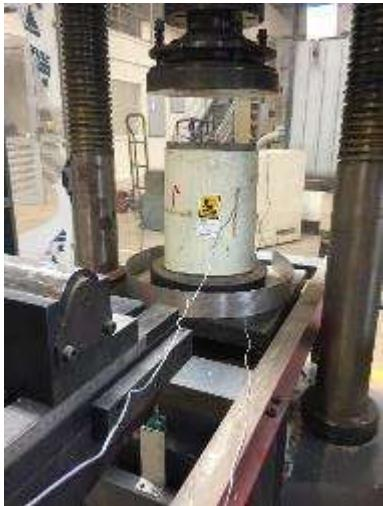
Figure 4-1 - SANS compression testing machine (a)
