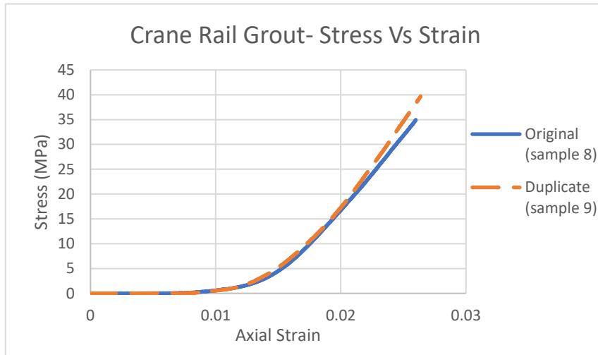
Figure 4-24 - Crane Rail Grout - 2/3 radius defect
