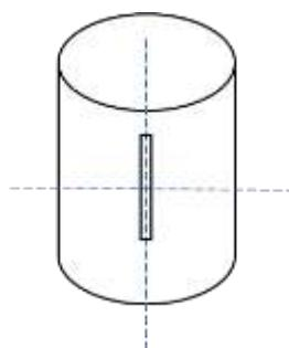
Figure 3-23 - Vertical strain gauge orientation
