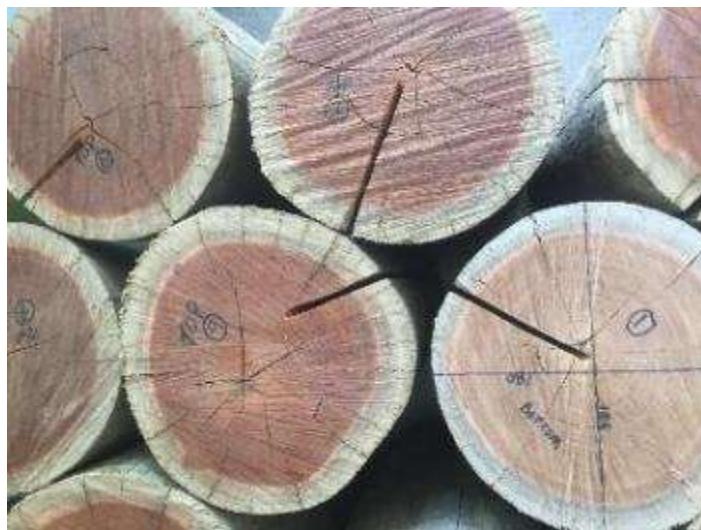
Figure 3-3 – Three different split depth defects
