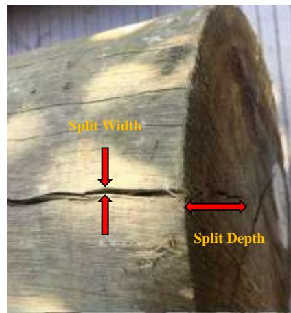
Figure 2-5 - Splitting along the grain
