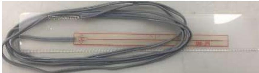
Figure 3-22 - Tokyo Sokki Kenkyo strain gauge
