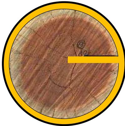
Figure 3-8 - Radius defect with crane rail grout and FRP wrapping
