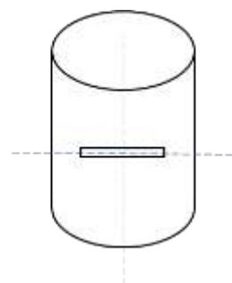
Figure 3-24 - Horizontal strain gauge orientation
