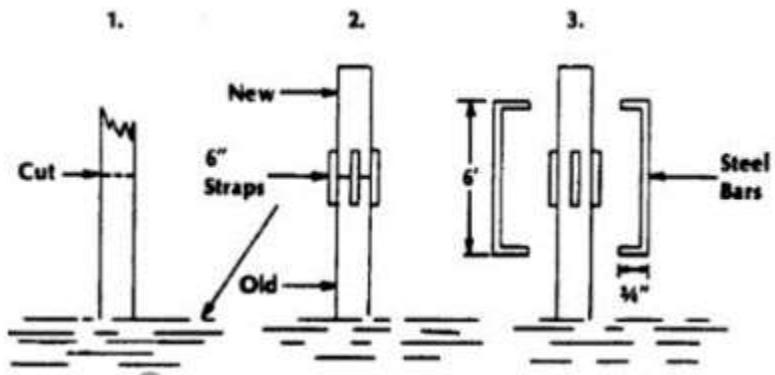
Figure 2-11 - Step - by - Step splicing procedure (Mohammadi et al. 2014)
