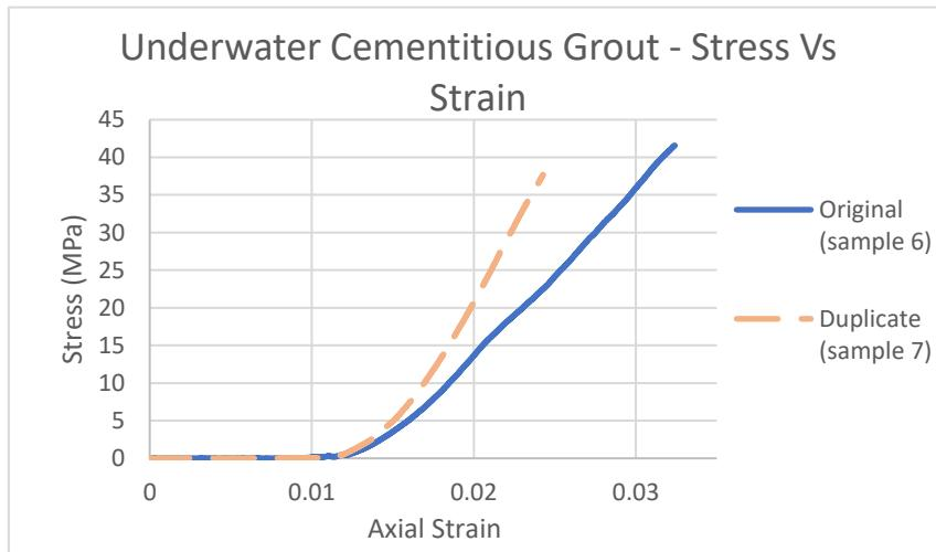
Figure 4-22 - Underwater Cementitious Grout - 2/3 radius defect
