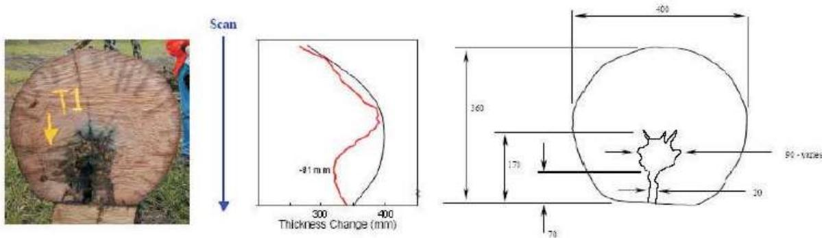
Figure 2-7 - "Lixi Profiler" scan
