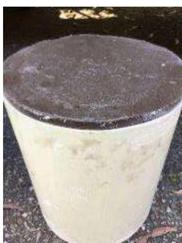
Figure 3-18 - Crane rail grout filler material
