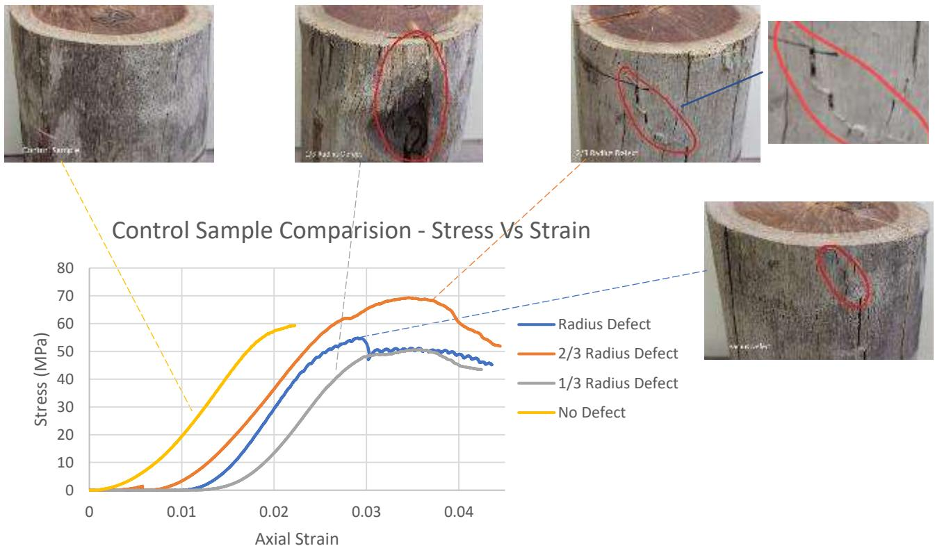
Figure 4-5 - Stress vs strain failure mode specimens
