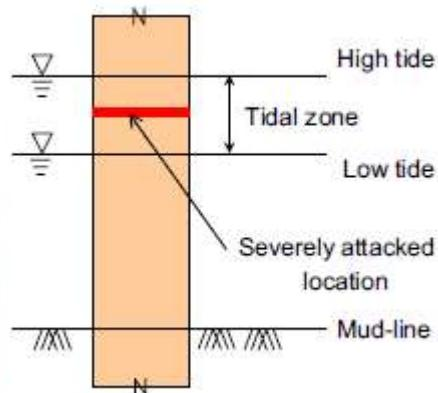
Figure 2-4 - Marine Bore Attack locations (M. N. Nguyen et al. 2007)
