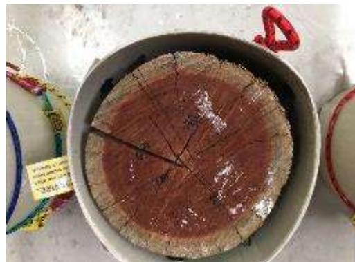
Figure 3-17 - Top view before annulus filled
