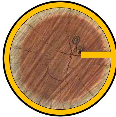
Figure 3-9 - 2/3 Radius defect with crane rail grout and FRP wrapping
