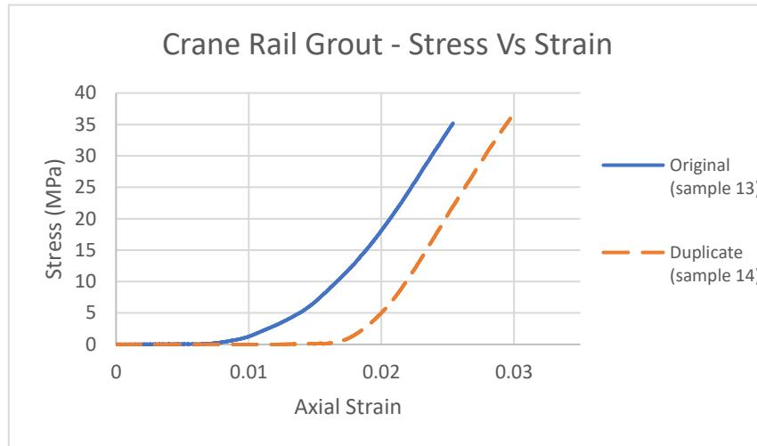
Figure 4-30 - Crane Rail Grout - 1/3 radius defect
