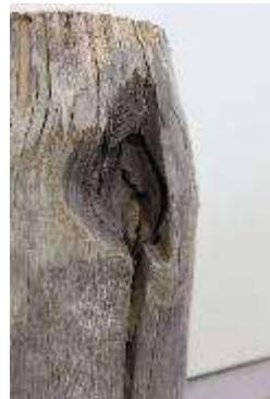
Figure 4-10 - Observed split in 1/3 radius defect sample
