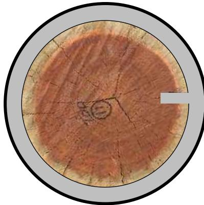
Figure 3-13 - 1/3 Radius with underwater cementitious grout and FRP wrapping
