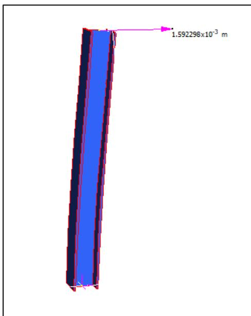
Figure 52: Column serviceability Model 1
