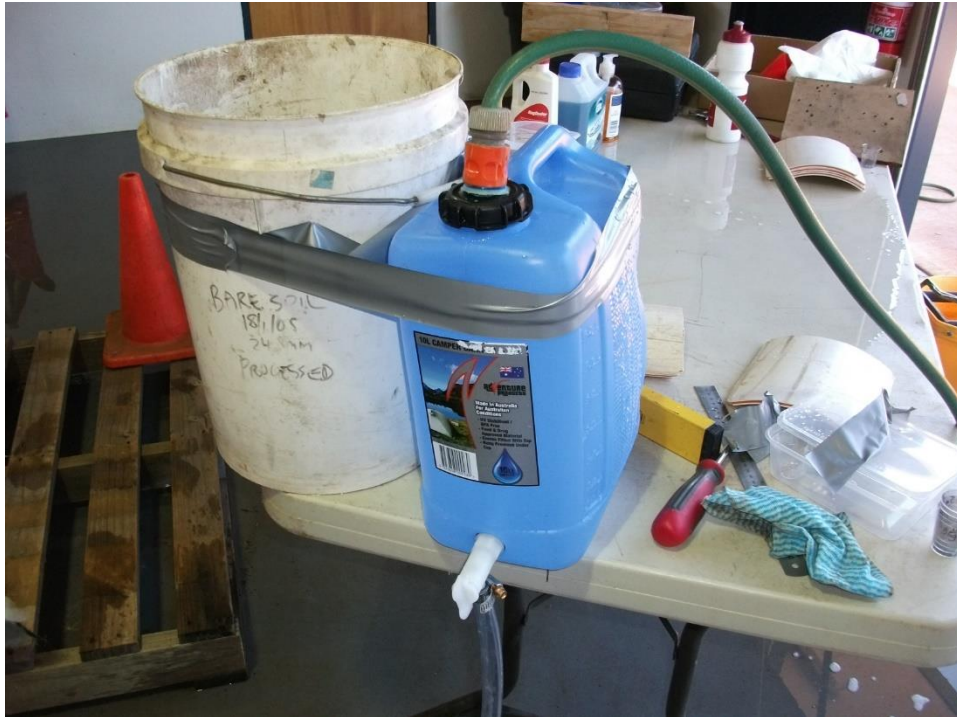
Figure 3.7.4- Chemical mix drum with town water supply coming in at the top and nozzle supply nose at the bottom.
