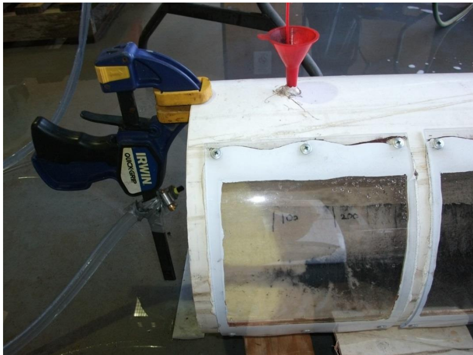
Figure 3.7.3- Photo of the spray nozzle at the entrance of the wind tunnel and the coal dust funnel.
