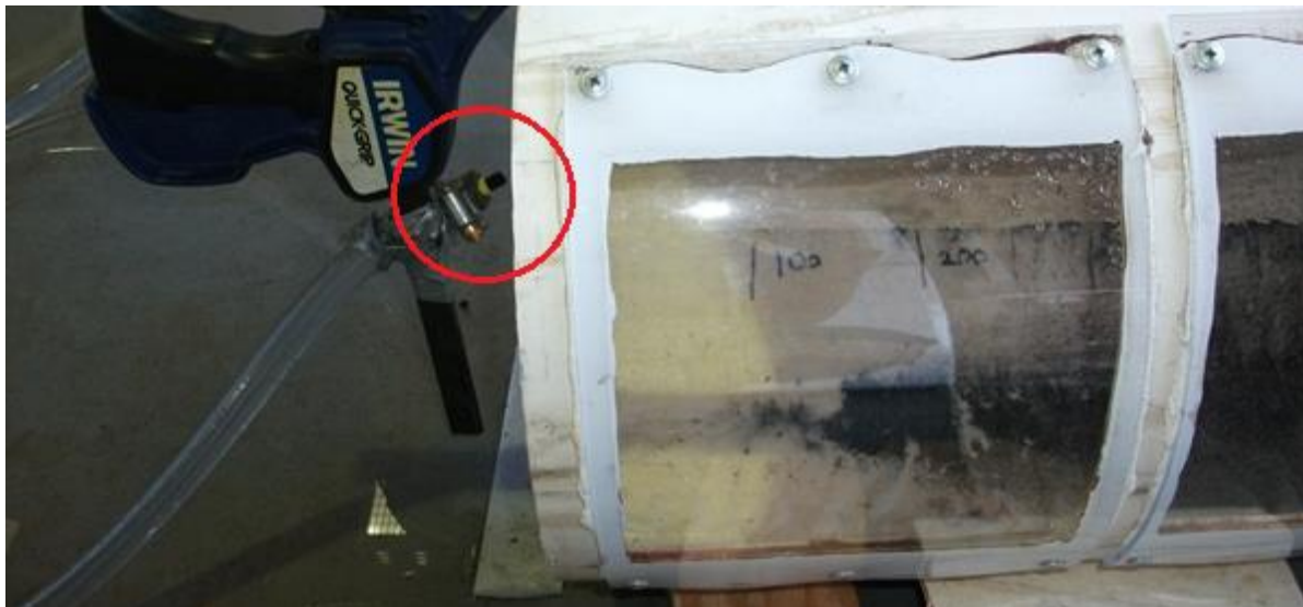
Figure 5.4.2 – The garden style spray nozzle that was used made it hard to get enough pressure.
