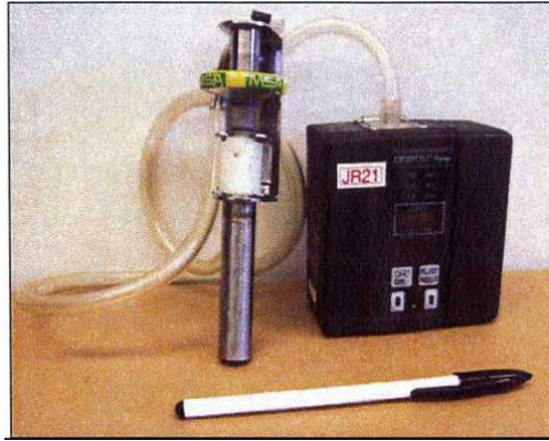
Figure 2.3- Gravimetric sampling pump, cyclone and filter assembly.
