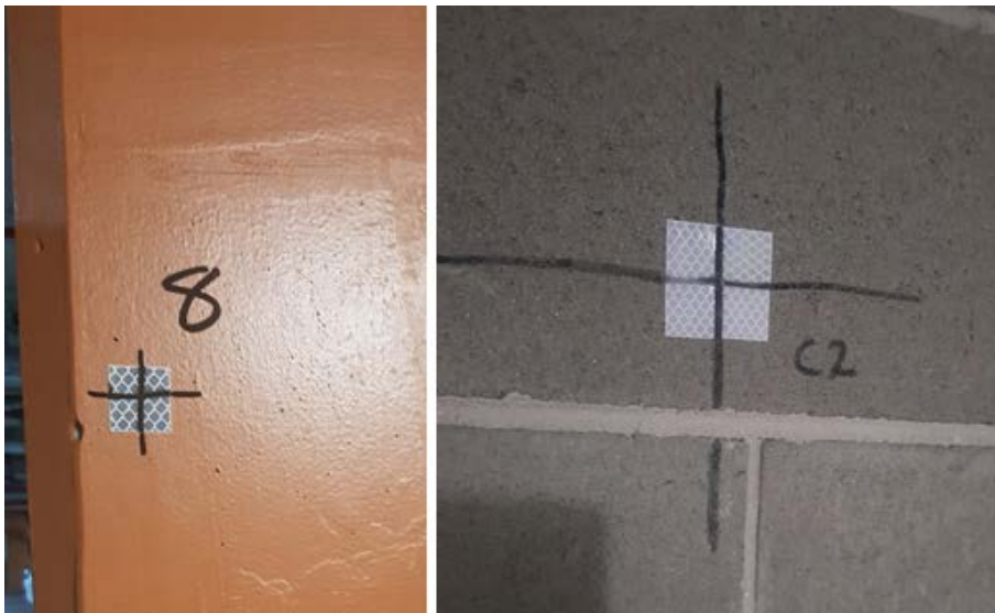
Figure 3.4.5 – Comparison of Normal sized and large control target
