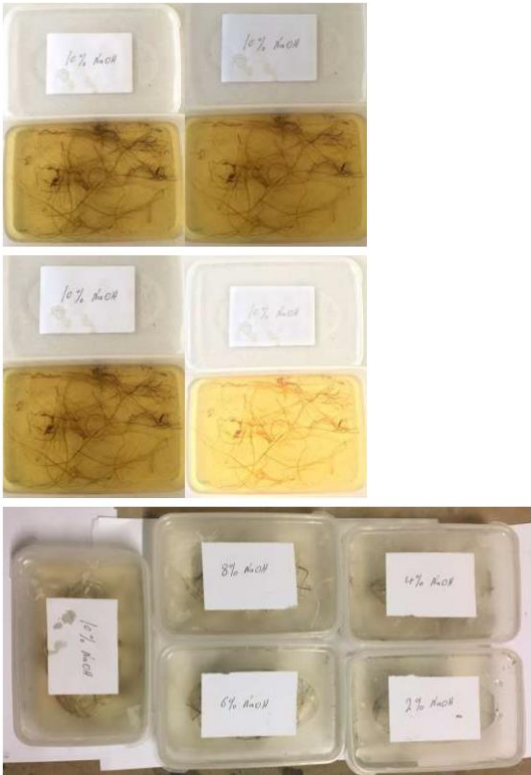
Figure 3. 2 NaOH treatment of the fibre at different concentrations.
