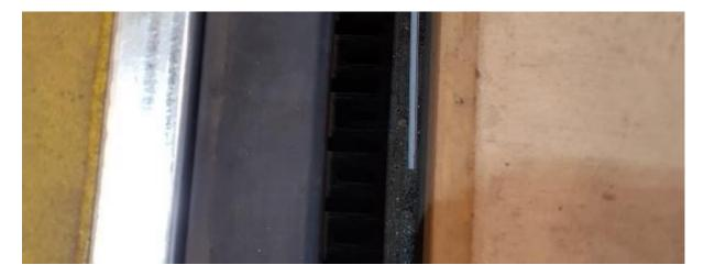
Figure 4.24. Gap between platform and light rail vehicle.
