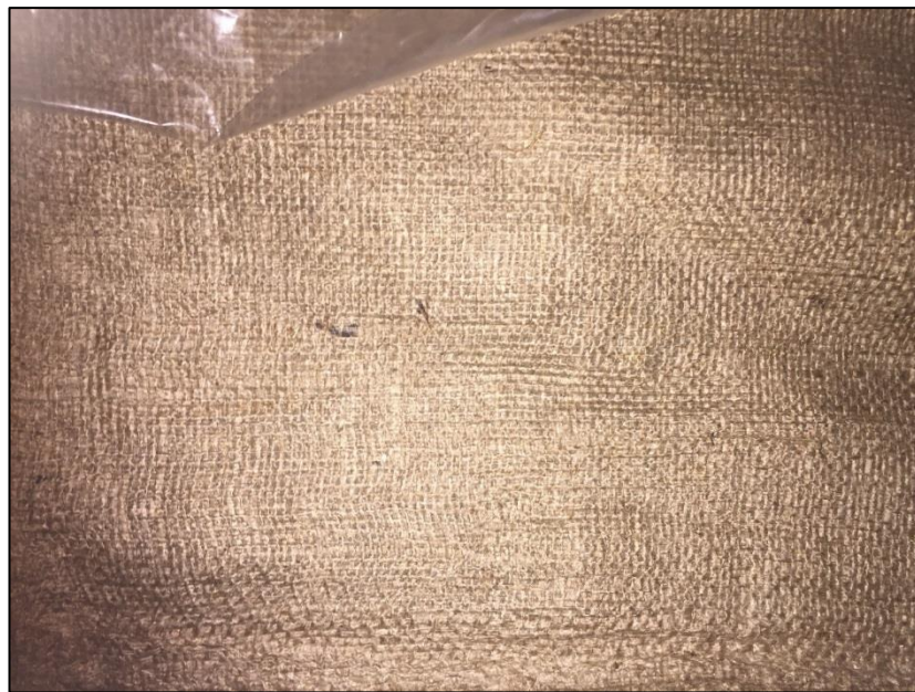
Fig. 3. 2 jute fibre mats purchased from Bunning warehouse.
