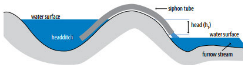
Figure 2.4. Siphon Operating with Free Outflow (D.Wigginton, 2013)
