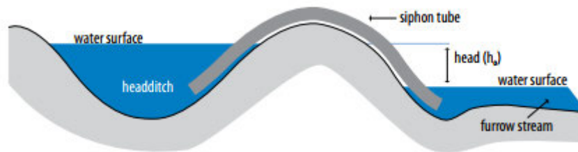
Figure 2.3. Siphon Operating with Submerged Flow (D.Wigginton, 2013)
