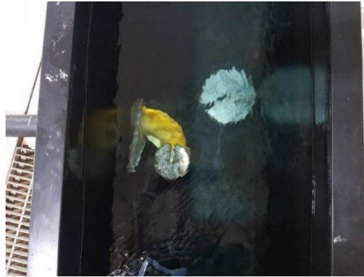
Figure 4.2. Weight Plate added to top of Inlet Pipe
