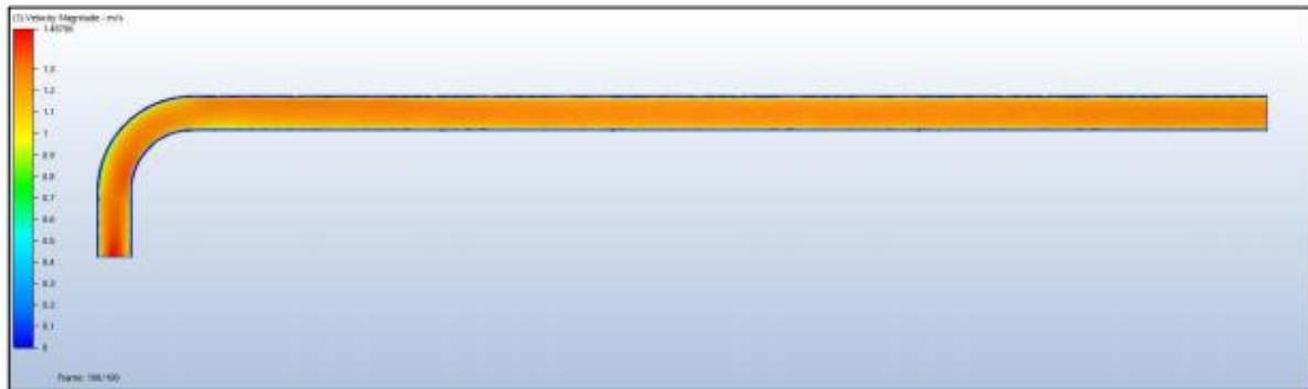
Figure 3.5. 90mm Smart Siphon CFD Flow Profile (Green, 2016)
