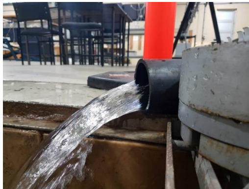
Figure 4.3. Pipe flow not at 'Full Pipe' flow
