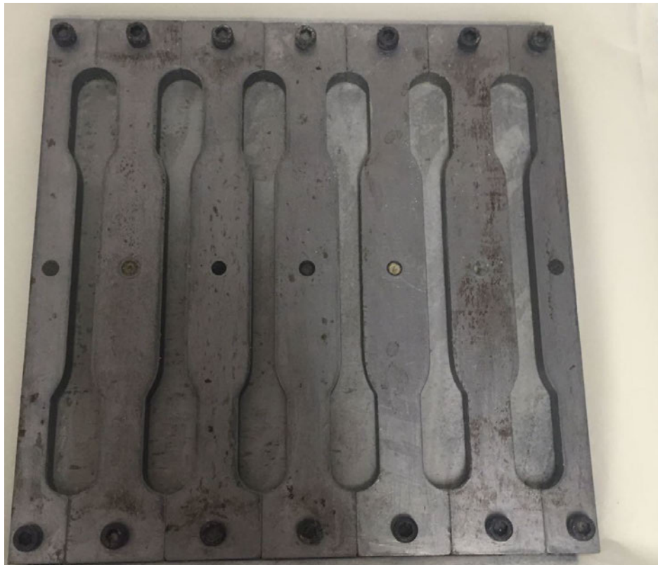
Figure 3. 5 mould used for the tensile samples
