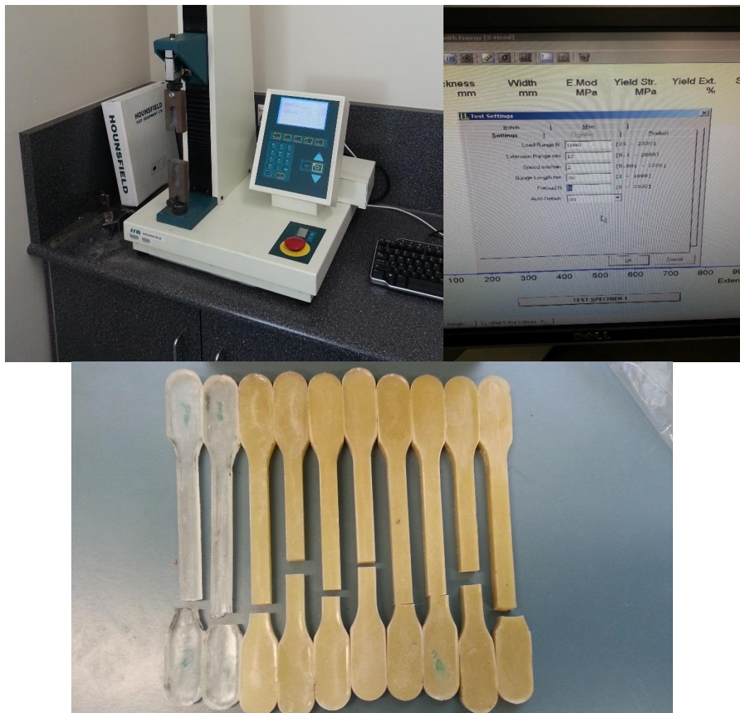
Figure 3. 9 universal tensile machine and eh software with the fractured samples after conducting the tests
