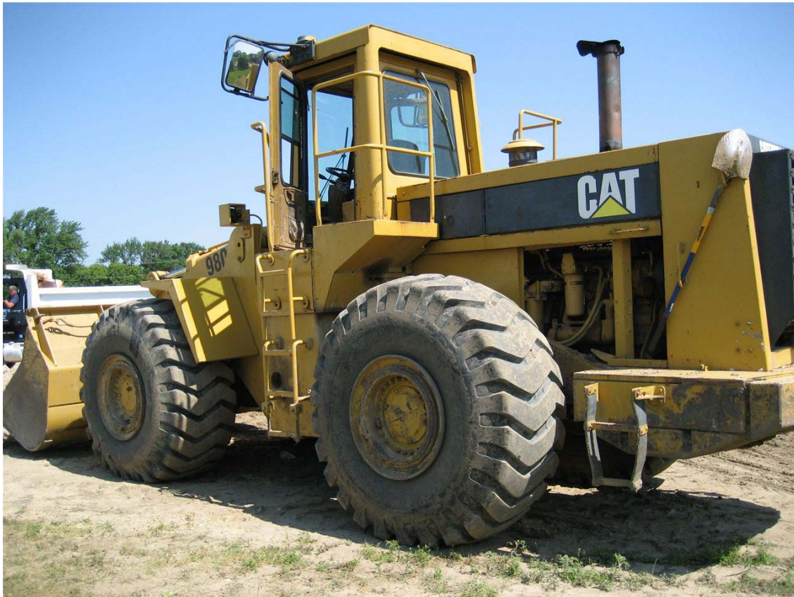
Figure 4.5: CAT 980C Front End Loader
