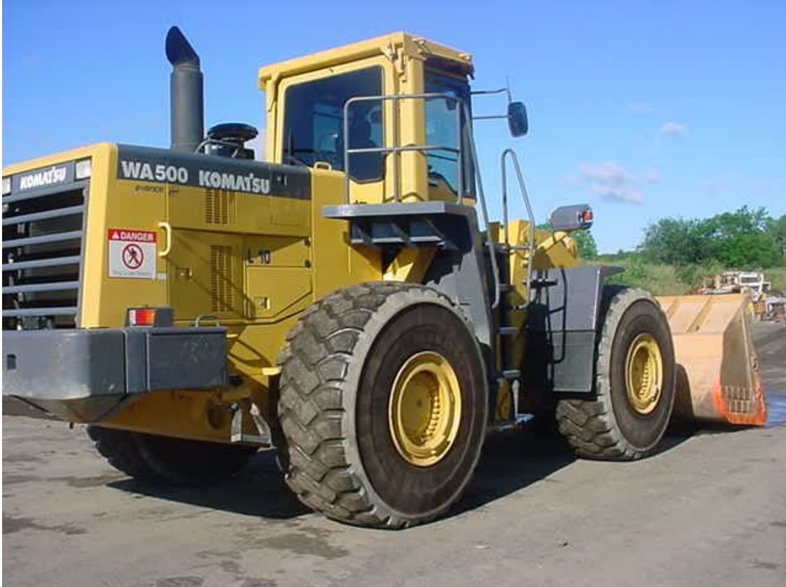
Figure 4.2: Komatsu WA500 Front End Loader (Machinery Trader, www.machinerytrader.com )
