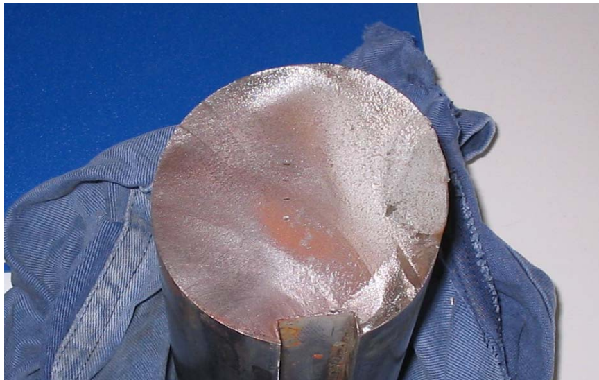
Figure 5.5: Cross Section view of broken shaft
