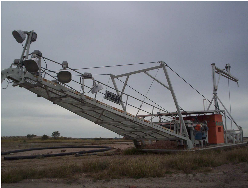
Figure 4.6 - Skid lighting System – Visit to Blair Athol Coal
