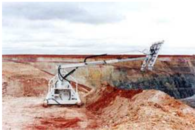
Figure 4.2 – Praying Mantis Lighting Plant – source: www.allight.com
