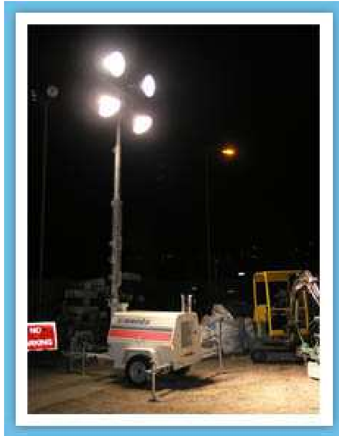
Figure 4.3 – Terex Amida Lighting System - Source: http://www.lighttowerspares.com
