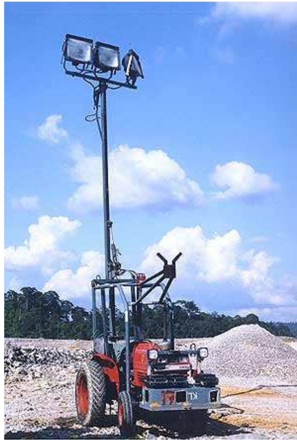
Figure 4.4 Kubota Lighting System - Source: http://www.minasco.com.au/Kubota-lighting-plant-2.jpg
