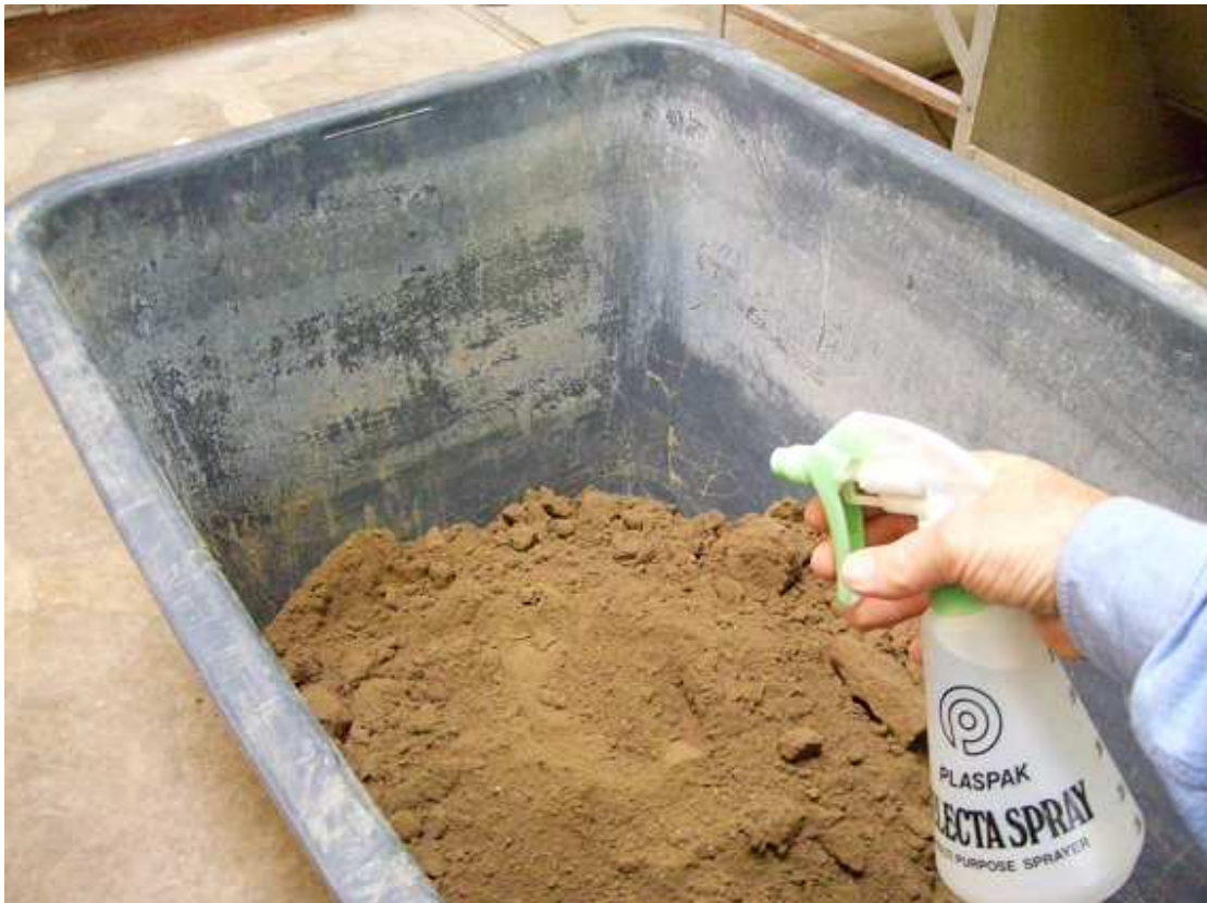
Figure 6.4 Application of Water to Soil Sample in 200litre Tub
