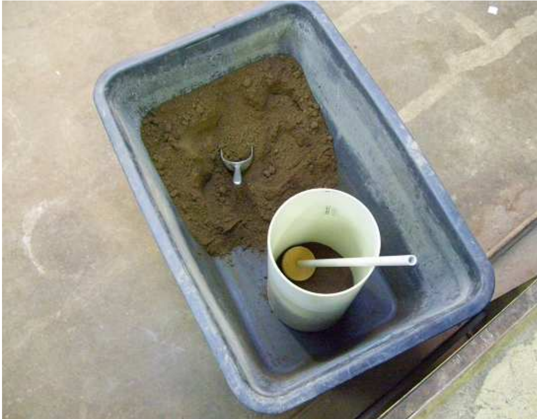
Figure 6.5 Compacting Soil Sample to Ensure Even Density
