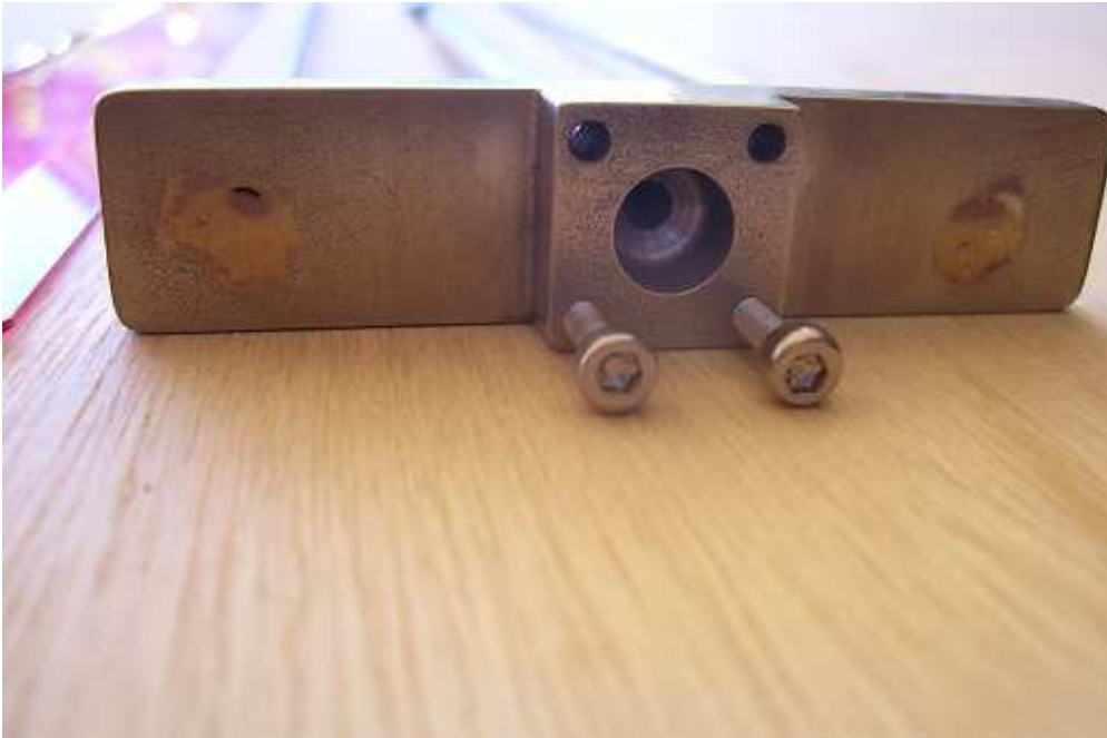
Figure D.3 Stainless Steel Arbour Showing Connection Details for Coaxial BNC Socket
