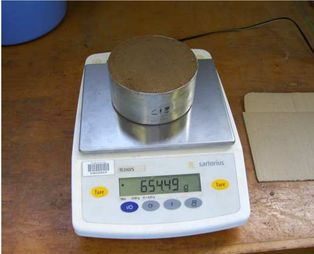
Figure 6.7 Accurate Weighing of Soil Sample After 24 Hours Drying
