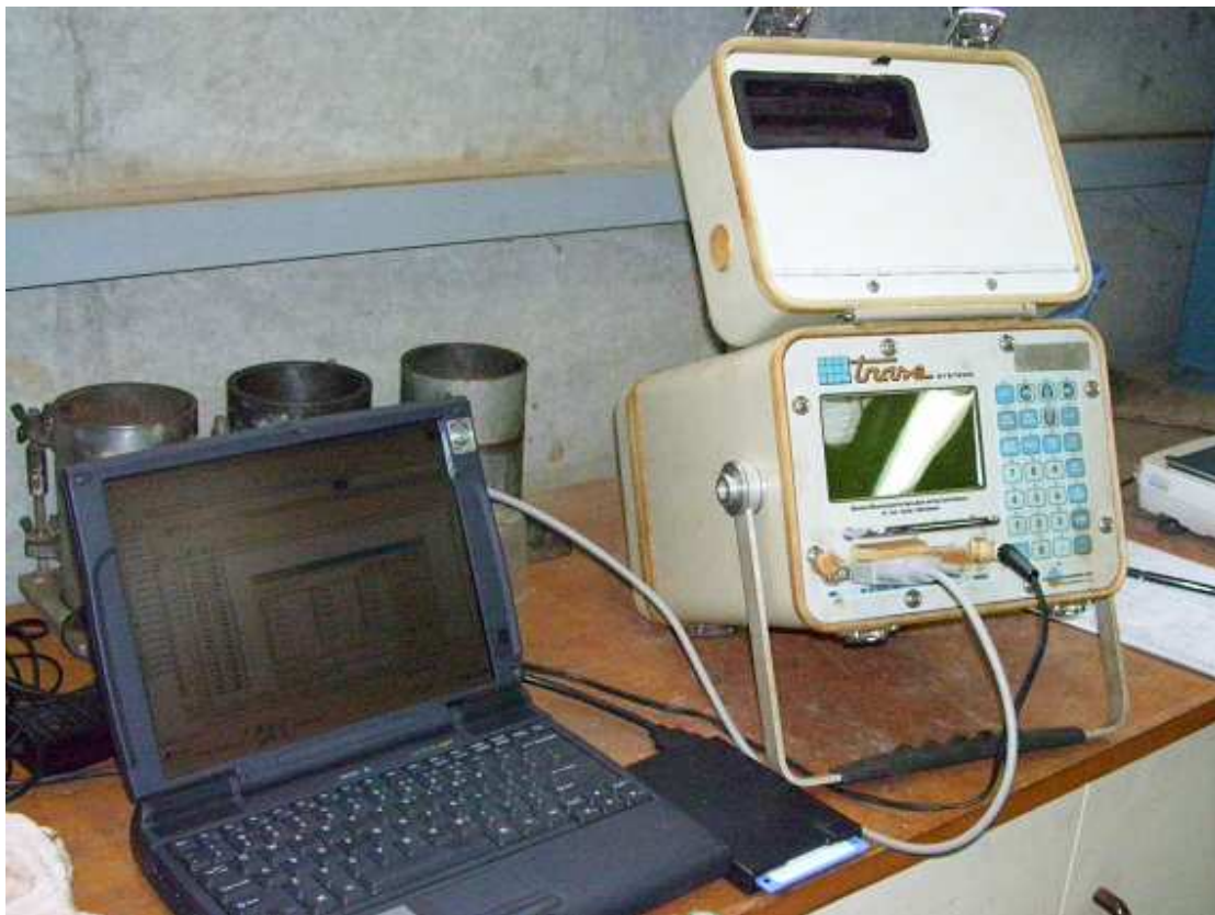
Figure 6.6 Downloading of TDR Waveforms to Laptop via RS232 Serial Port
