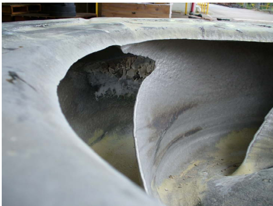
Figure 7.14: Loss in effective vane surface
