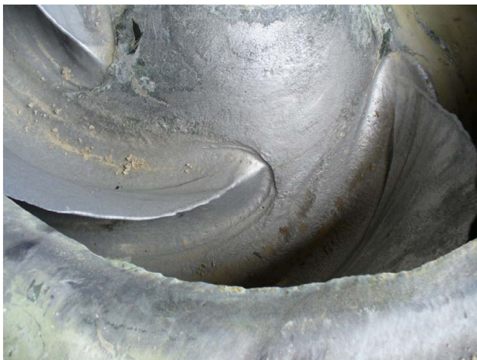
Figure 7.12: Metal loss on cutting edges, suction side
