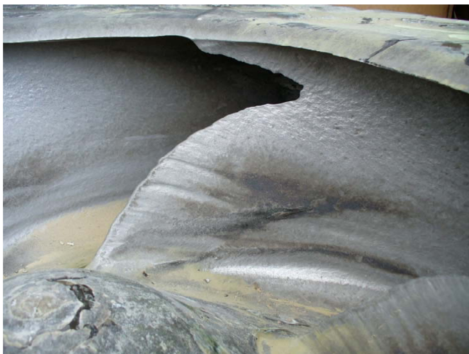
Figure 7.10: Eroded suction side impeller vane
