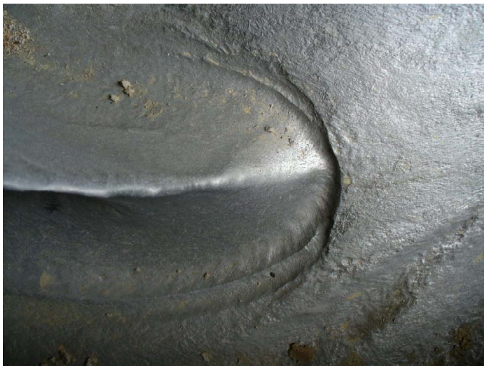
Figure 7.13: Close up of metal loss
