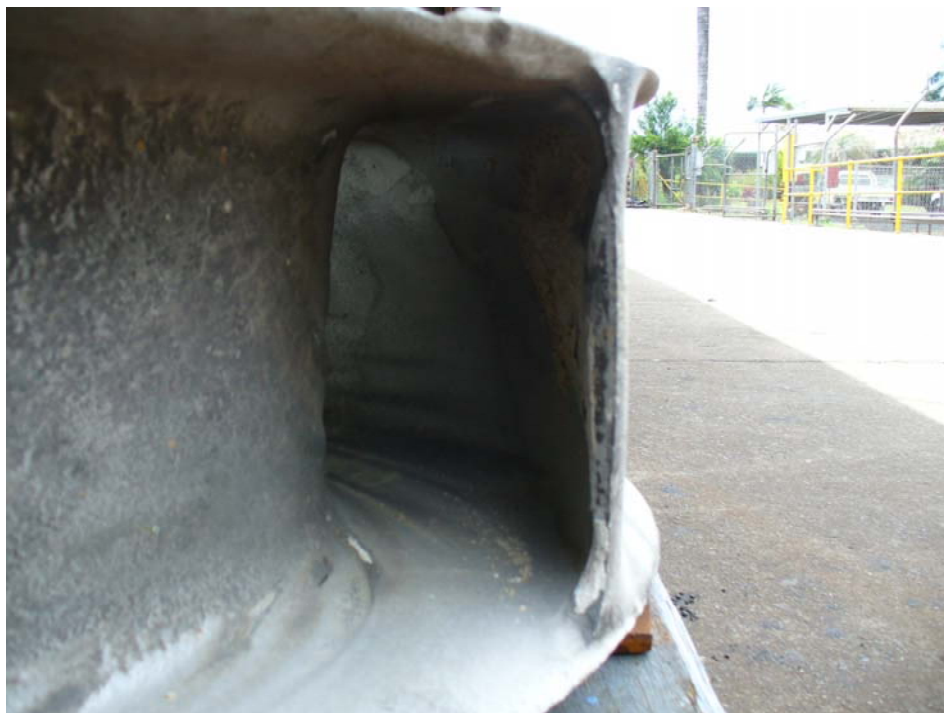
Figure 7.11: Erosion on exit of impeller vane, discharge
