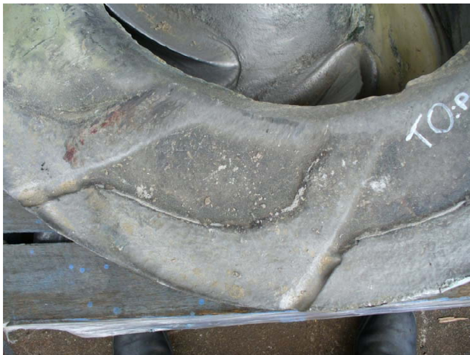
Figure 7.9: Wear on face and leading edges, suction side
