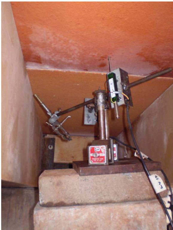
Figure 3-4: LVDT positioning for differential deck displacement
