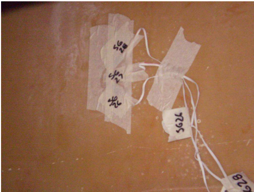
Figure 3-5: Delta rosette strain gauge configuration
