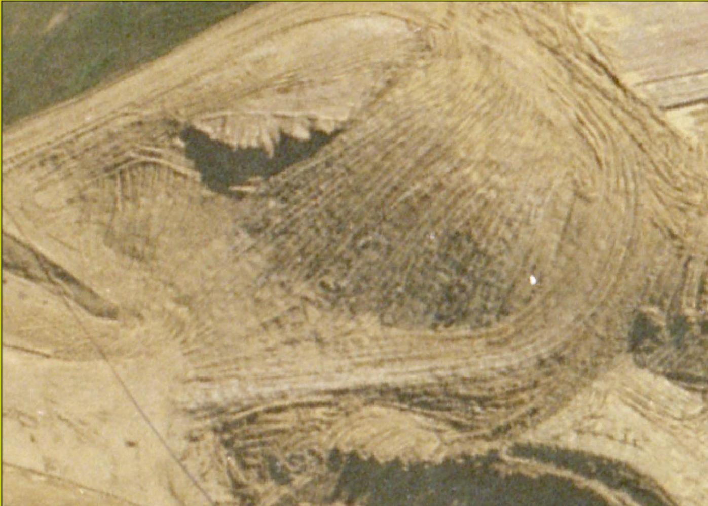
Overburden that covers the limestone is placed here by Scrapers to backfill past mining areas
