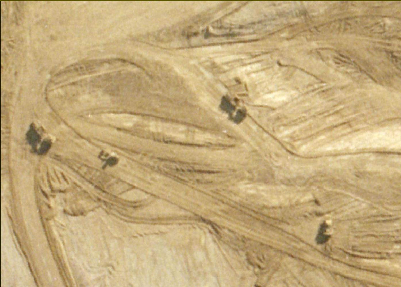
The limestone is mined by Bull Dozers and Scrapers on the exposed limestone bed
