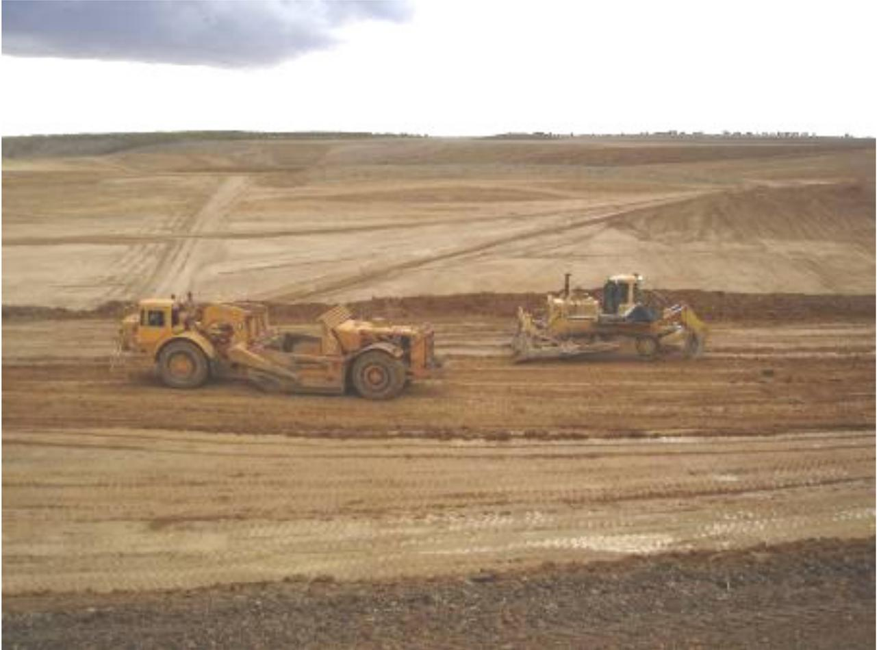
**Figure 8 : A Scraper and Bull Dozer travelling on overburden deposits**
