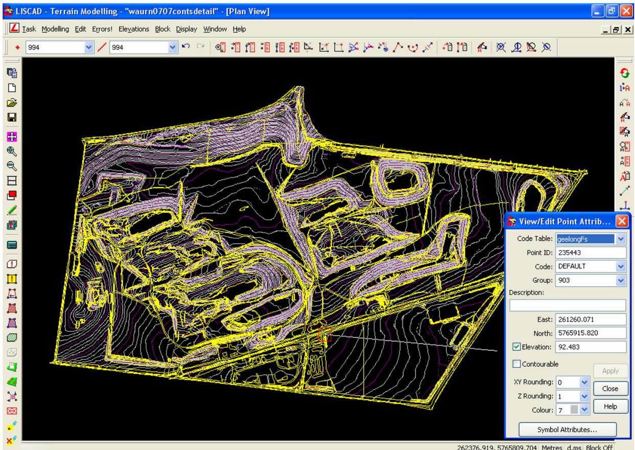
**Figure 12 : Level data in Aerial Photo in LISCAD**
