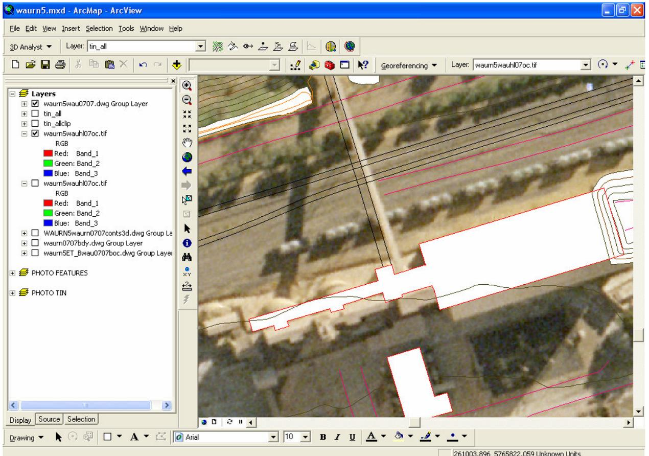
**Figure 21 : Georeferenced image overlaid with feature line work in ArcView**
