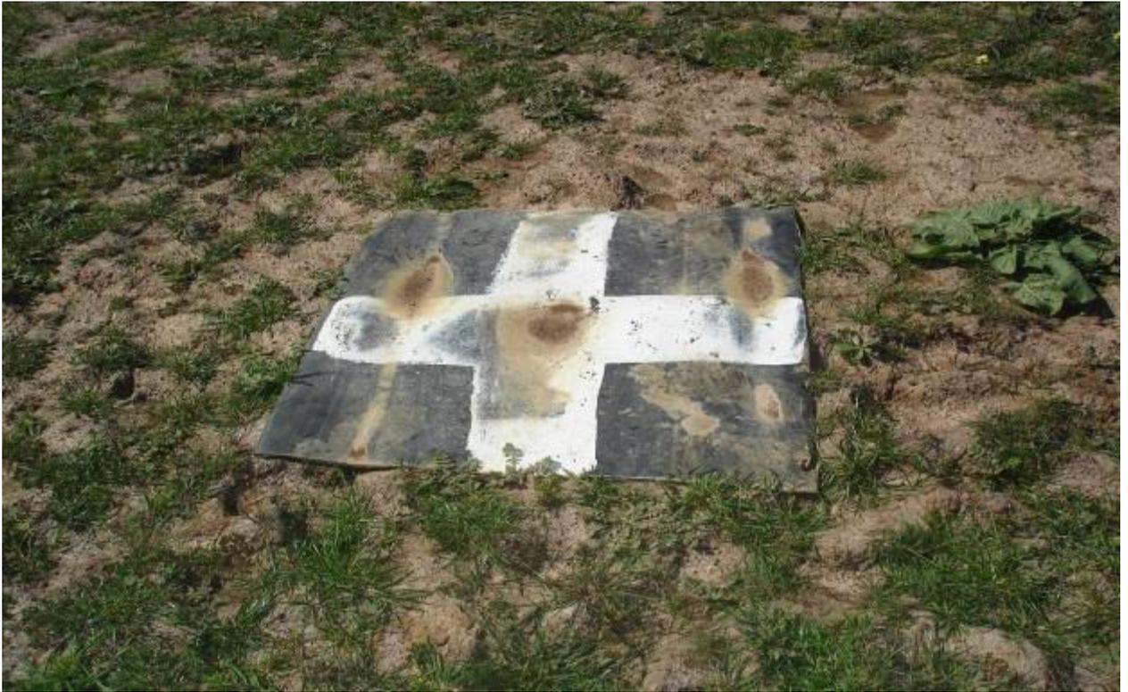
**Figure 10 : Image showing one of the Ground Control Points, placed on site before the aerial photography was flown**
