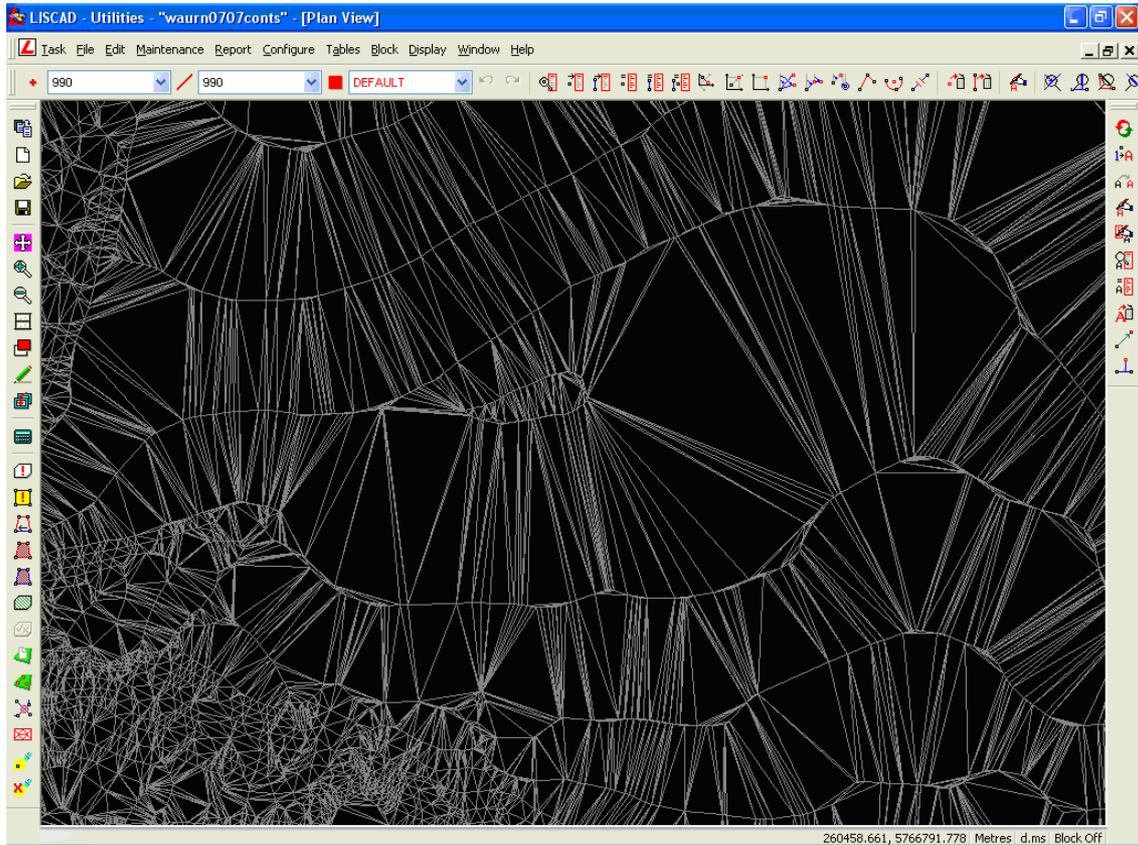
**Figure 2 : Example of a TIN from LISCAD’s Terrain Modelling package**
