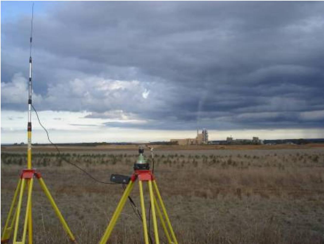
**Figure 9 : GPS base station unit logging data looking south, across rehabilitation areas the quarry to the factory**
