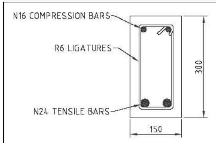
**Figure 3.3:** Cross Section of the Design Specimen
