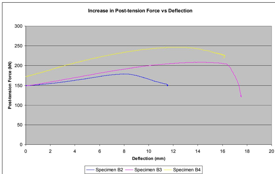
**Figure 5.12:** Increase in Post-tension Force as the Beams are Loaded
