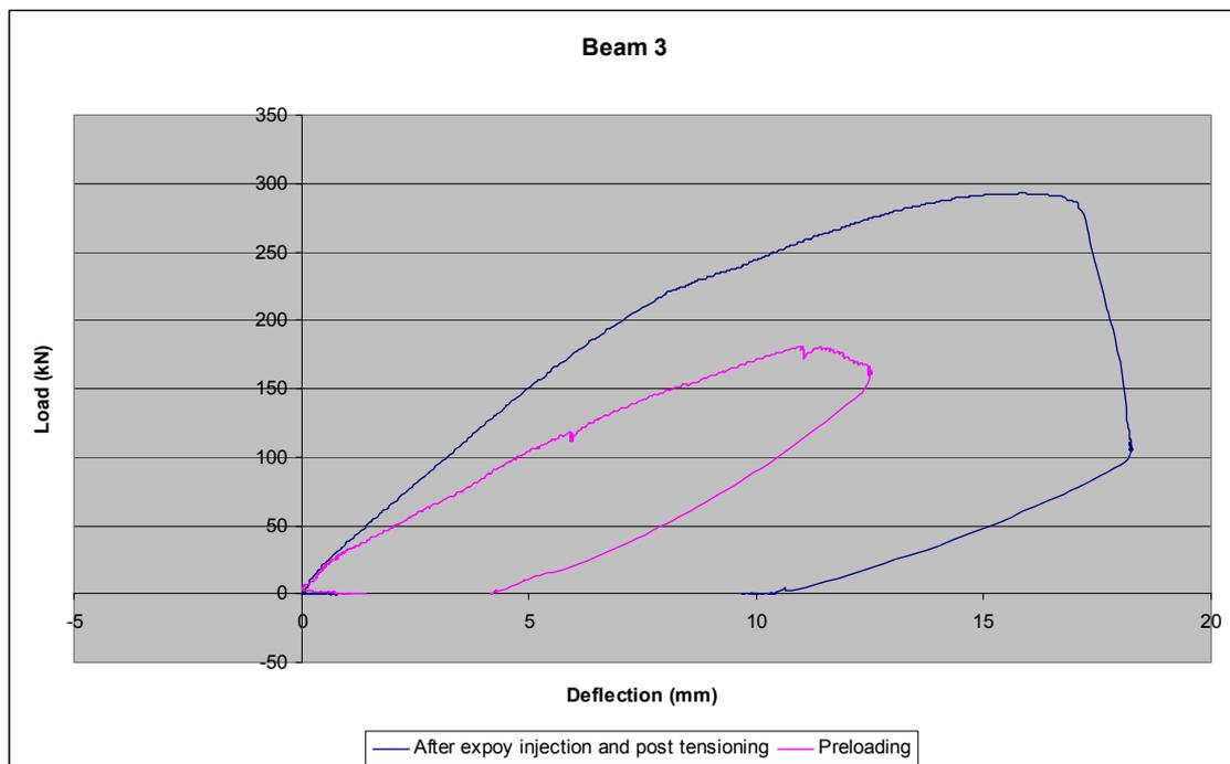
**Figure 5.10** Load-deflection plot of Specimen B3
