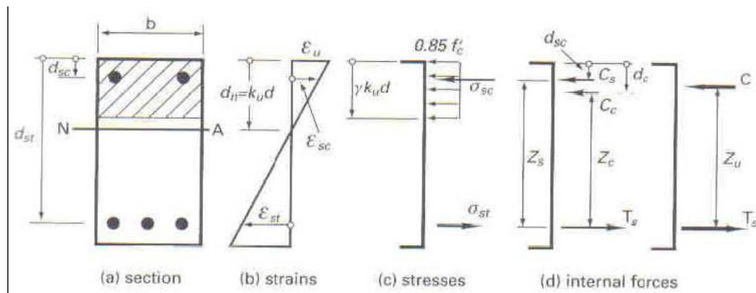
**Figure 3.3:** Doubly Reinforced Section at Ultimate Moment
