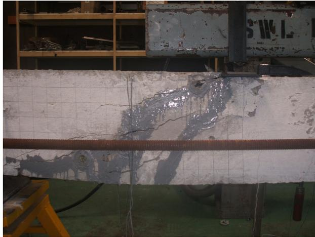
**Figure 5.6** Crack pattern in specimen B3.
