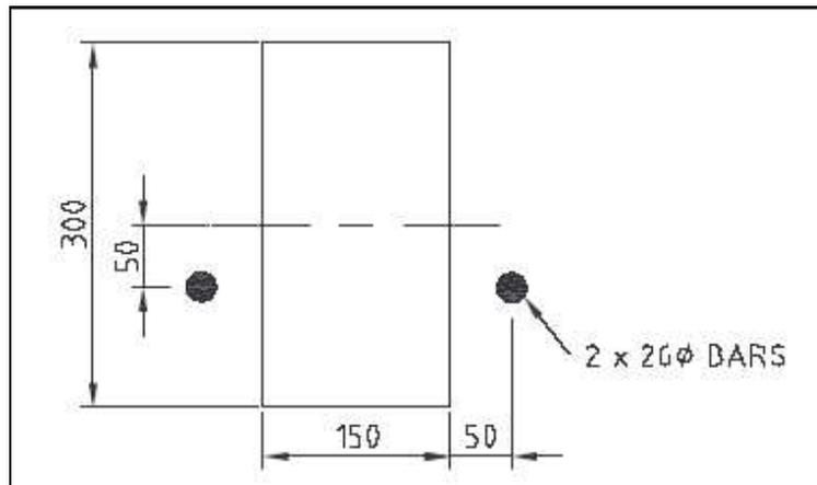
**Figure 3.4:** Positioning of Post-tensioning Bars
