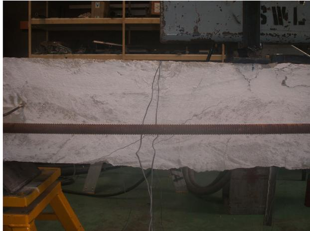
**Figure 5.7** Crack pattern in specimen B4.
