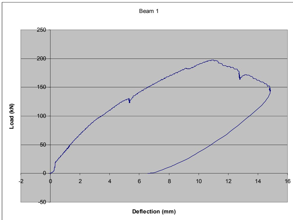
**Figure 5.8** Load-deflection plot of Specimen B1
