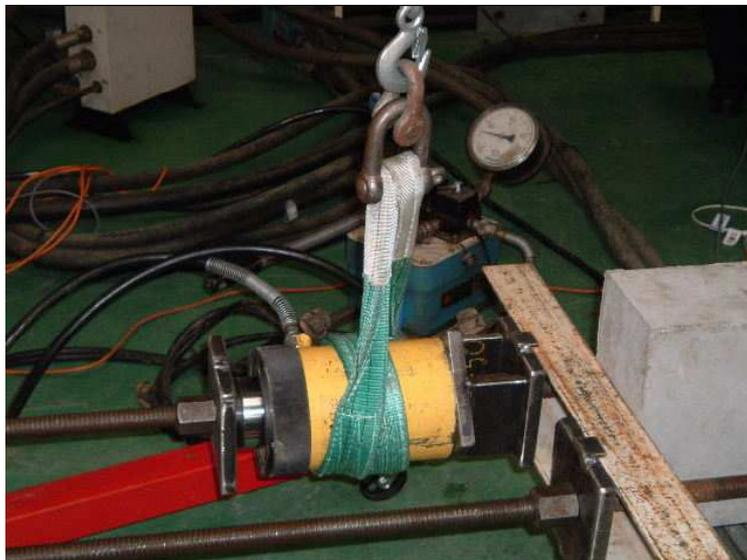
**Figure 4.3:** Stressing of Rods
