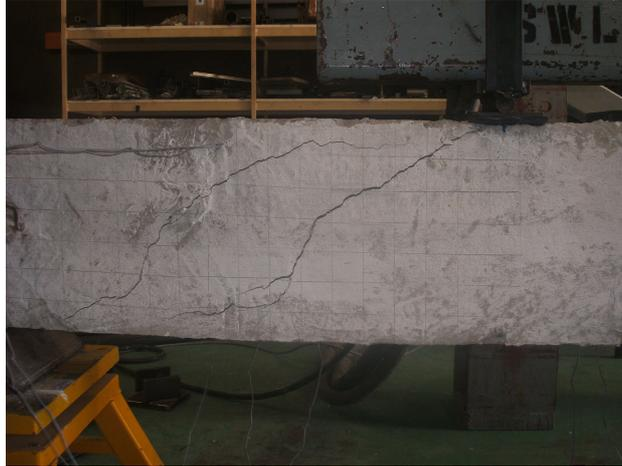
**Figure 5.3** Initial shear crack pattern in B2
