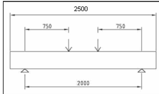
**Figure 3.1:** Specimen Size and Loading Position
