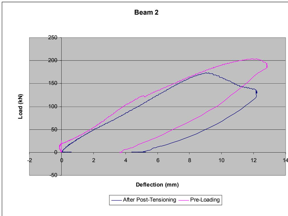
**Figure 5.9** Load-deflection plot of Specimen B2
