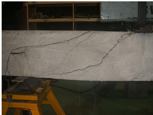
**Figure 5.1** Crack pattern for B1
