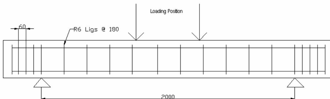
**Figure 3.5:** Specimen Design
