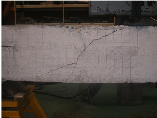
**Figure 5.5.** Initial crack pattern in specimen B3
