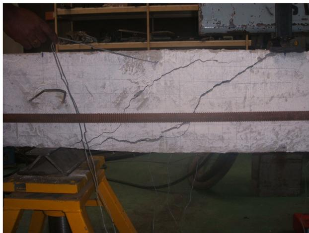
**Figure 5.4** Crack pattern in specimen B2
