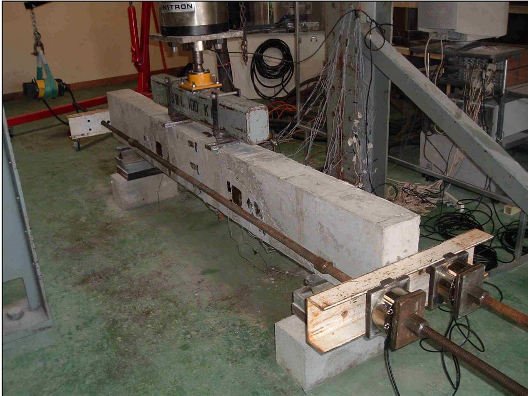
**Figure 4.4:** Test Configuration
