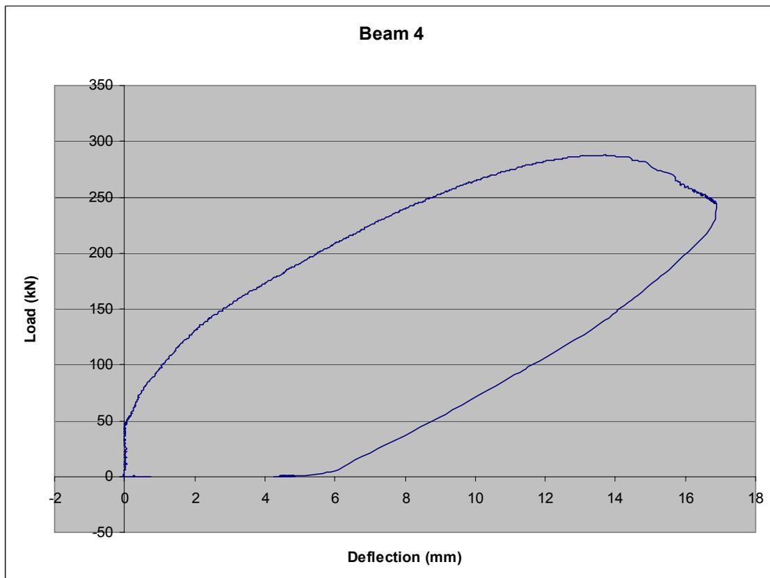
Figure 5.11 Load-deflection plot of Specimen B4
