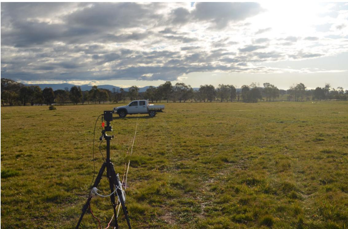
Figure 8.3: Experiment evaluating the maximum detectable range of a utility using mid-range chirp parameters.
