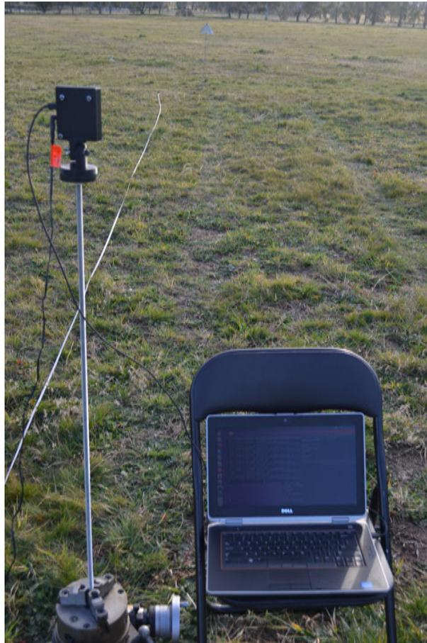
Figure 3.8: Beam width calibration
