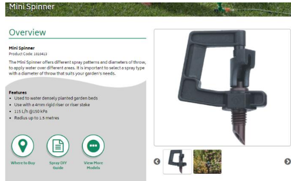
Figure 4-7 Typical mini sprinkler (from Hardy Pope)
