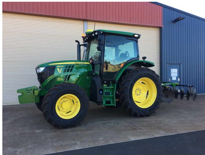
Figure 3.11: Deere 6120R used within tests, with a SF6000 Receiver mounted atop the cab
