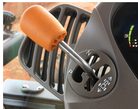
Figure 4.27: Gear selector (not engaged in any gear)
