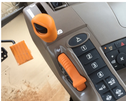
Figure 4.26: Speed and throttle controls (top left: speed control, bottom centre: throttle)
