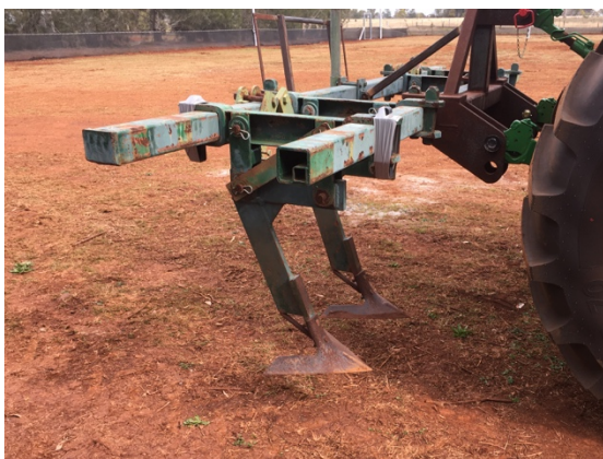
Figure 3.17A-B: Duck-foot ripper (noting two shanks removed) to provide unbalanced load
