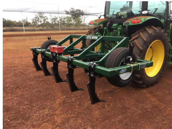
Figure 3.16A-B: Nine-shank chisel plough to provide a balanced load
