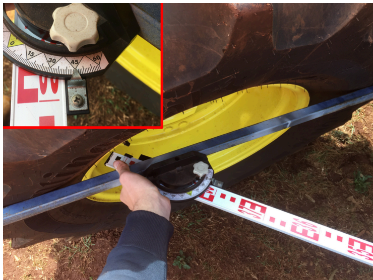
Figure 4.21: Straight edges being held against centre of each tyre
