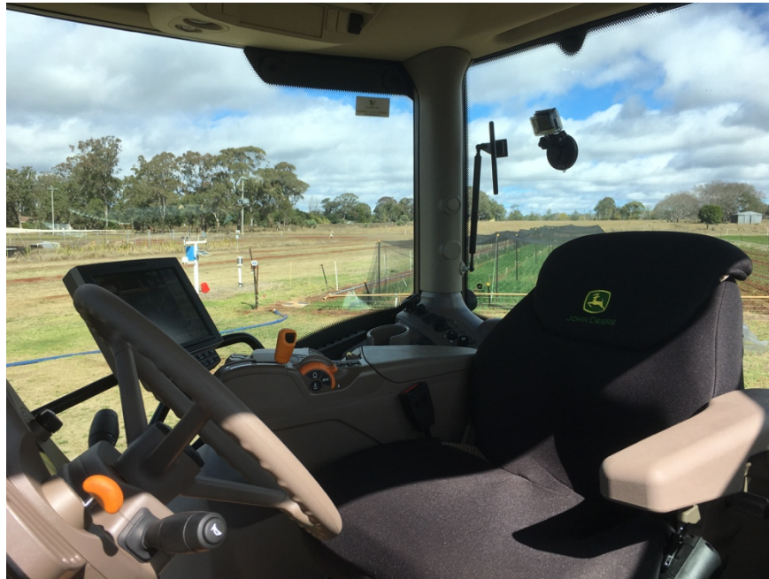
Figure 3.24: Cab of 6120R, with the GoPro mounted on the rear windscreen
