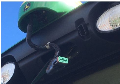
Figure 4.4: Disconnected SF6000 Receiver
