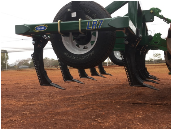
Figure 3.16A-B: Nine-shank chisel plough to provide a balanced load
