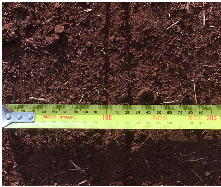
Figure 4.7: Measuring the error between passes to deduce accuracy
