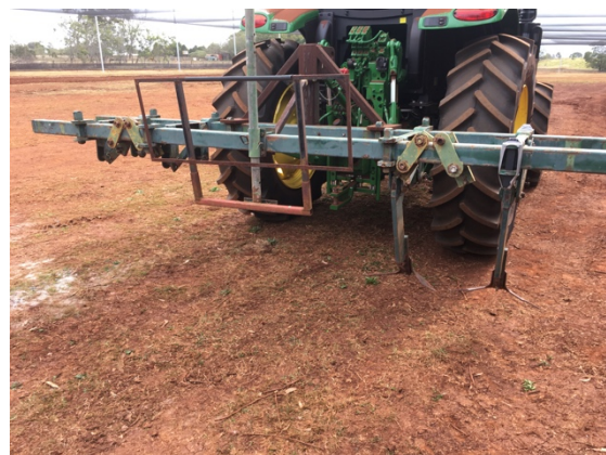
Figure 3.17A-B: Duck-foot ripper (noting two shanks removed) to provide unbalanced load
