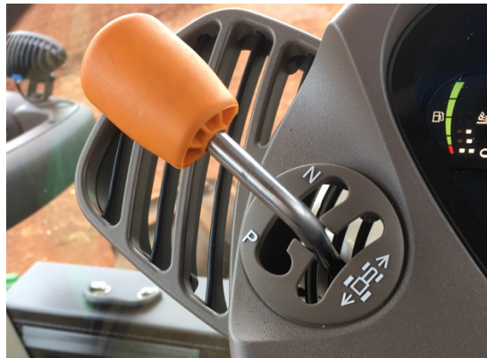
Figure 4.6: Gear selector (in the spring-loaded 'neutral' position)
