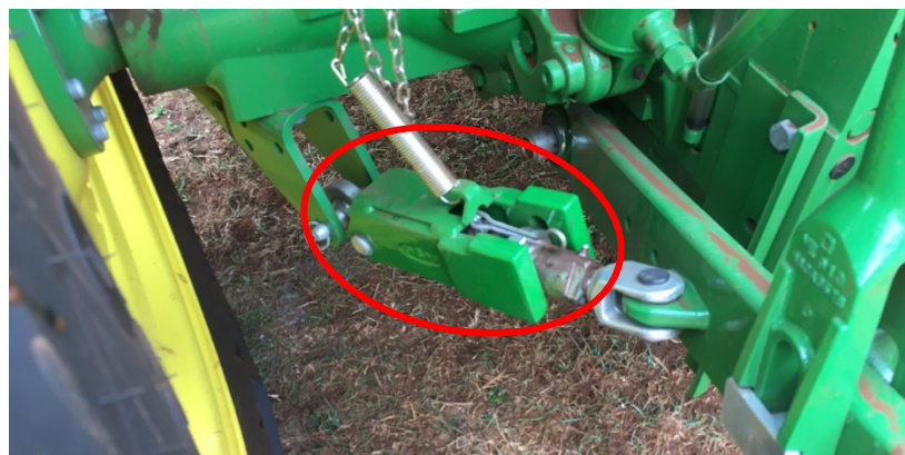
Figure 3.18: Sway-block (circled) engaged on rear hitch
