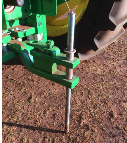
Figure 3.19: Installed row marking spike
