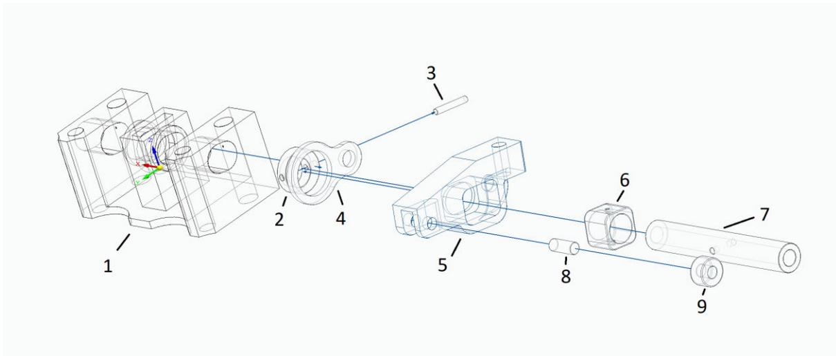
*Figure 3: exploded diagram of components for a single rocker*
