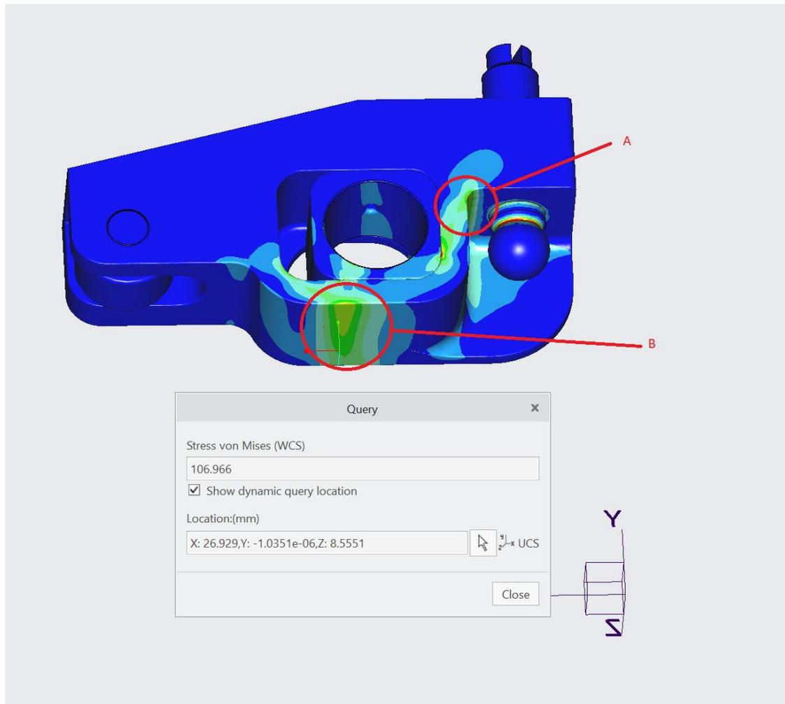
Figure 4.1: FEA results comparison for rocker
