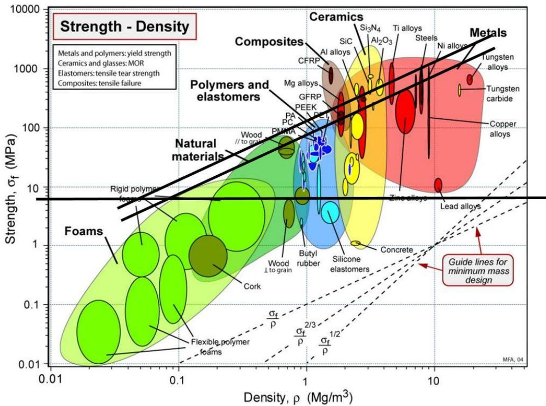
Figure 3.4 & 3.5: Strength vs. Relative cost and strength vs. Density (Canfield joints, material selection)
