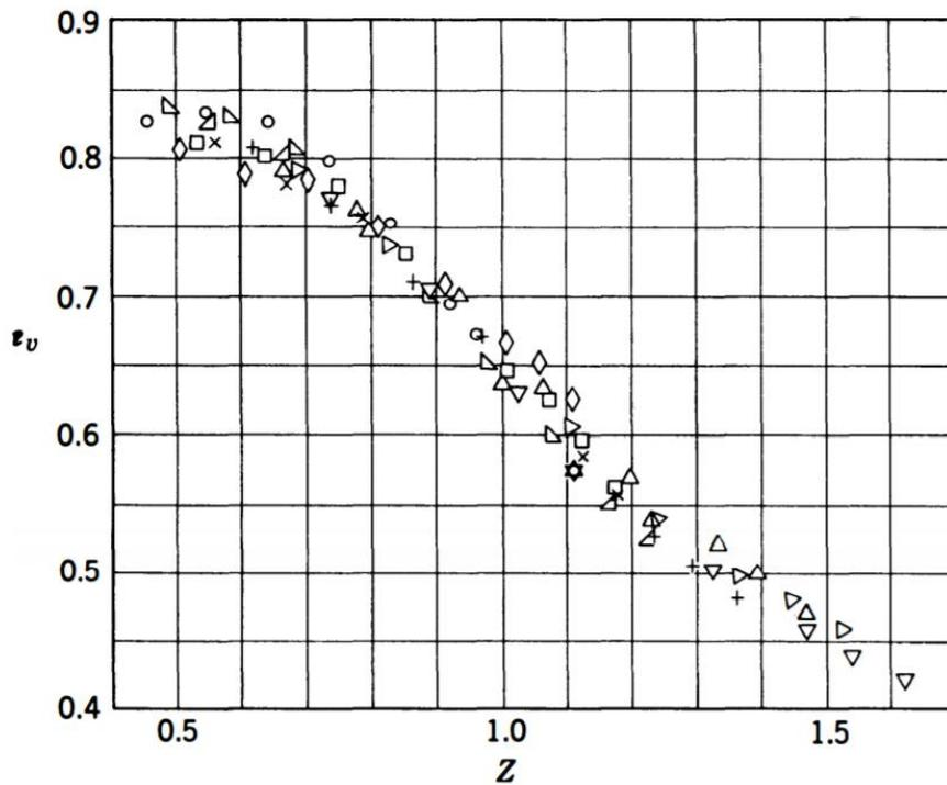
Volumetric efficiency vs inlet-valve Mach index.
