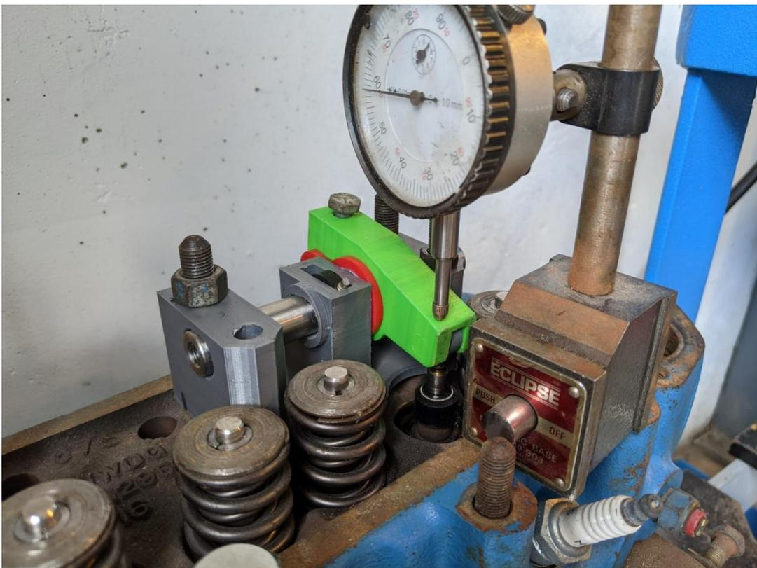
*Figure 4.15: Measuring maximum valve lift*
