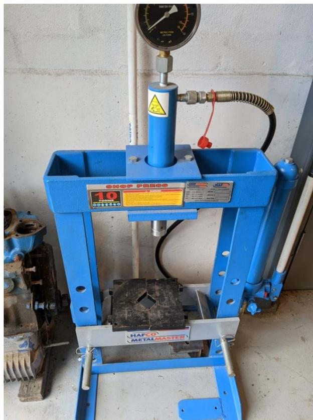
*Appendix A.2.2: Hydraulic press for removing valve springs*
