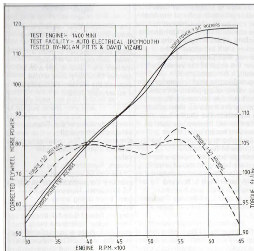
Figure 2: Difference of power and torque with rocker ratios 1.3 and 1.5, showing loss of low end torque with 1.5 ratio rockers over the smaller 1.3. (David Vizard)
