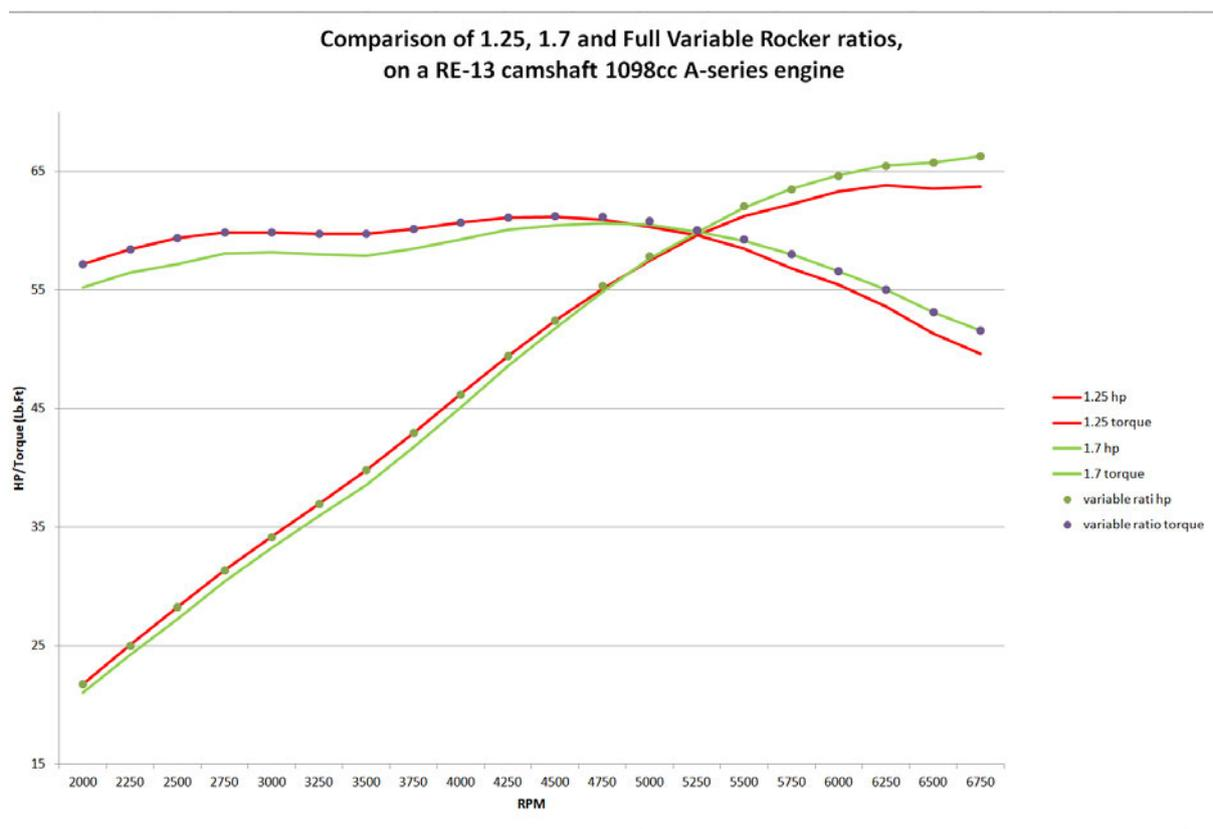
Figure 4.02: 1098cc standard cam engine simulations (engine analyser 3.9B)
