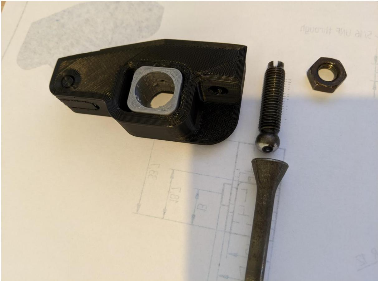
*Figure 4.13: Pushrod and pushrod adjuster bolt being the shape limiting factor*
