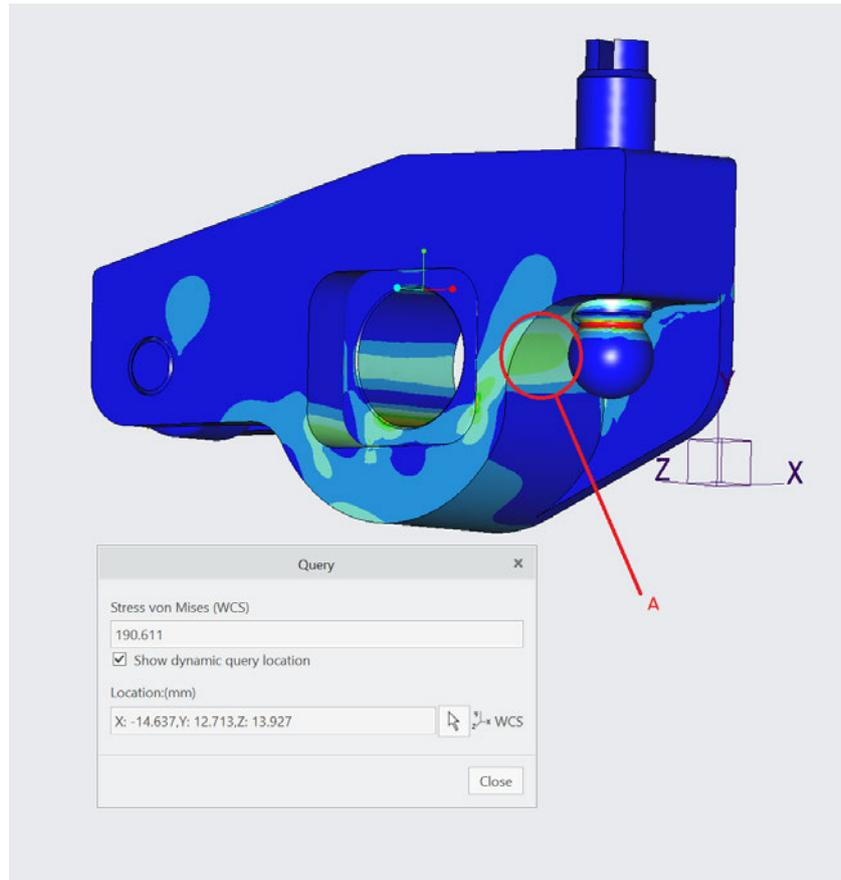
Figure 4.14: FEA results with further modifications (V3)
