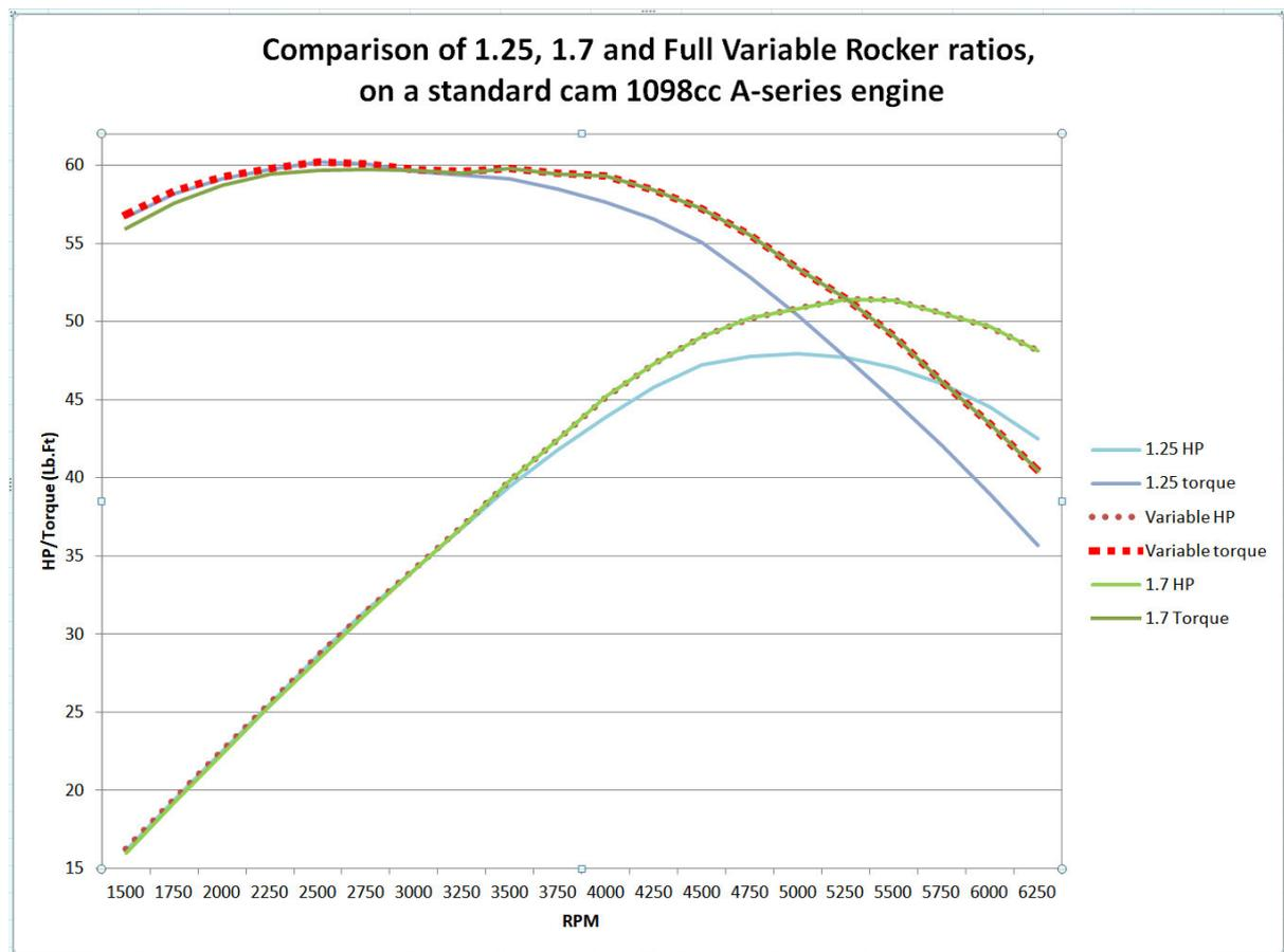
Figure 4.01: 1098cc standard cam engine simulations (engine analyser 3.9B)
