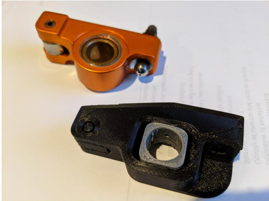
Figure 4.11: Comparison of Harland sharp rocker showing large radius in critical areas
