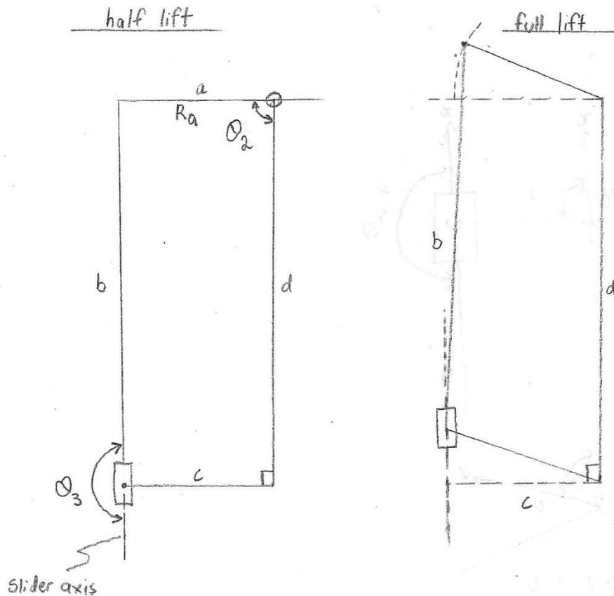
Figure 3.3: Valve lift movement kinematics
