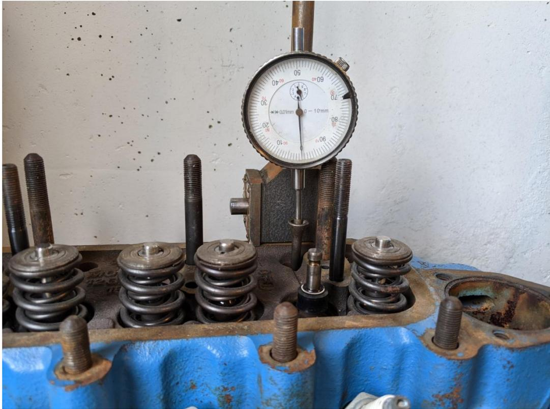
*Figure 4.14: Measuring maximum cam lift*
