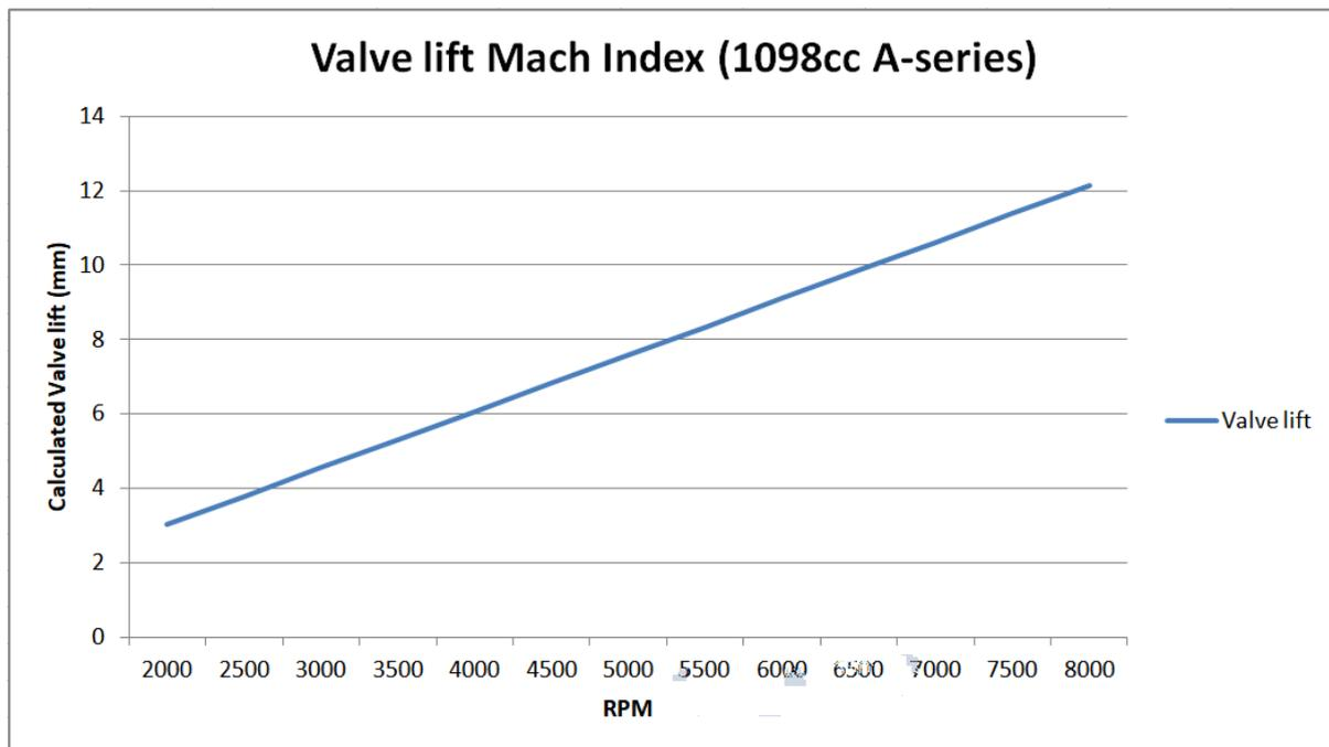
*Figure 4.04: Mach index ratio, calculated valve lift for 1098cc A-series*
