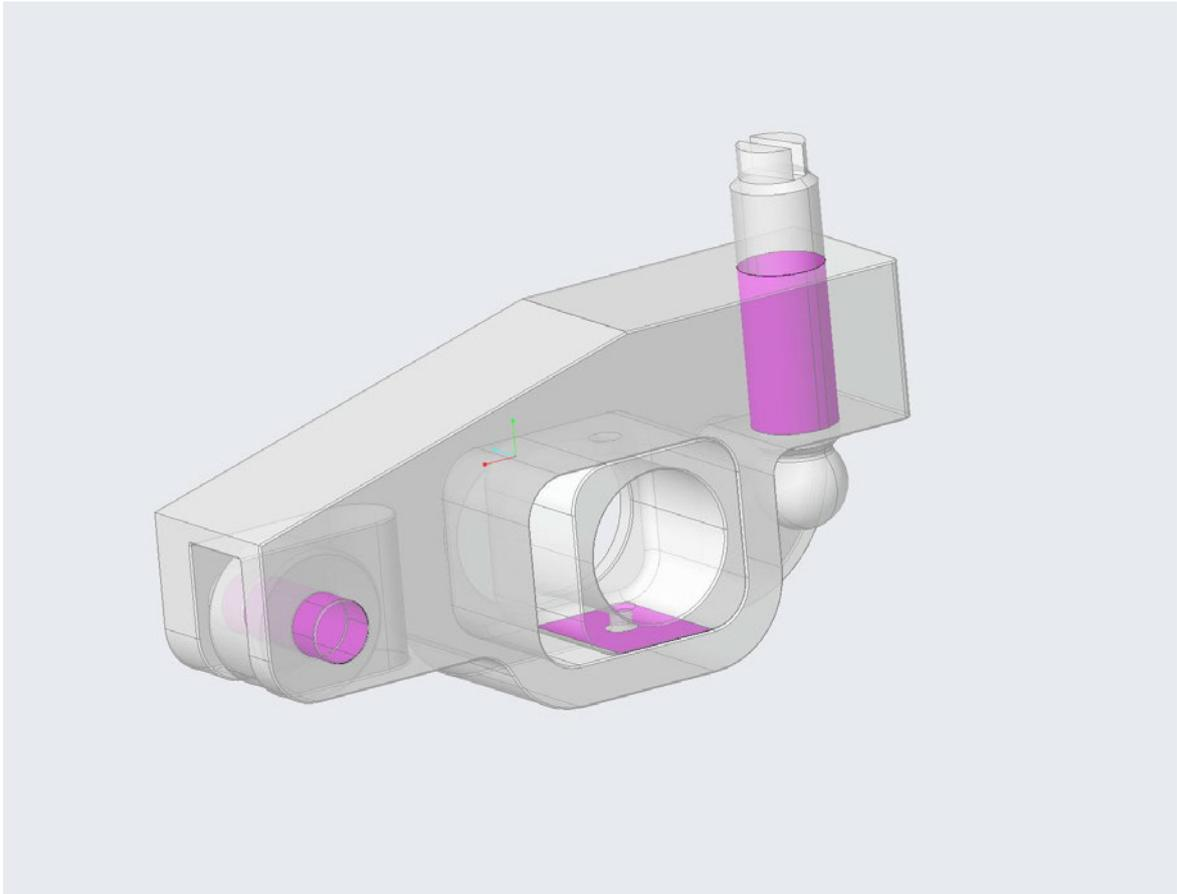
Figure 4.08: Creo Simulate rocker contact surfaces
