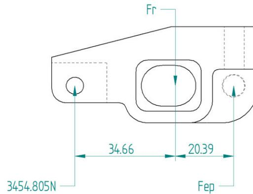
Figure 4.05: Rocker force diagram
