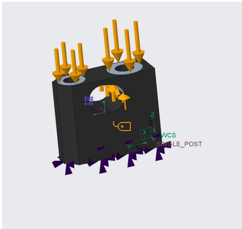
*Figure 4.11: Rocker loads and constraints*
