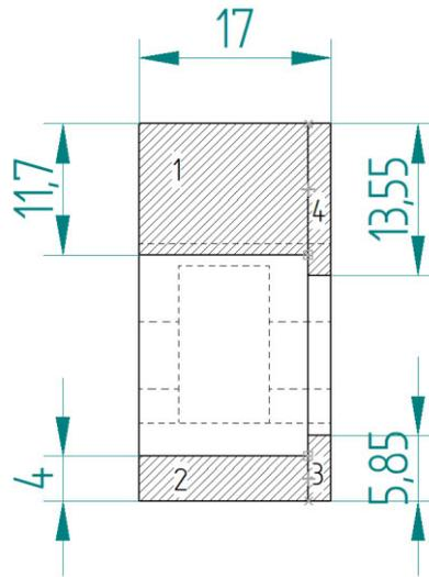
Figure 4.06: Section view of rocker for moment of inertia
