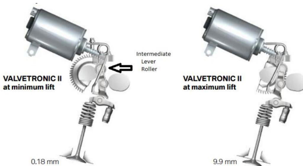
Figure 2.2: BMW Valvetronic valve lift (search auto parts 2017, how to repair BMW Valvetronic)
