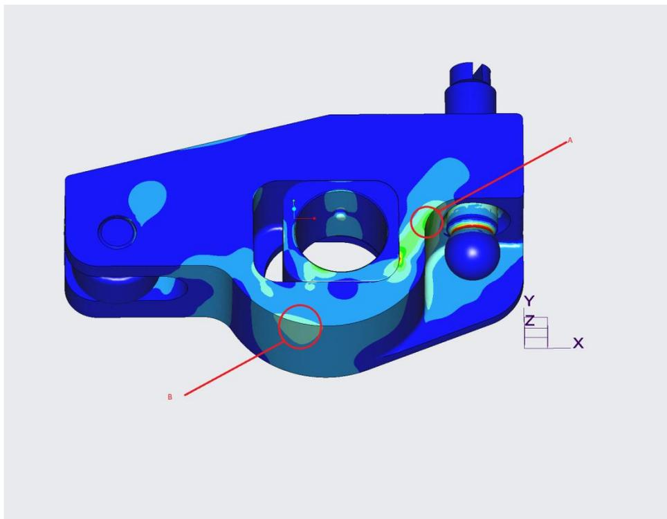
Figure 4.12: FEA results for modified design (V2)
