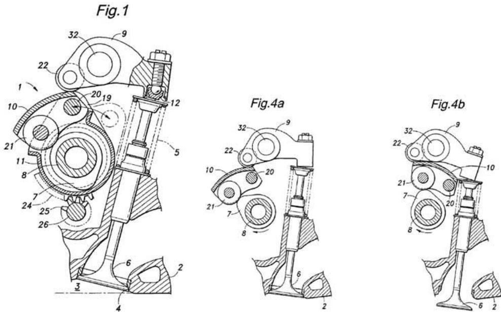
Figure 2.1: Cross sectional view of Honda's AVTEC continuously variable valve lift
