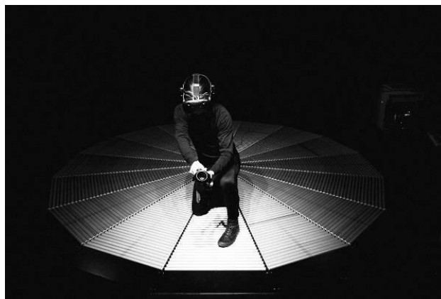
Figure 2.2: The Omnidock - a roller-driven design omnidirectional treadmill (Lodola, 2018).
