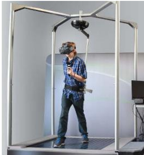
Figure 2.3: The Infinadeck omnidirectional treadmill with a belt-driven design walking platform (Lodola, 2018).
