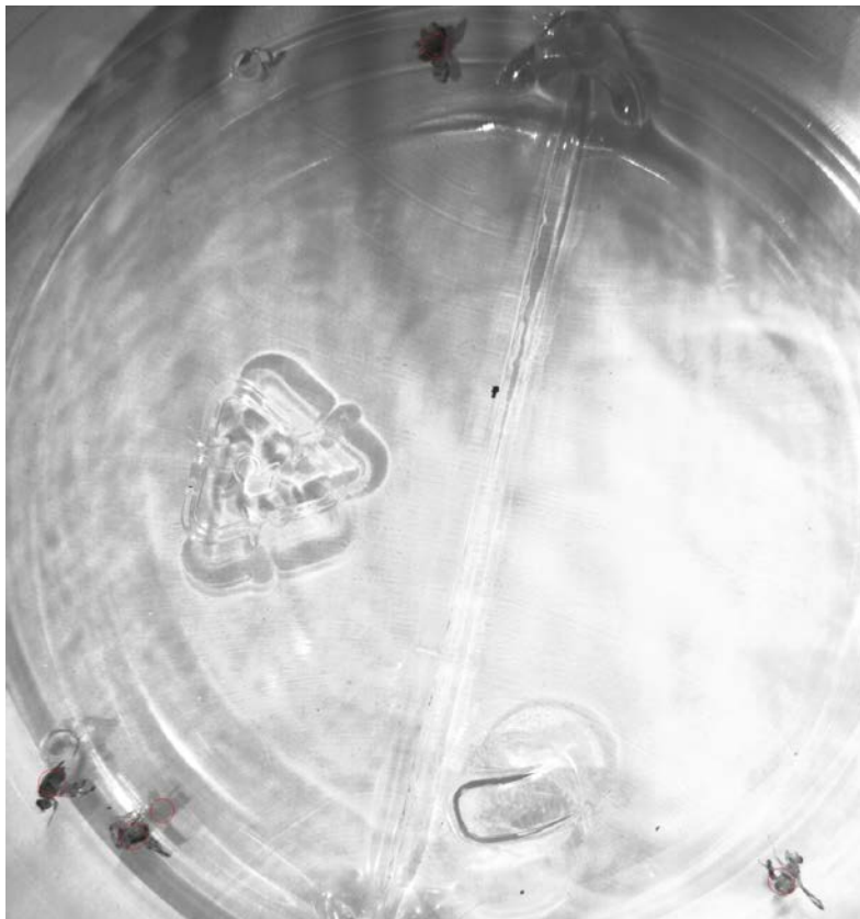
Figure 21 Blob detection results for the same image as Figure 11 (Note blobs marked as fine red circles).
