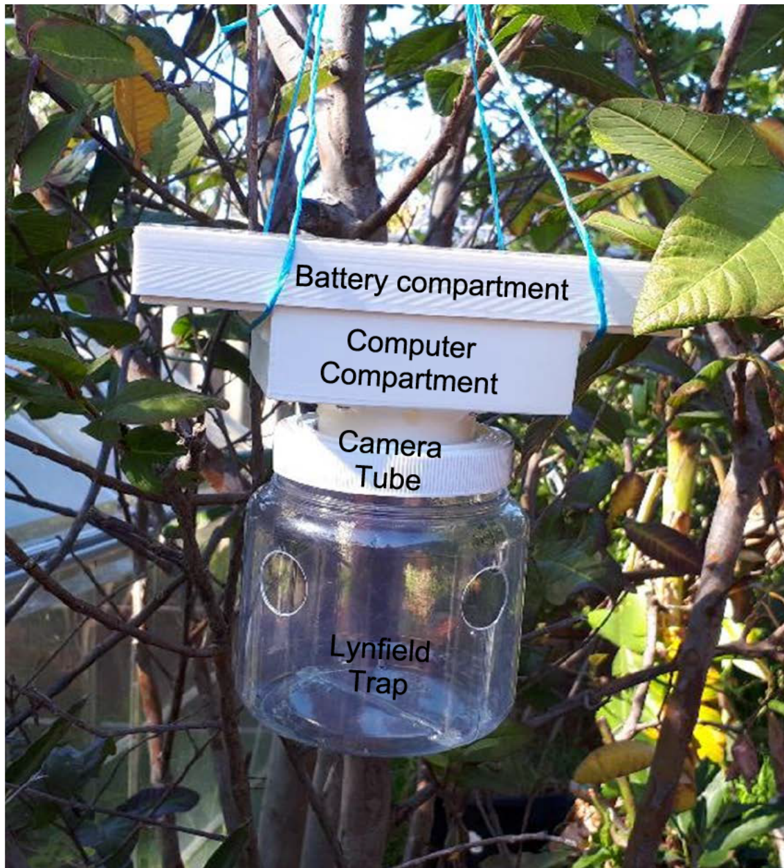
Figure 8 Photo of fully assembled trap
