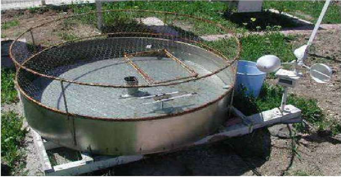
Figure 3 - Evaporation Pan (Source: Ertek 2011): Photograph of a Pan Evaporation Method Apparatus, note the climate measurement devices and the animal cage.
