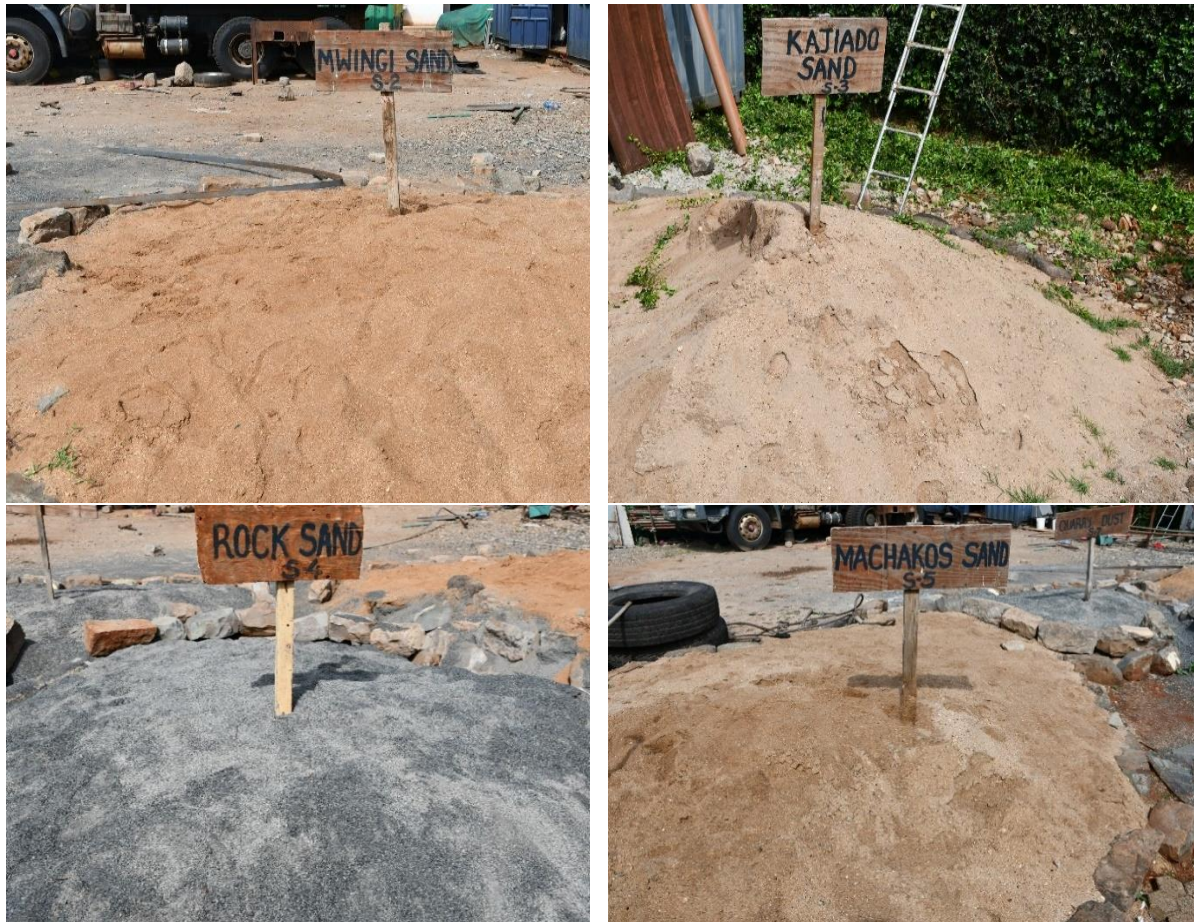
Figure 3.2 Some of the fine aggregates available in Nairobi.
