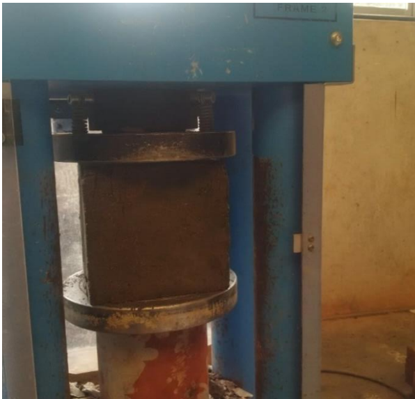
Figure 3-4 Compressive strength testing in the laboratory
