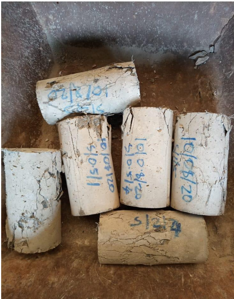
Figure 4.1 some of the tested specimens showing failure behaviour
