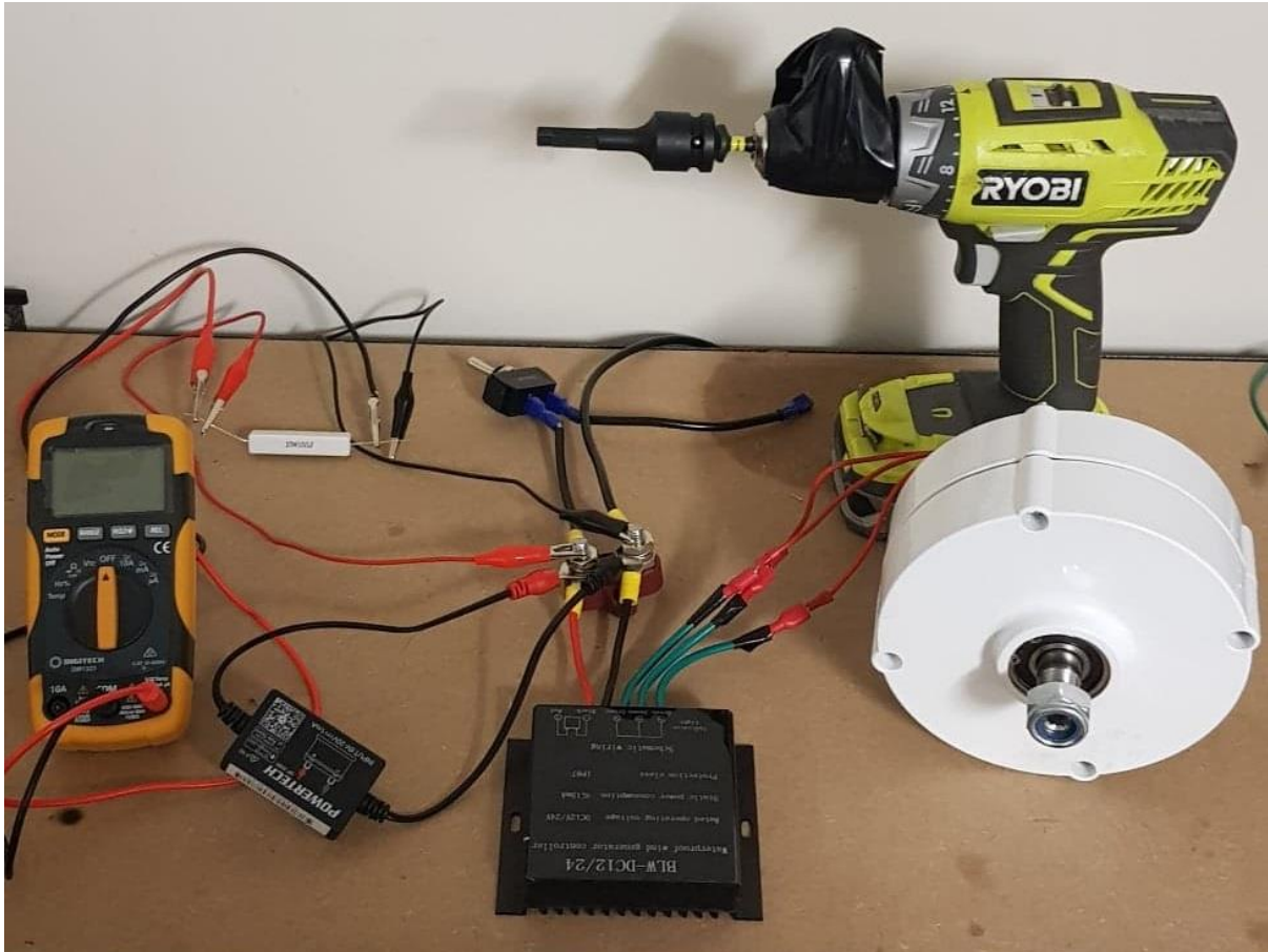
Figure 54: The electrical component test assembly
