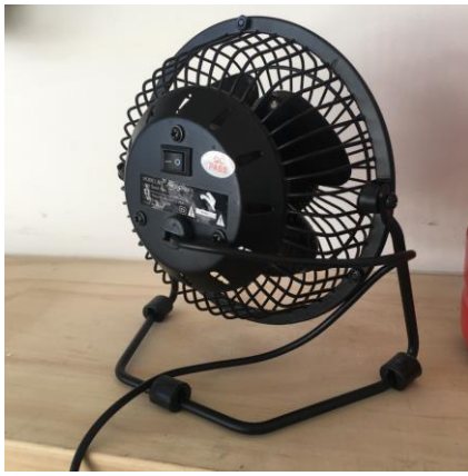
Figure B1.6: Use of mini fans to assist with fumes
