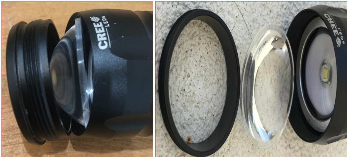
Figure 5.1: LED torch threaded lens cap demonstrates possible modular design option for ease of disassembly
