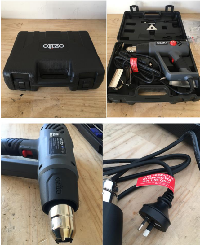
Figure B1.9.2: Heat gun used during component removal.
