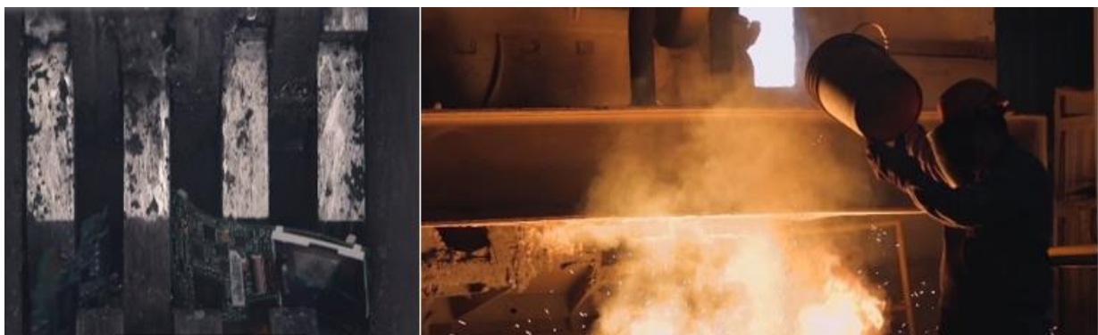
Figure 2.13: Electronic scrap shredded and melted for metal recovery (Mobile Muster 2020).
