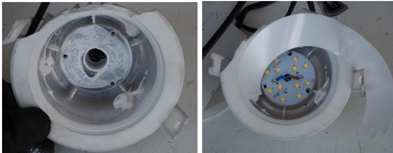
Figure 4.2: Downlight LED Board removal process
