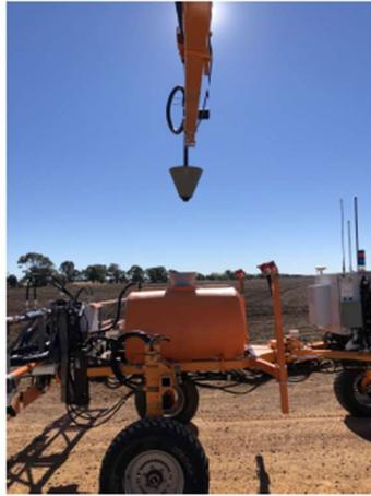
(a) The alignment of the refill hose prior to being lowered
