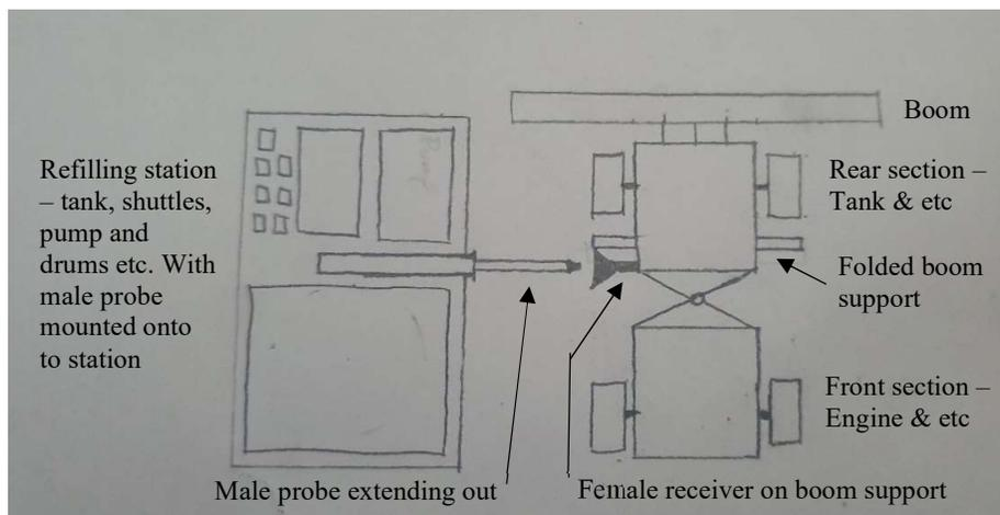
Figure 24: Chosen concept sketch for alternative design
