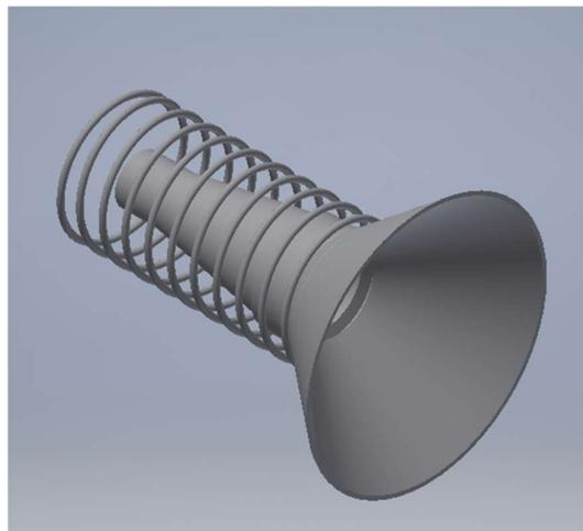
Figure 38: Original spring concept for female component
