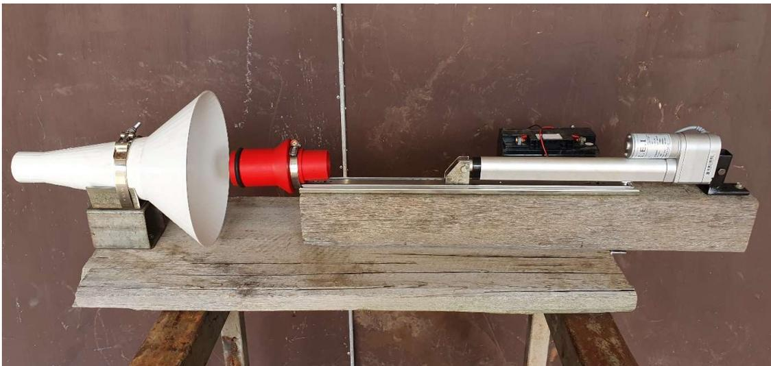
*Figure 29: Test rig fully retracted and inline. Female component is white, male is red.*
