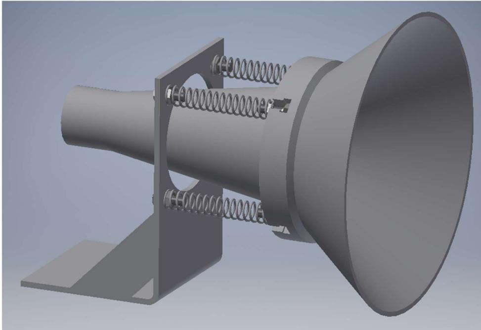
*Figure 40: Sprung mounting system for female component*
