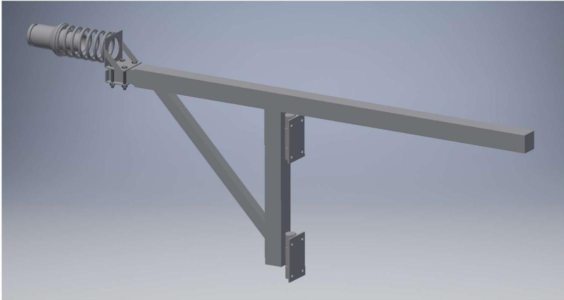
*Figure 42: Male probes telescoping and hinged frame - retracted*
