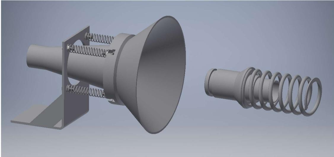
*Figure 41: Sprung female mount with male probe and spring*
