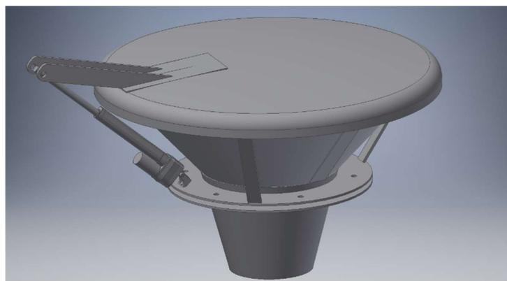
*Figure 37: Braced and mounted receiver with mock actuator and lid*
