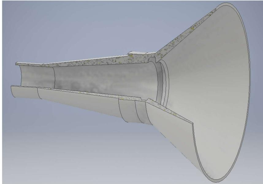
*Figure 27: Female component, aka receiver, cross sectional profile*
