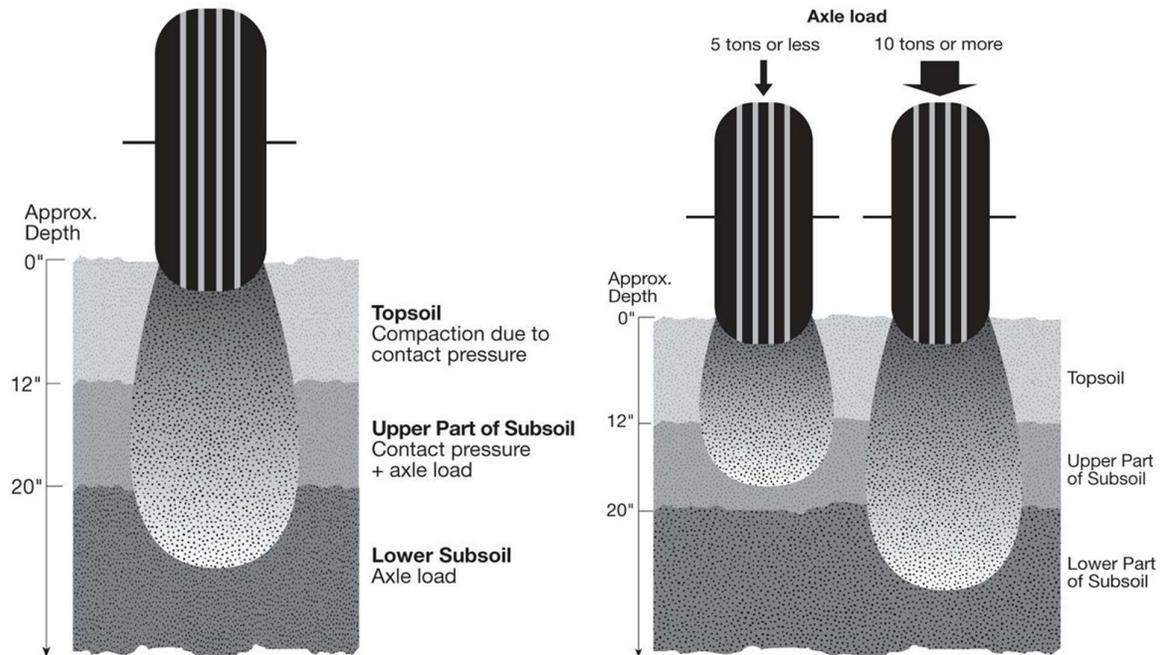
Figure 1: Effects of axle loadings on different sections of soil – illustrations by Duiker (2005)
