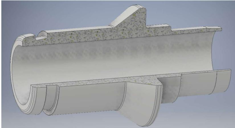
*Figure 26: Male component, aka "piston"/probe cross sectional profile*
