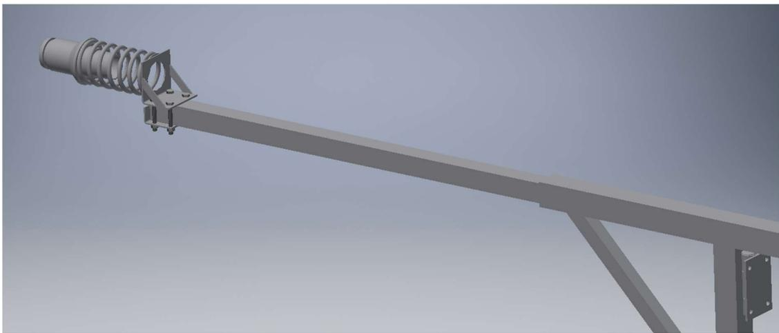
*Figure 43: Male probes telescoping and hinged frame - extended*
