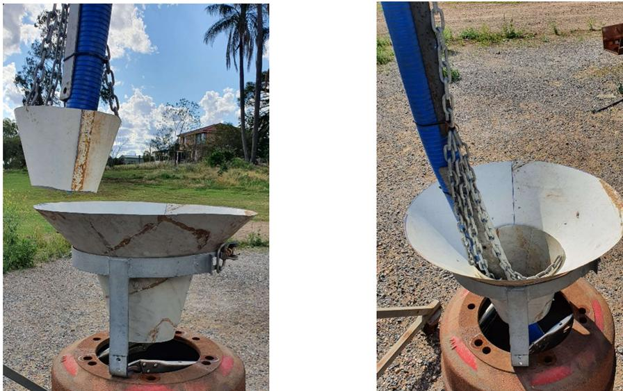
Figure 23: Trial 2 setup at maximum offset (LEFT), with successful connection (RIGHT)
