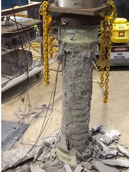
Specimen #2 “T” – 6 x 15.9mm dia. bars after failure
