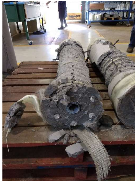
Specimen #2 “T” – 6 x 15.9mm dia. bars after failure
