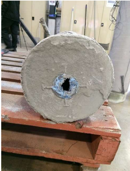
Specimen #7 “C” – GFRP spirals and HCRS after failure
