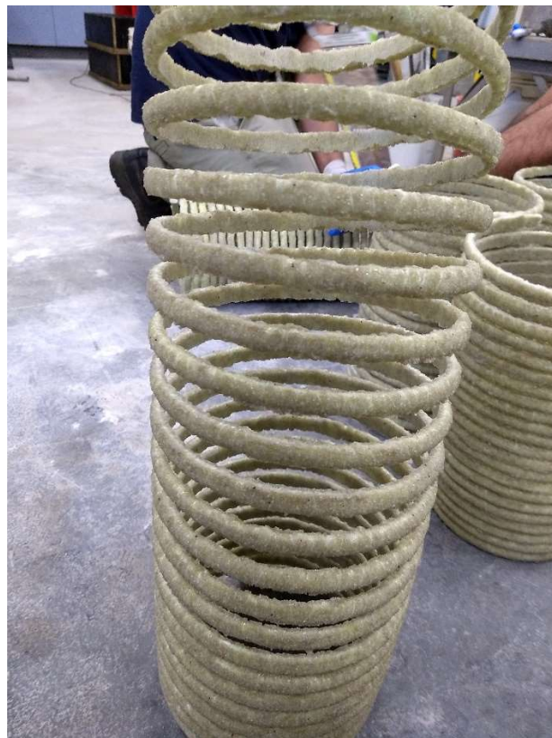
Figure 2: Sand-coated GFRP Spirals (9.5mm nominal diameter)
