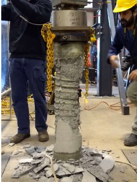
Specimen #8 “C” – GFRP spirals after failure
