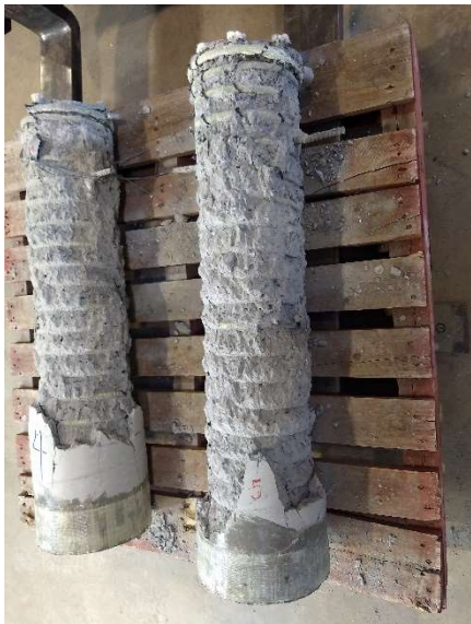
Specimen #5 “T” – 8 x 15.9mm dia. bars after failure
