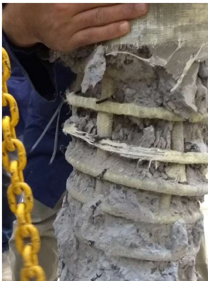
Specimen #6 “C” – 6 x 15.9mm dia. bars (no HCRS) after failure
