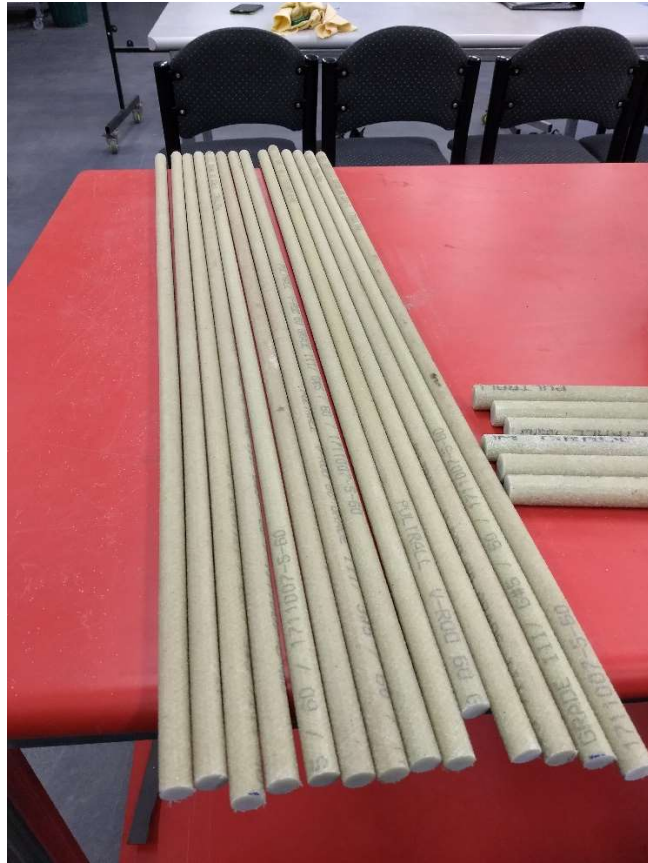
Figure 1: Sand-coated GFRP Bars (15.9mm nominal diameter)
