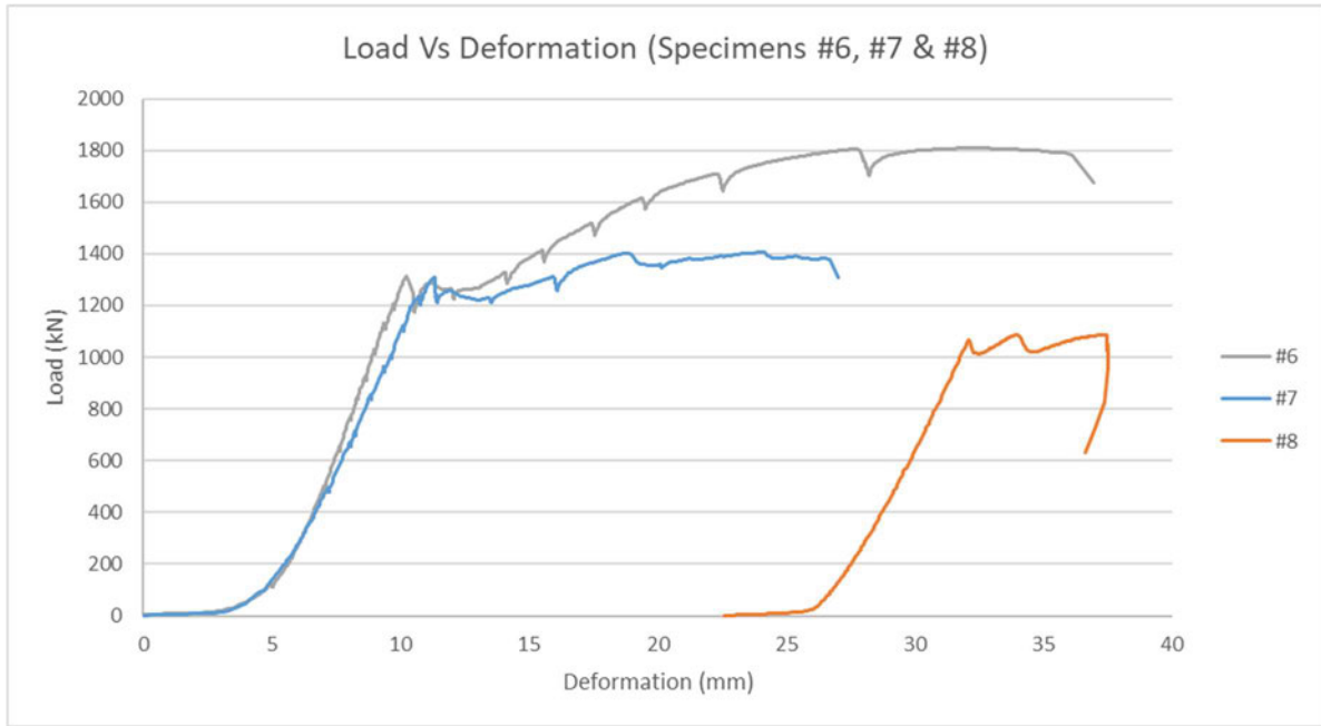
Figure 14 - Axial load and deformation behaviour of the Controlled concrete columns
