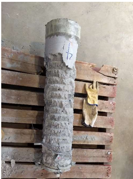
Specimen #4 “T” – 4 x 15.9mm dia. bars after failure
