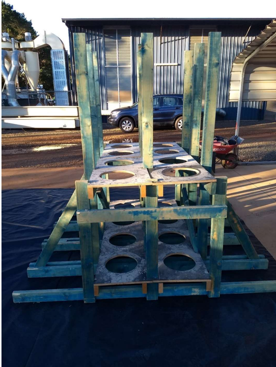
Figure 9: Timber formwork supporting the concrete column specimens
