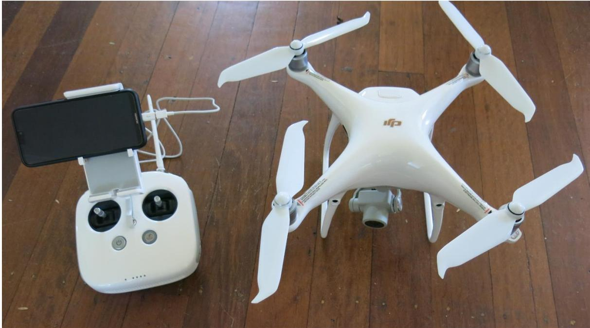
Figure 21: DJI Phantom 4 Pro V2.0 quadcopter UAV and controller with smartphone connected by usb cable
