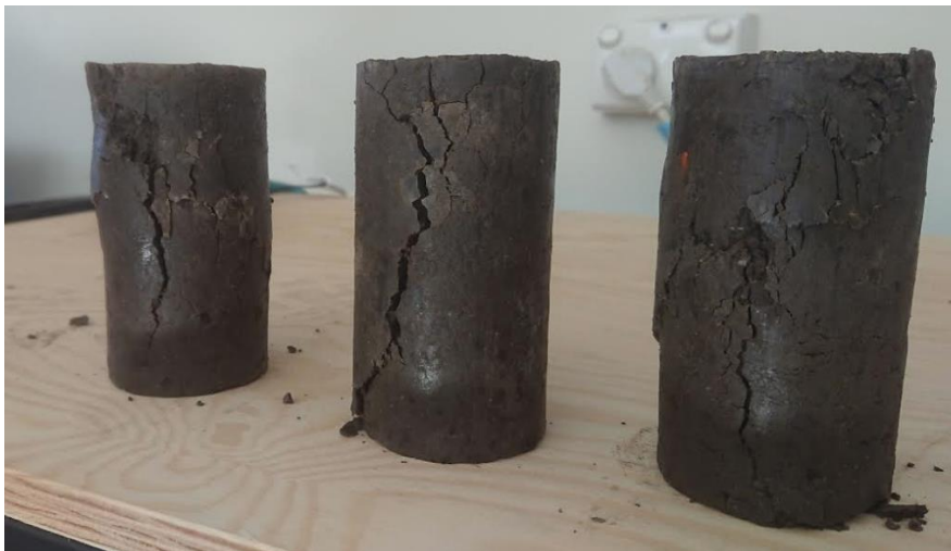
Figure 34- Brittle failure of all three fly ash treated samples (Author 2019)
