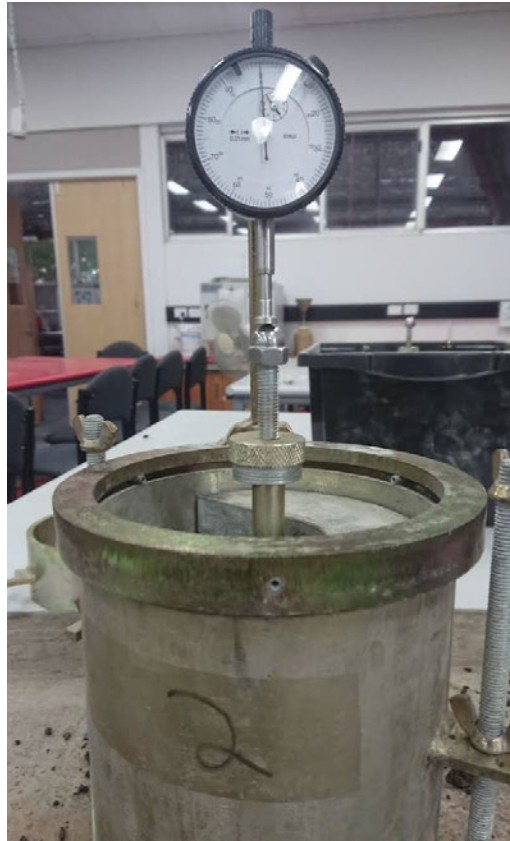
Figure 20- Zeroing dial gauge for swell reading (Author 2019)
