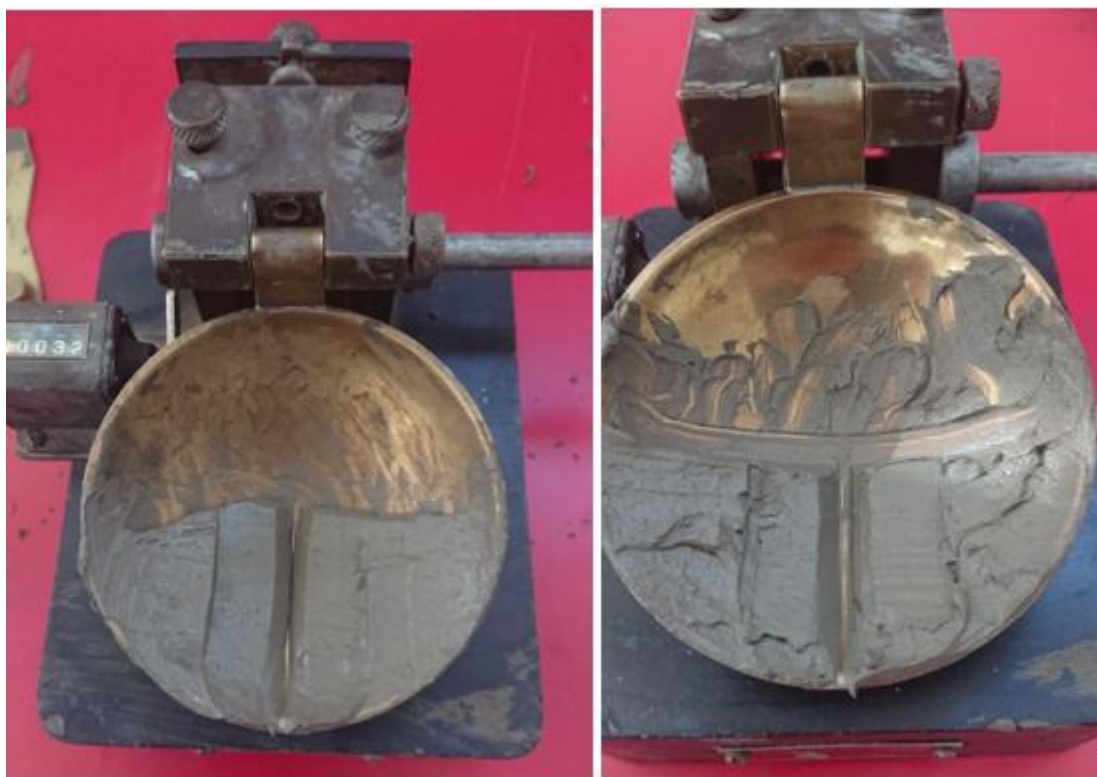
Figure 19- Casagrande bowl liquid limit test (Author 2019)
