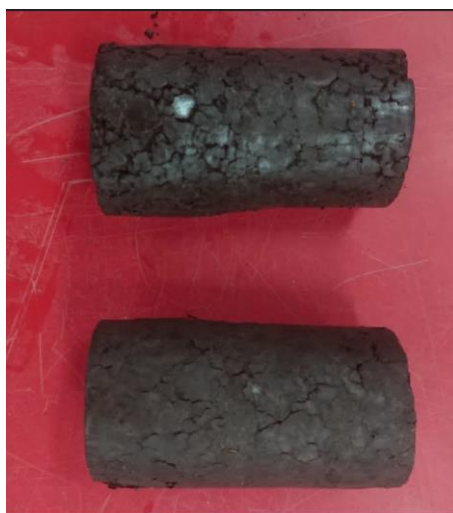
Figure 31- Plastic failure of untreated sample (Author 2019)
