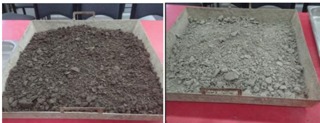
Figure 22- Clay sample before and after addition of fly ash (Author 2019)
