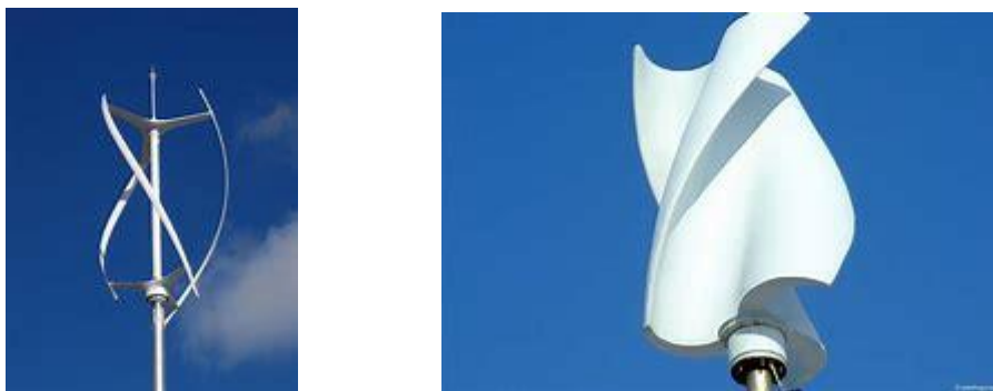
Figure 4.2: Example of VAWT, a Darrieus (left) and Savonius (right). (Source: Webb, 2007)
