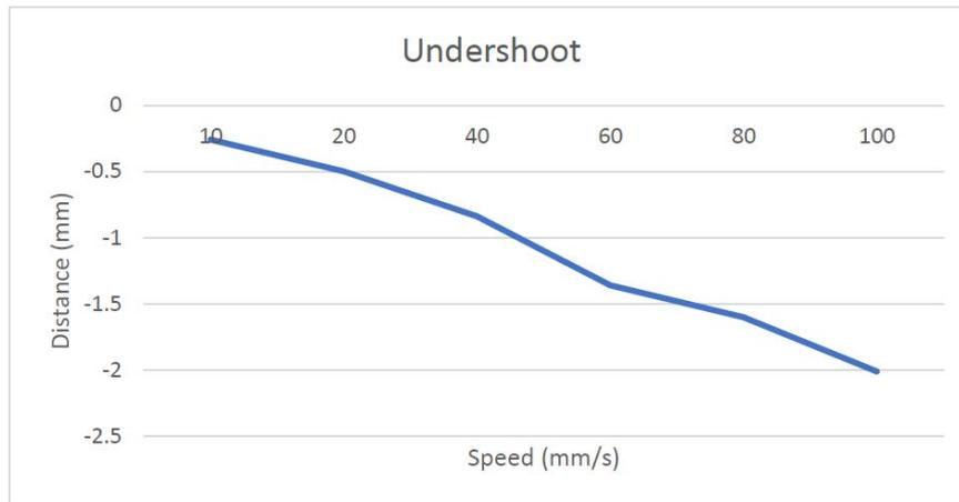
Figure 4.3: Undershoot curve for collision avoidance tests with  $t_r = 40$  ms
