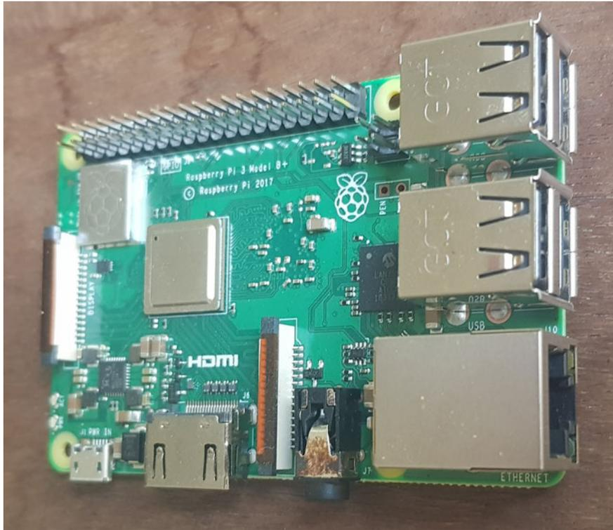
Figure 3.1: Photo of Raspberry Pi 3 Model B+ used for development.
