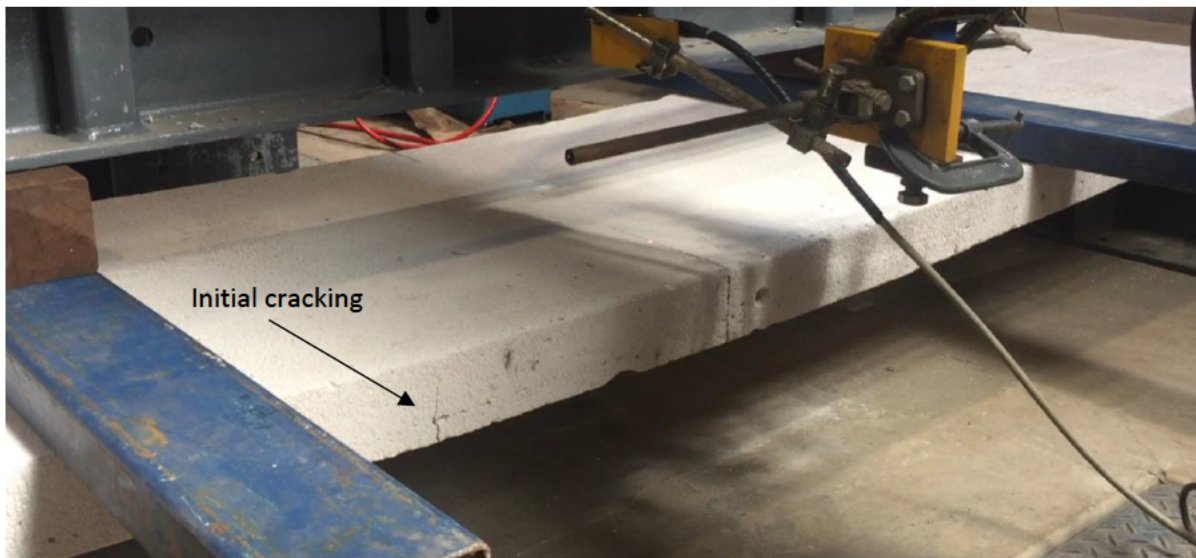
Figure 4.5 - Test Sample 1 Initial Cracking
