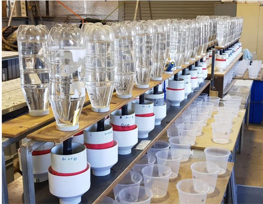
**Figure 54 Hydraulic Conductivity experimental set up**
