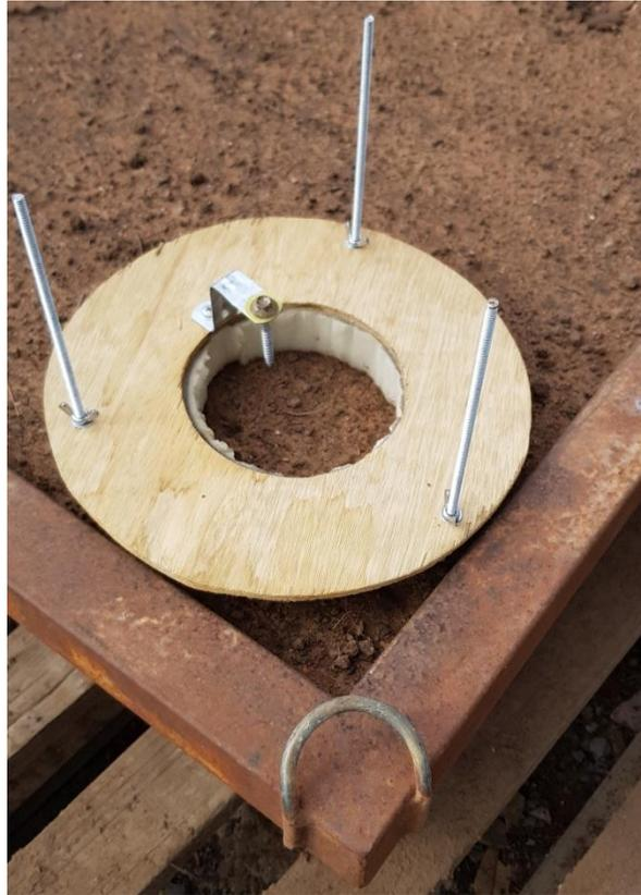
Figure 50 Water Replacement Method Apparatus
