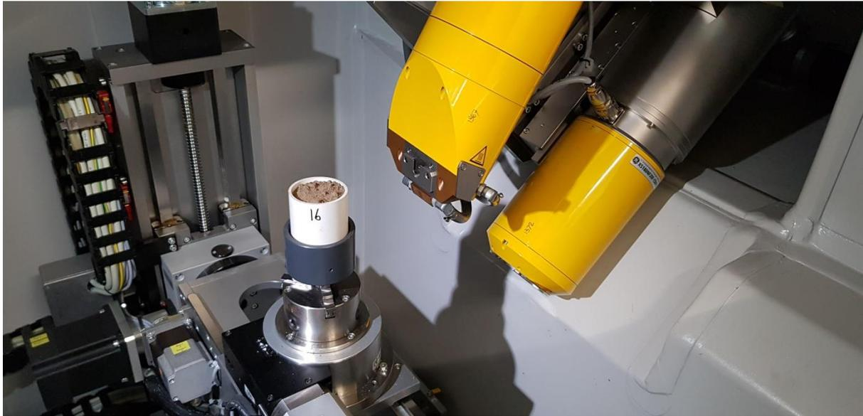
Figure 53 Soil core on mount in X-ray CT scanner
