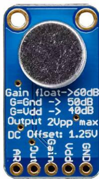
Figure 3.4: MAX9814 Microphone with AGC (Core Electronics 2019)
