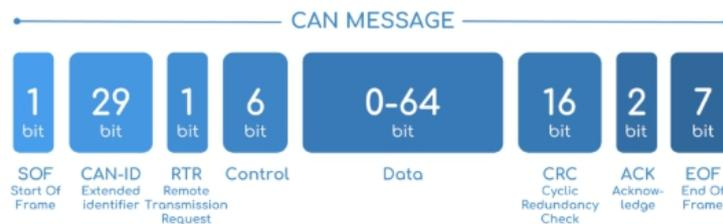
Figure 2.20: CAN bus message breakdown (CSS Electronics 2019)
