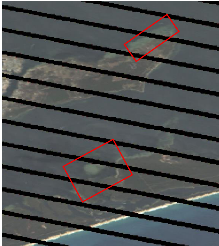
Figure 3.2 Diagonal data gaps run through Point King and Waddy Island study sites, in images between 2004 and 2017.
