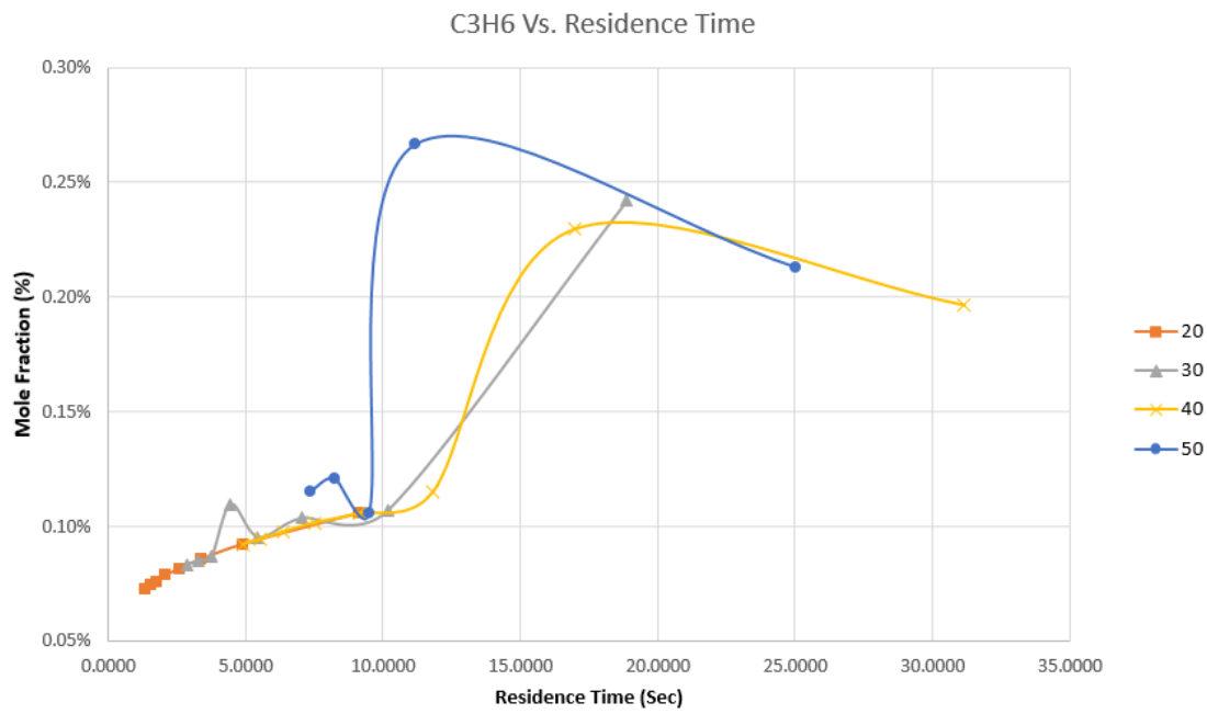
Figure 4.21: Identified Cyclopropane Fraction vs residence time
