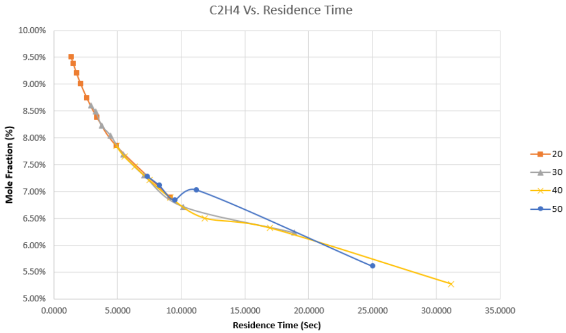
Figure 4.25: Identified Ethylene Fraction vs residence time
