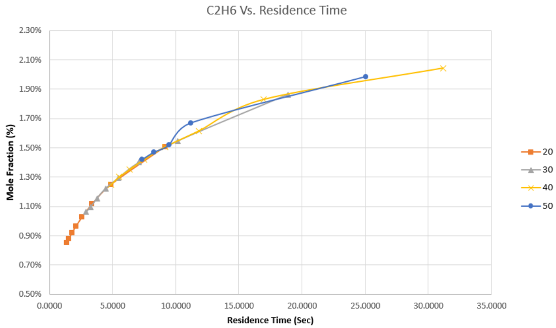
Figure 4.23: Identified Ethane Fraction vs residence time
