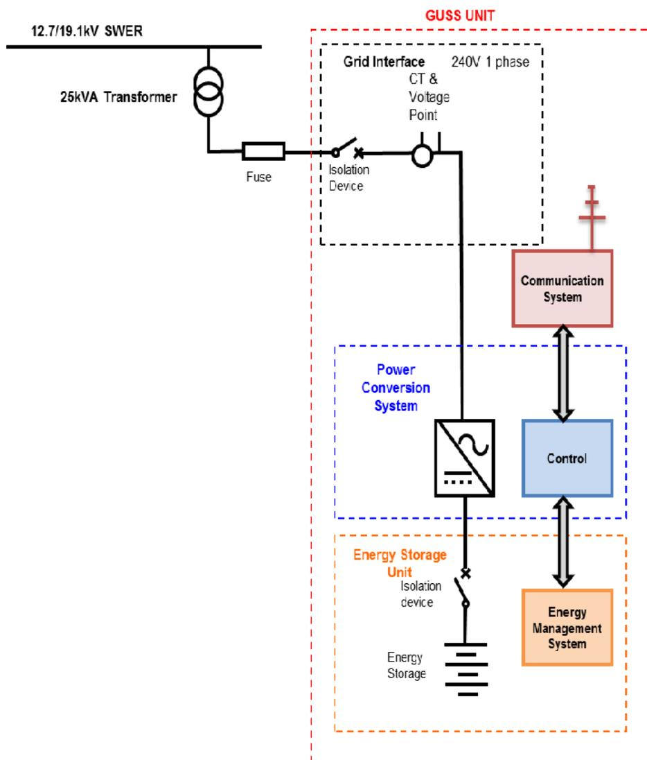
Figure 32: GUSS Unit Connected Configuration and Control (Taylor 2015)
