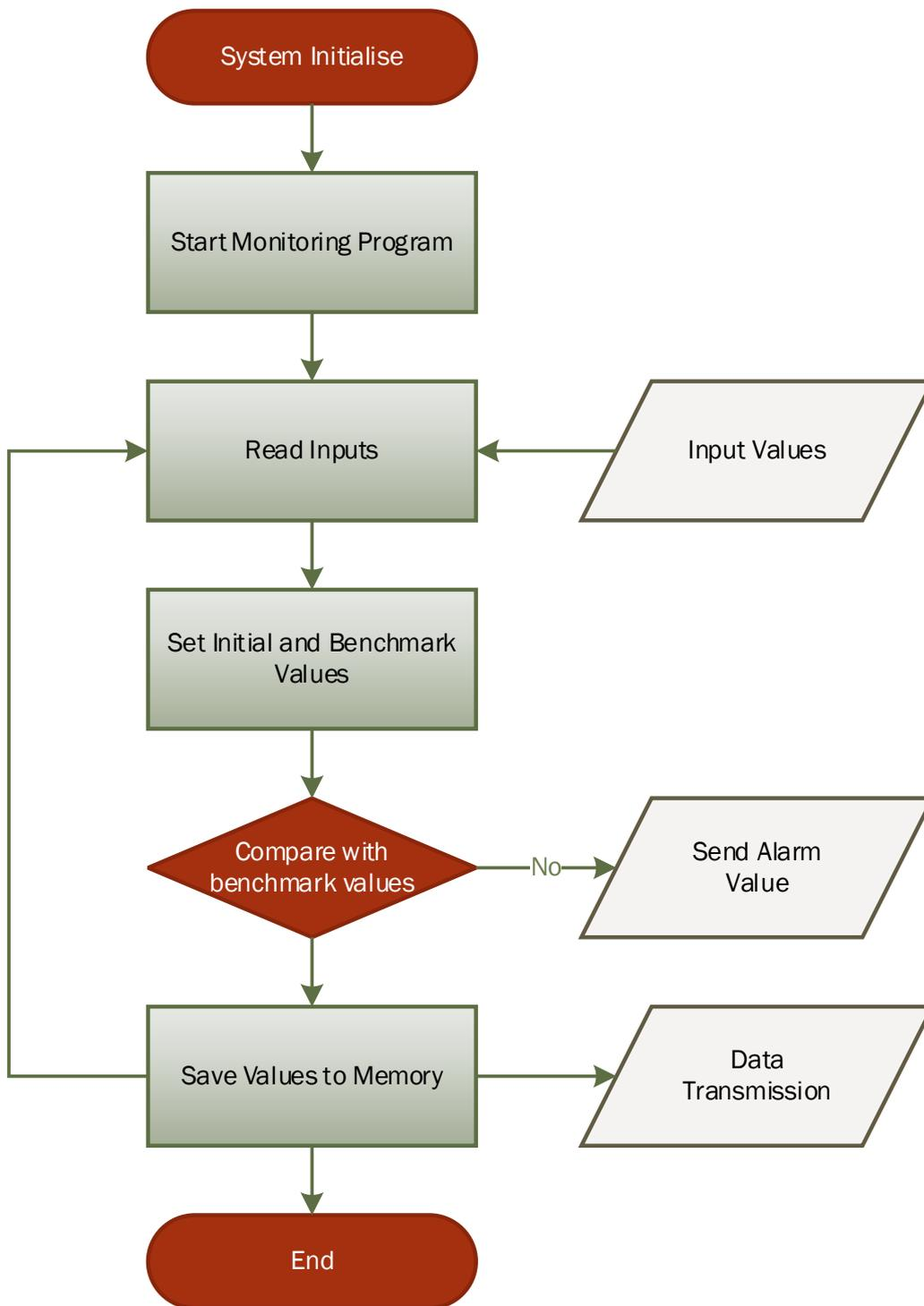
**Figure 111: Program Flowchart for SWER Earth Monitoring Device**
