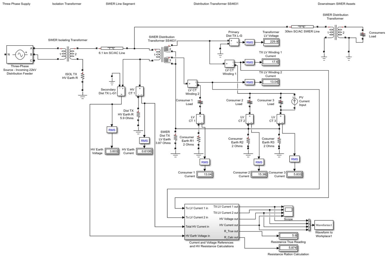
Figure 107: SWER Base Model with HV Earth Monitoring Subsystem
