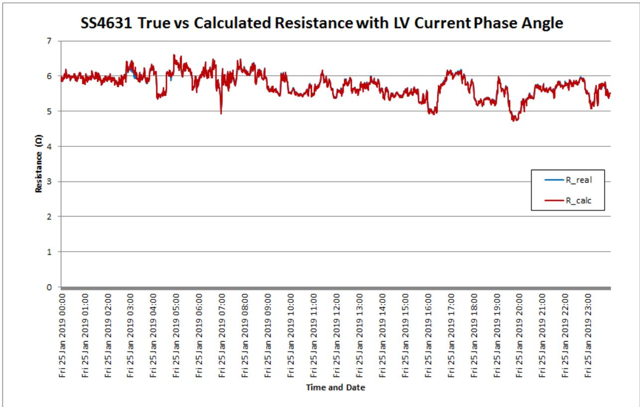
Figure 93: SS4631 True HV Earth Resistance vs Calculated HV Earth Resistance for 25<sup>th</sup> January 2019 with Current Phase Angle
