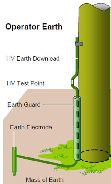
**Figure 52: Diagram of Passive or Operator Earth (Ergon Energy 2017)**
