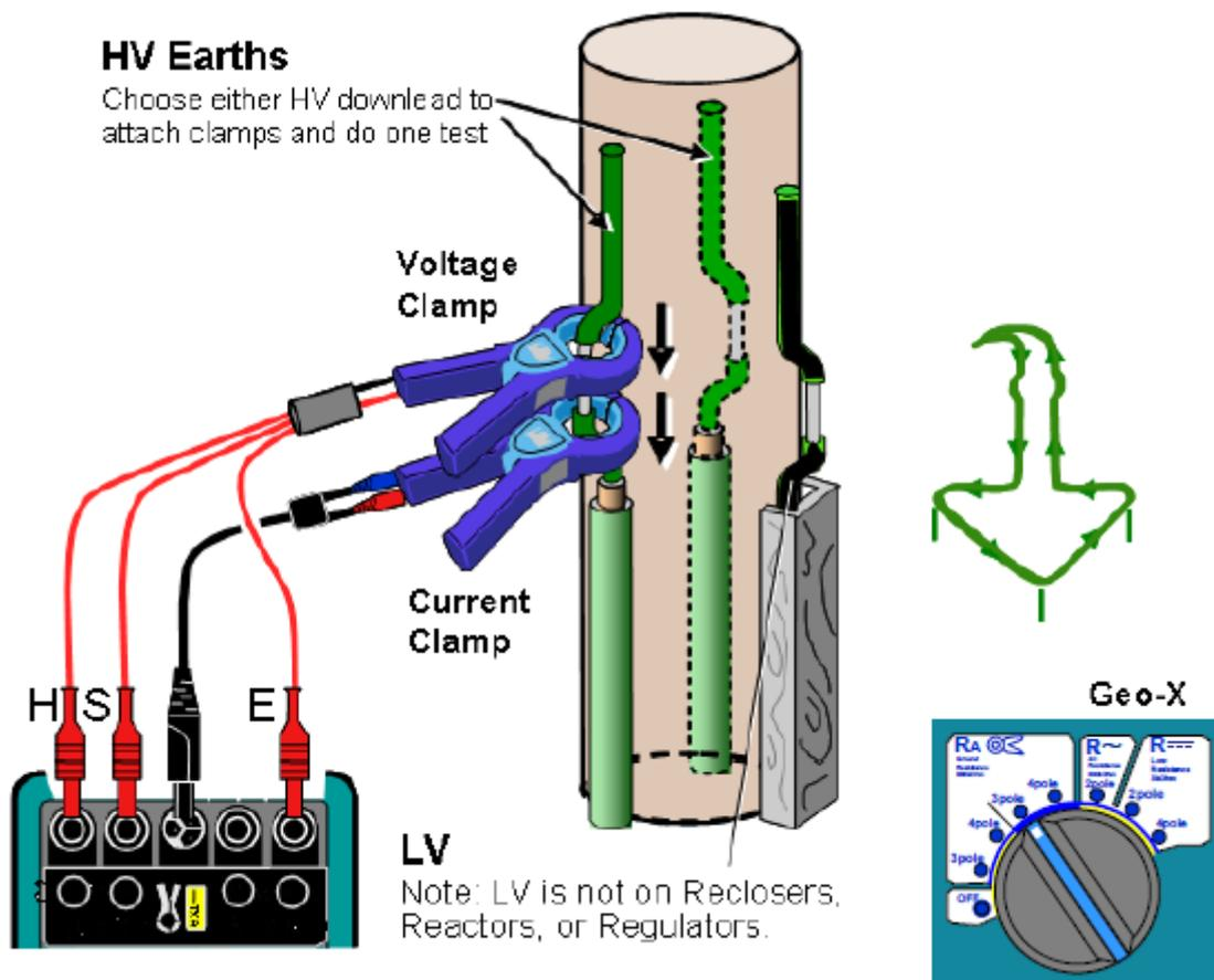
Figure 55: 2 Clamp Loop Resistance HV SWER Earth Continuity Test (Ergon Energy 2017)
