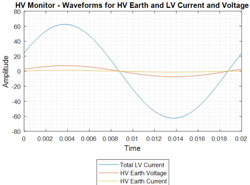
Figure 108: HV Earth Monitoring Subsystem MATLAB Waveform Output Plot
