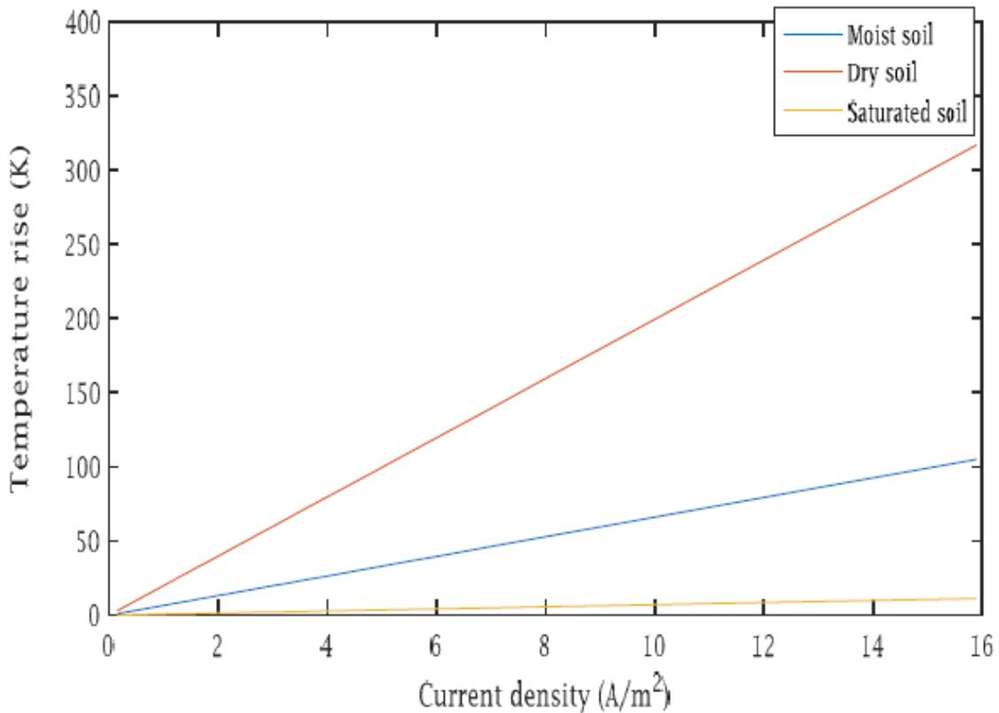
**Figure 50: Current Density vs Temperature Rise (Noorudheen, Wolfs & Alahakoon 2016)**
