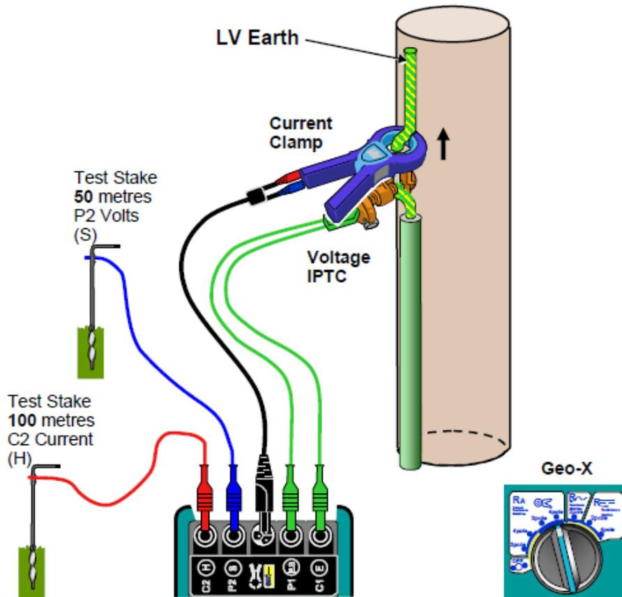
Figure 57: Grid Neutral LV SWER Earth Test Method (Ergon Energy 2017)
