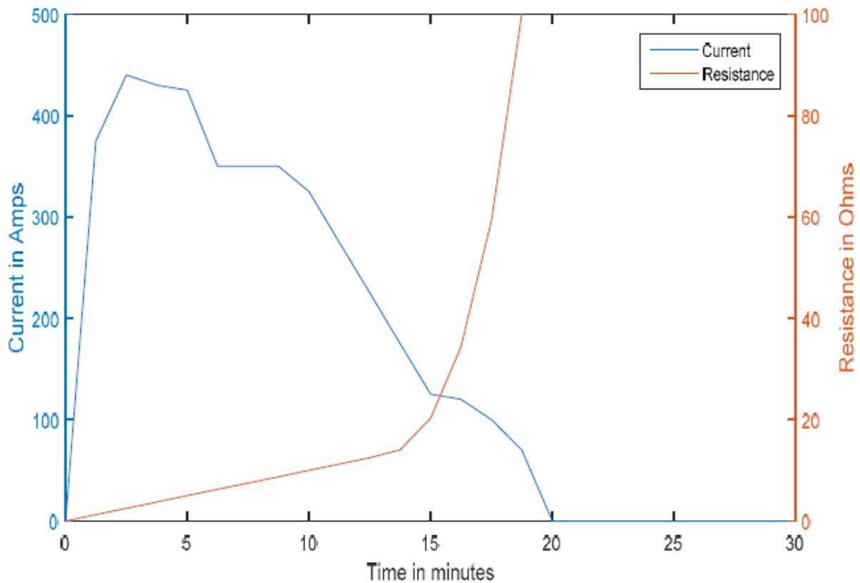
**Figure 49: Variation of Resistance and Current with time in Overloaded Electrodes (Noorudheen, Wolfs & Alahakoon 2016) (Taylor 1935)**
