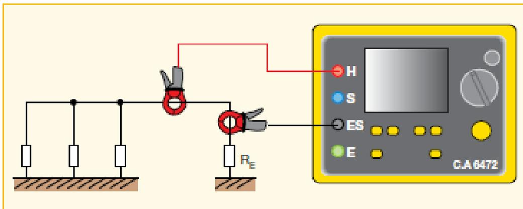
Figure 15: Earth Loop Resistance Measurement with Two Clamps Method (Megger 2010)
