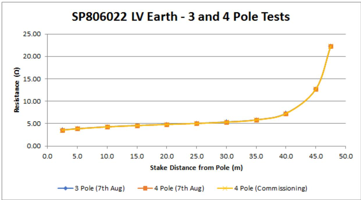
Figure 116: SP806022 LV Earth – 3 and 4 Pole Tests
