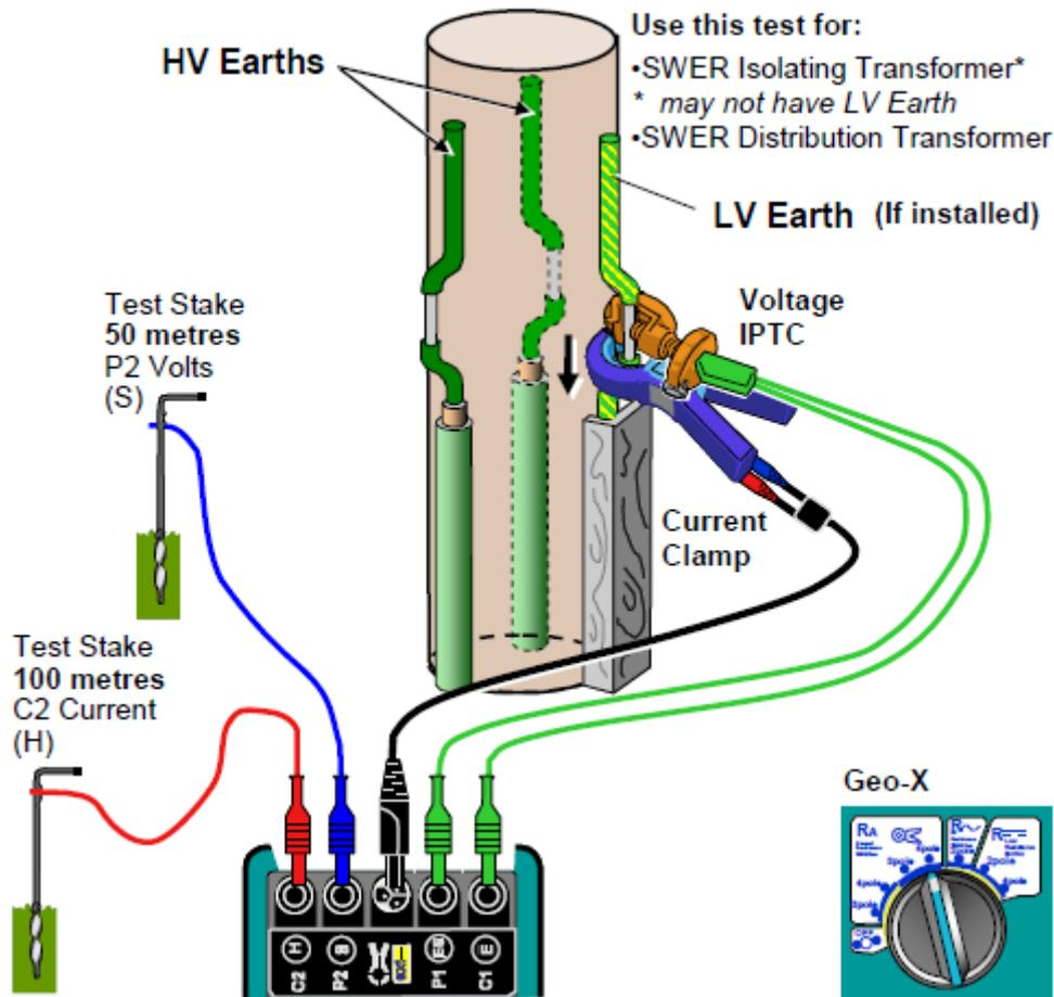
Figure 56: 4 Pole Selective LV SWER Earth Test Method (Ergon Energy 2017)
