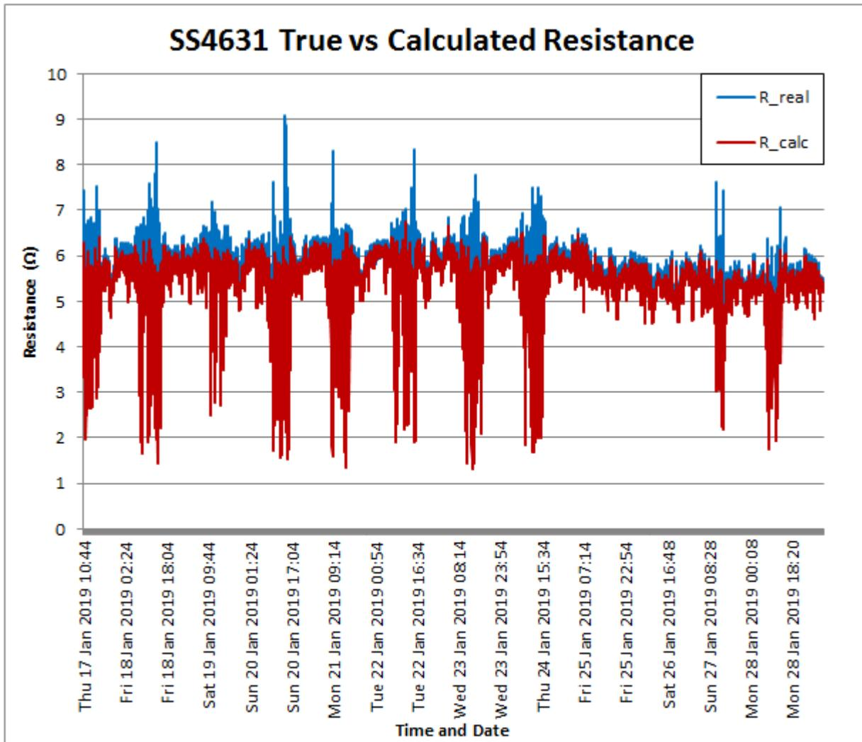
**Figure 83: SS4631 True HV Earth Resistance vs Calculated HV Earth Resistance over 11 days**
