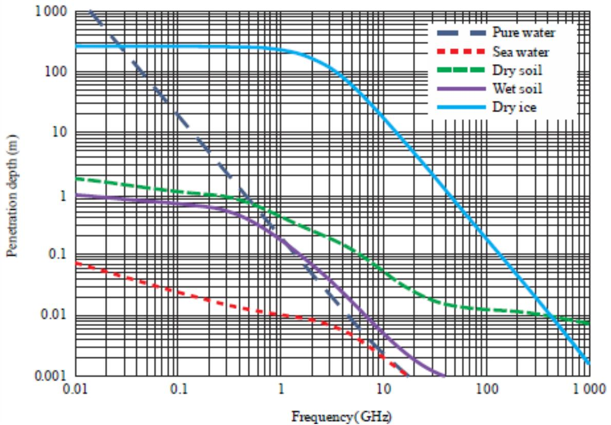
**Figure 40: Electrical Characteristics of the Surface of the Earth (Radiocommunication Sector of ITU 2017)**
