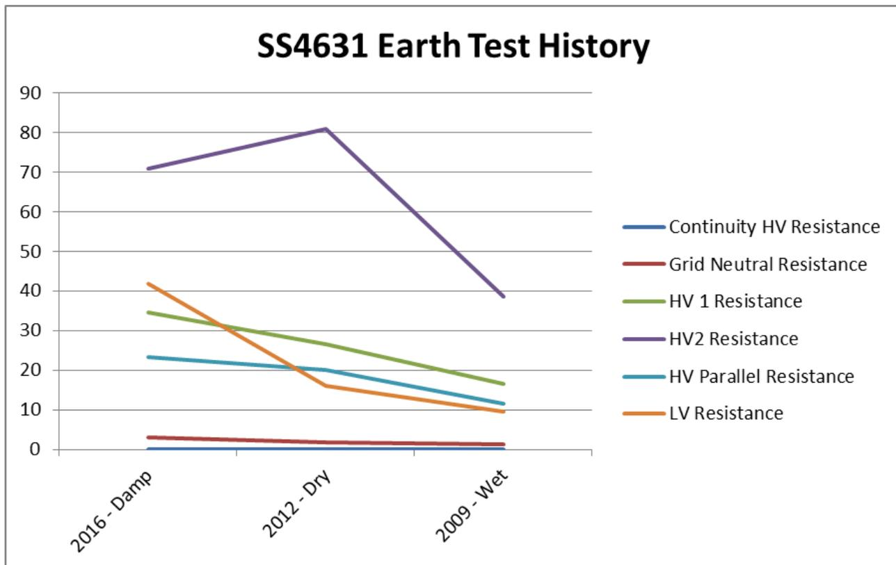
Figure 61: Earth Test History from 2009 to 2016 for SWER Distribution Transformer SS4631
