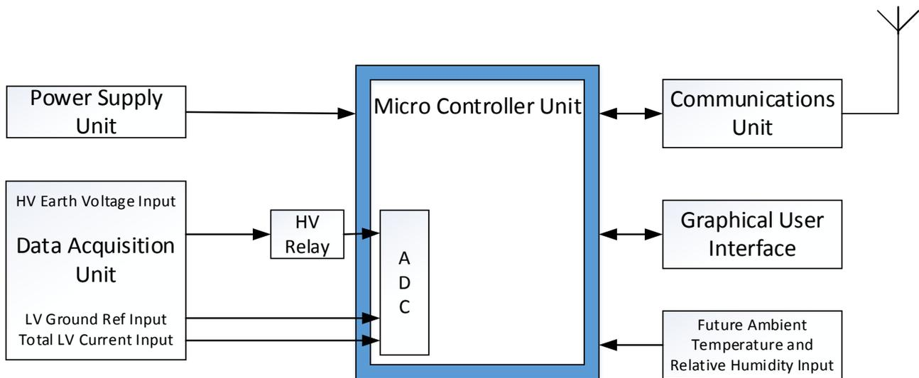
**Figure 109: System Architectural Overview for SWER Earth Monitoring Device**
