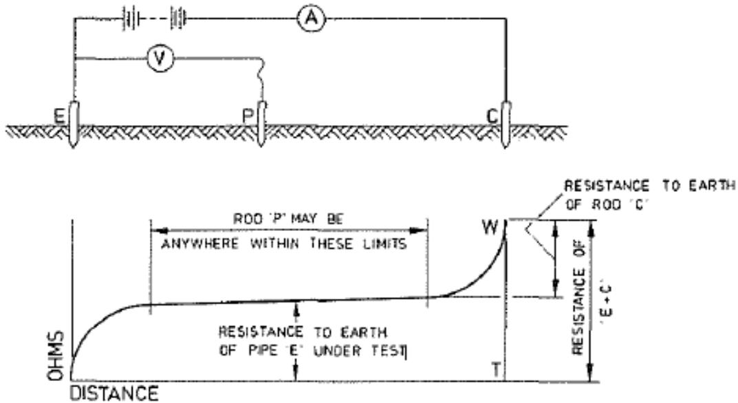
Figure 12: Fall of Potential Generic Resistance Plot (The Electricity Authority of New South Wales 1975)
