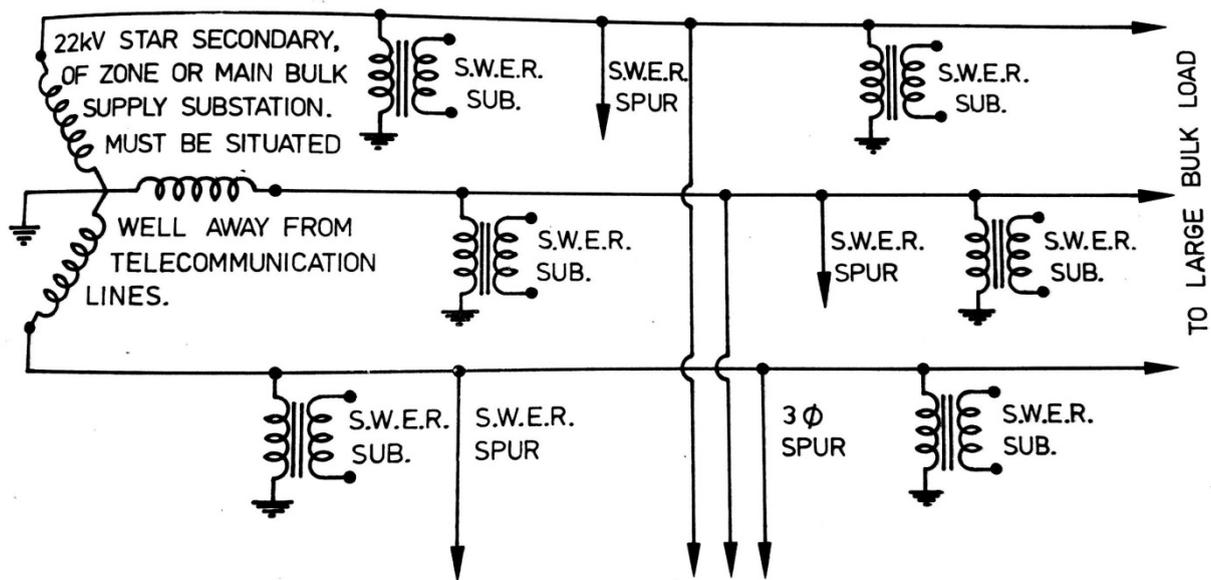
**Figure 28: Triplex SWER System (The Electricity Authority of New South Wales 1978)**
