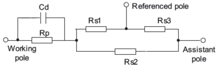
**Figure 19: Circuit Model for Three-Pole System (Cong-li & Minfang 2007)**
