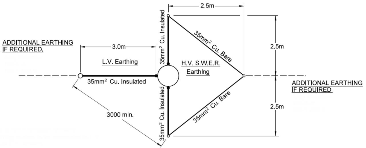
Figure 45: SWER Transformer Earth on Wood Pole (Distribution Network Standards 2018)
