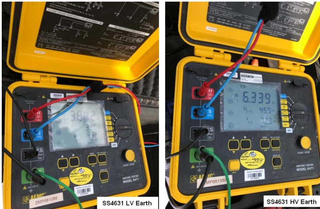
**Figure 73: SS4631 Earth Test Readings 7th January 2019**
