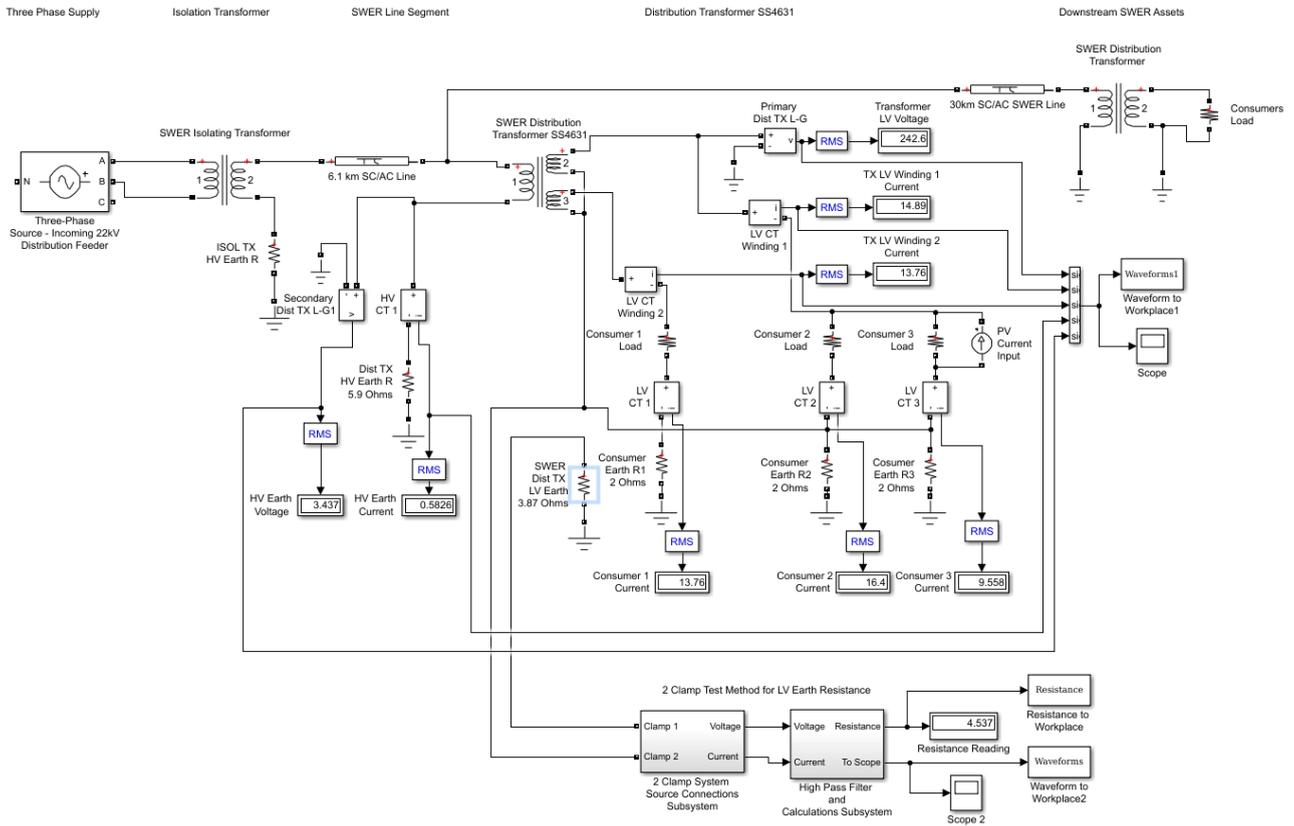
Figure 102: Two Clamp Test Model Connected to the Base SWER Model
