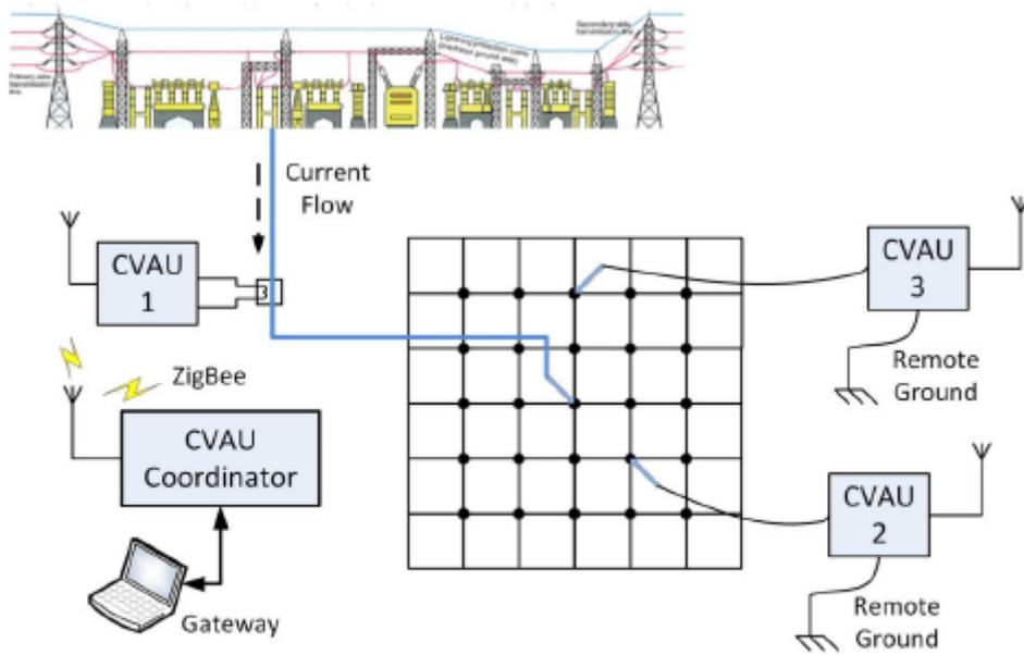
Fig. 1. Overview of the current and voltage acquisition unit (CVAU) arranged to monitor current and voltage at certain points of the electrical grounding grid.
