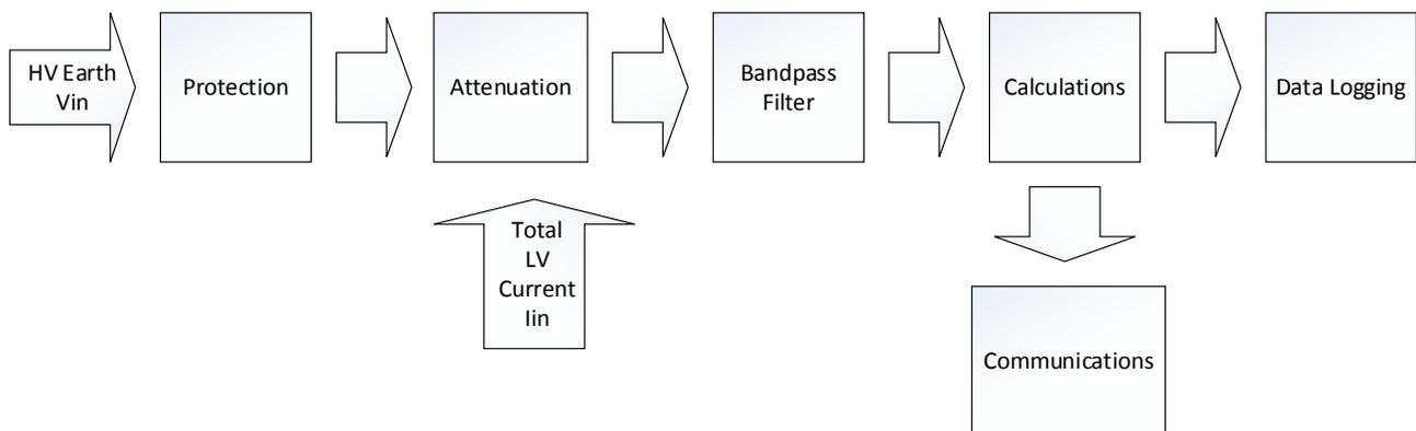
**Figure 110: Software System Flow Diagram for SWER Earth Monitoring Device**
