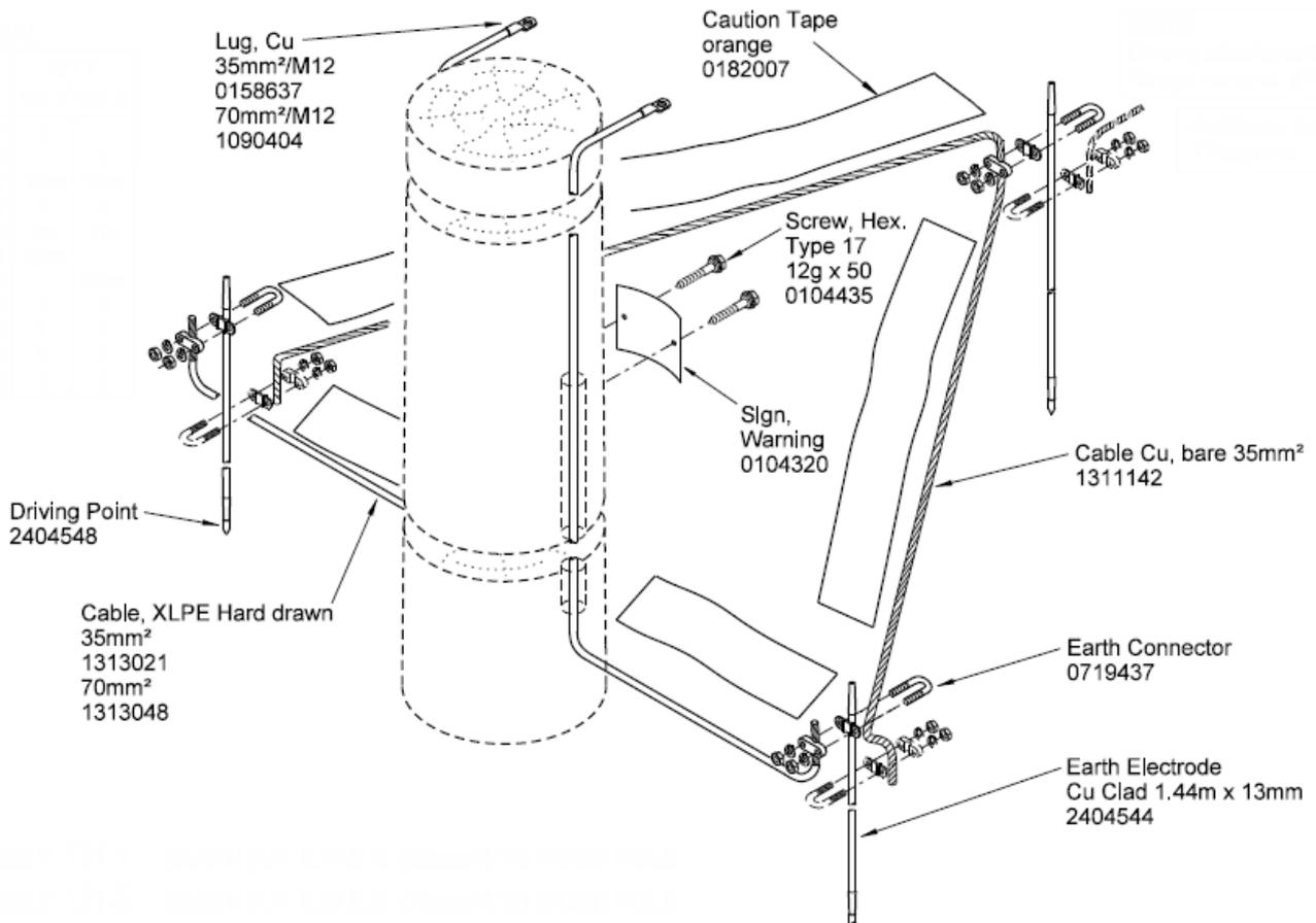
Figure 46: HV SWER Earth to Wood Pole (Distribution Network Standards 2018)
