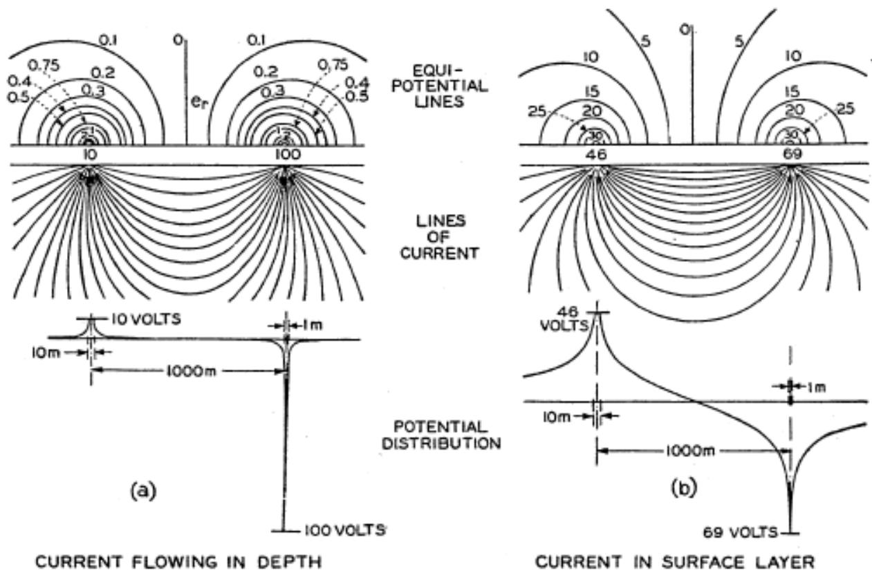
Figure 42: Current Streamlines around Spherical Electrodes (Rudenberg 1945)
