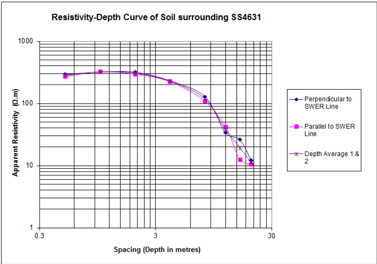
Figure 74: SS4631 Soil Resistivity-Depth Curve Results 17th January 2019
