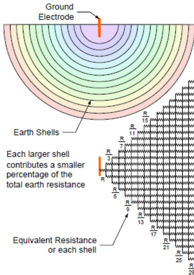
Figure 6: Concentric Earth Shells Around an Earth Electrode (Gill 2009) (Reeve Engineers 2008)
