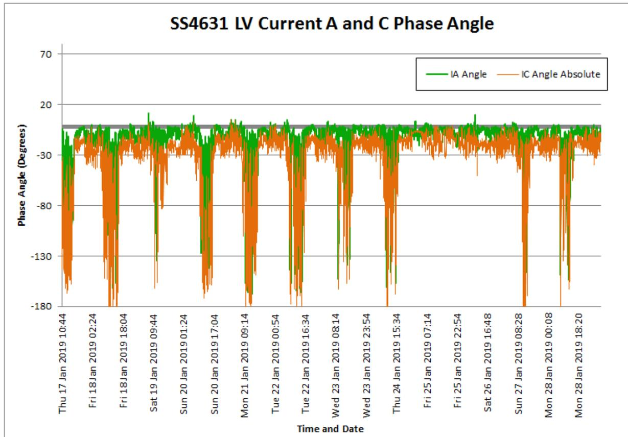
Figure 88: SS4631 Phase Angle of the LV Current for Two Windings
