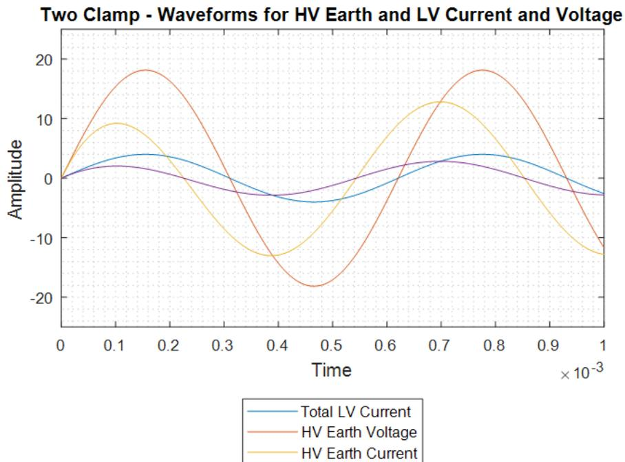
Figure 103: Waveform for Earth Current and Voltage from the Two Clamp Test Method
