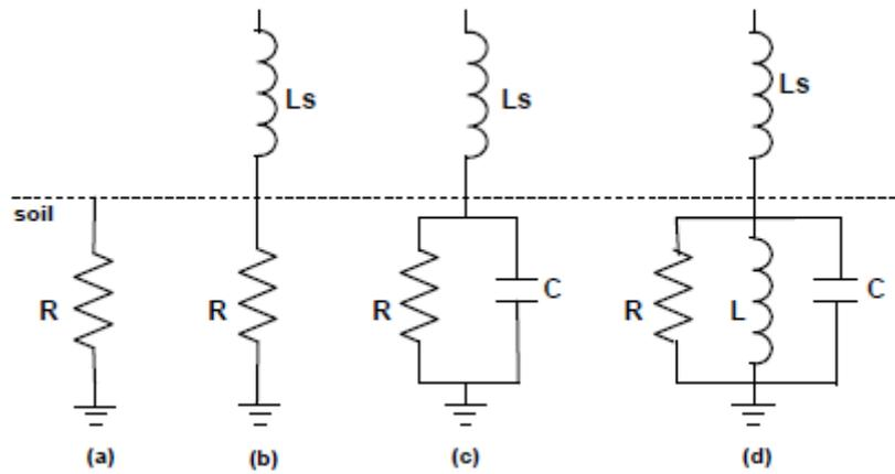
**Figure 22: Equivalent Circuit of a Rod (Aguiar et al. 2009)**
