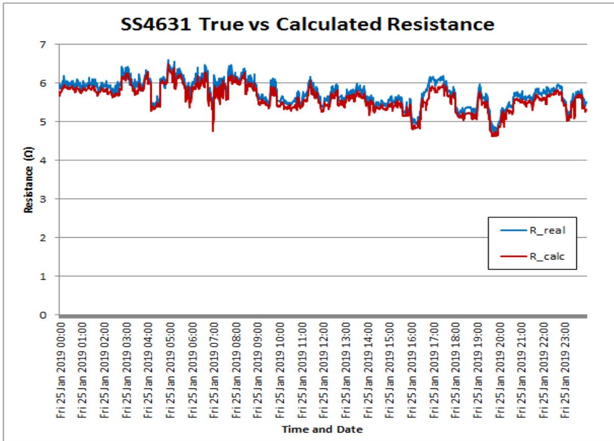
**Figure 86: SS4631 True HV Earth Resistance vs Calculated HV Earth Resistance for 25<sup>th</sup> January 2019**
