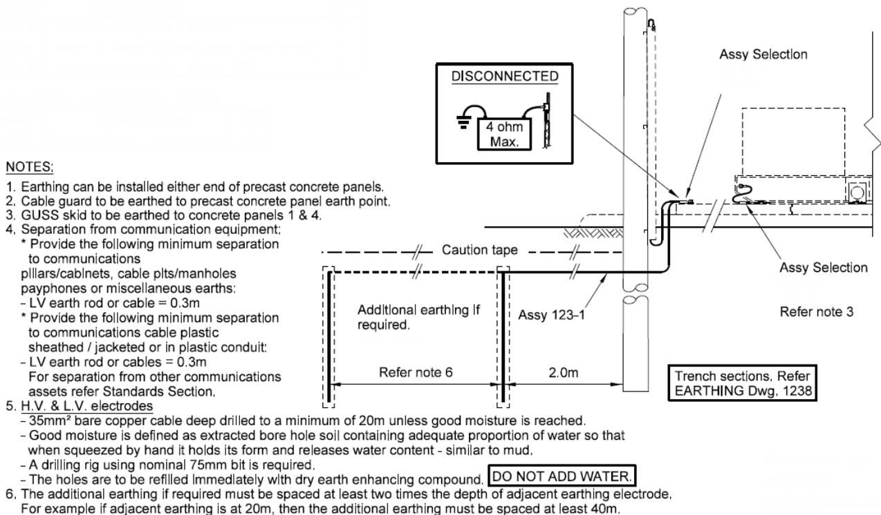
**Figure 33: MEN Earth Configuration for GUSS Units – Deep Drilled (Distribution Network Standards 2018)**
