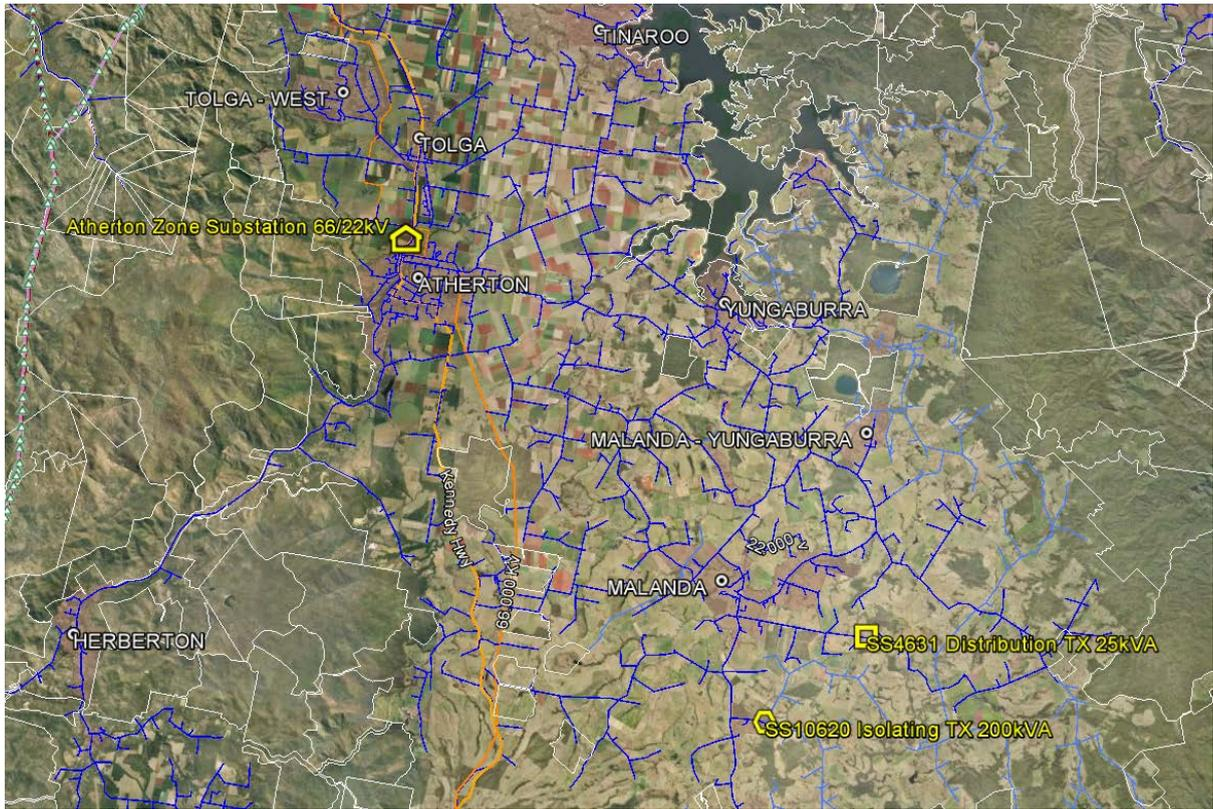
**Figure 68: Aerial View of SS4631 in Relation to the SWER Isolating Transformer and Main Zone Substation**
