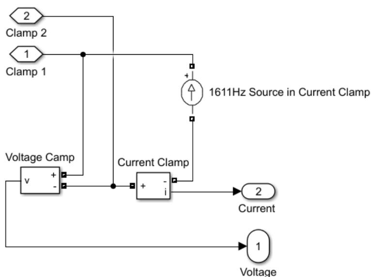
Figure 99: Two Clamp Test Method Subsystem
