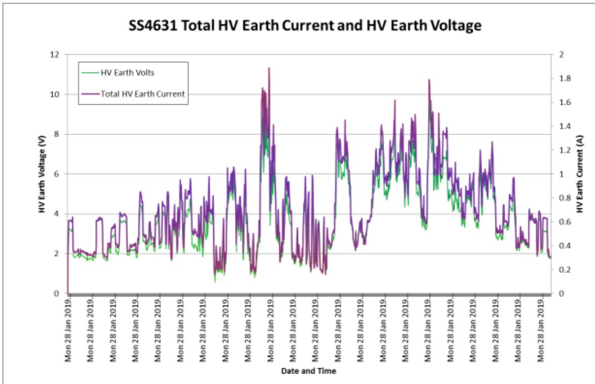
Figure 80: PowerMonic PM45 Analyser HV Earth Current and HV Earth Voltage SS4631
