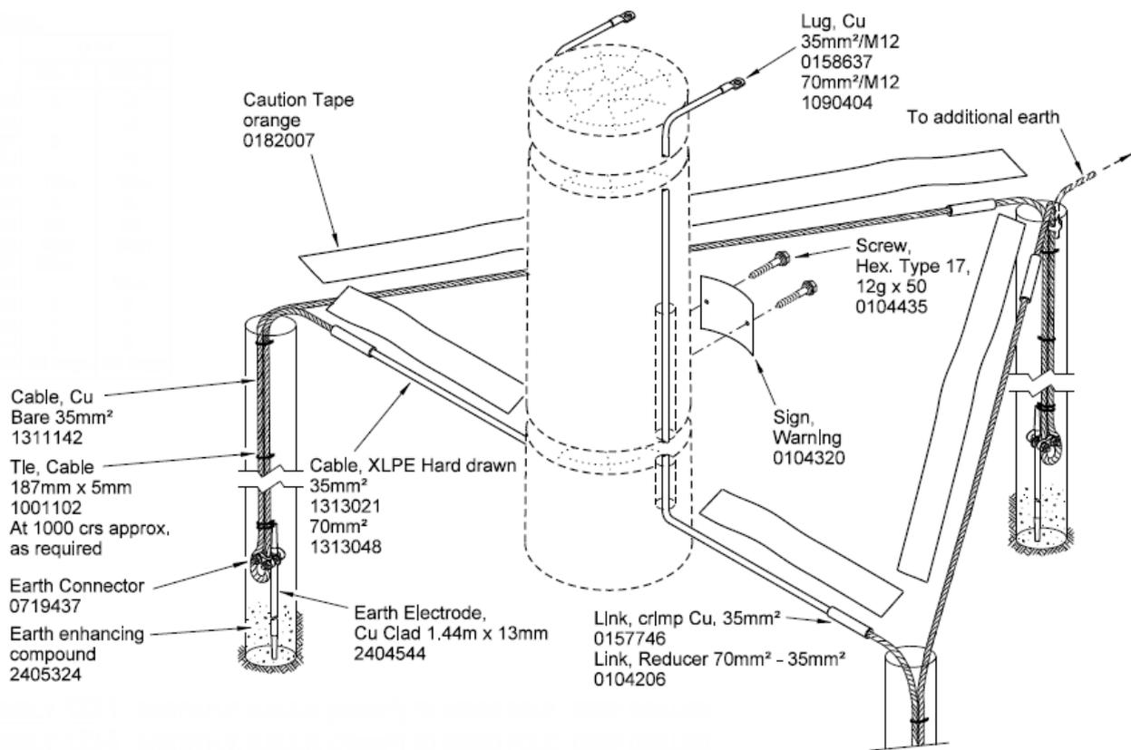
**Figure 48: HV SWER Earth to Wood Pole – Deep Drilled (Distribution Network Standards 2018)**
