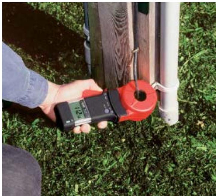
Figure 17: Stake-less Clamp-On Method Unit (Megger 2010)
