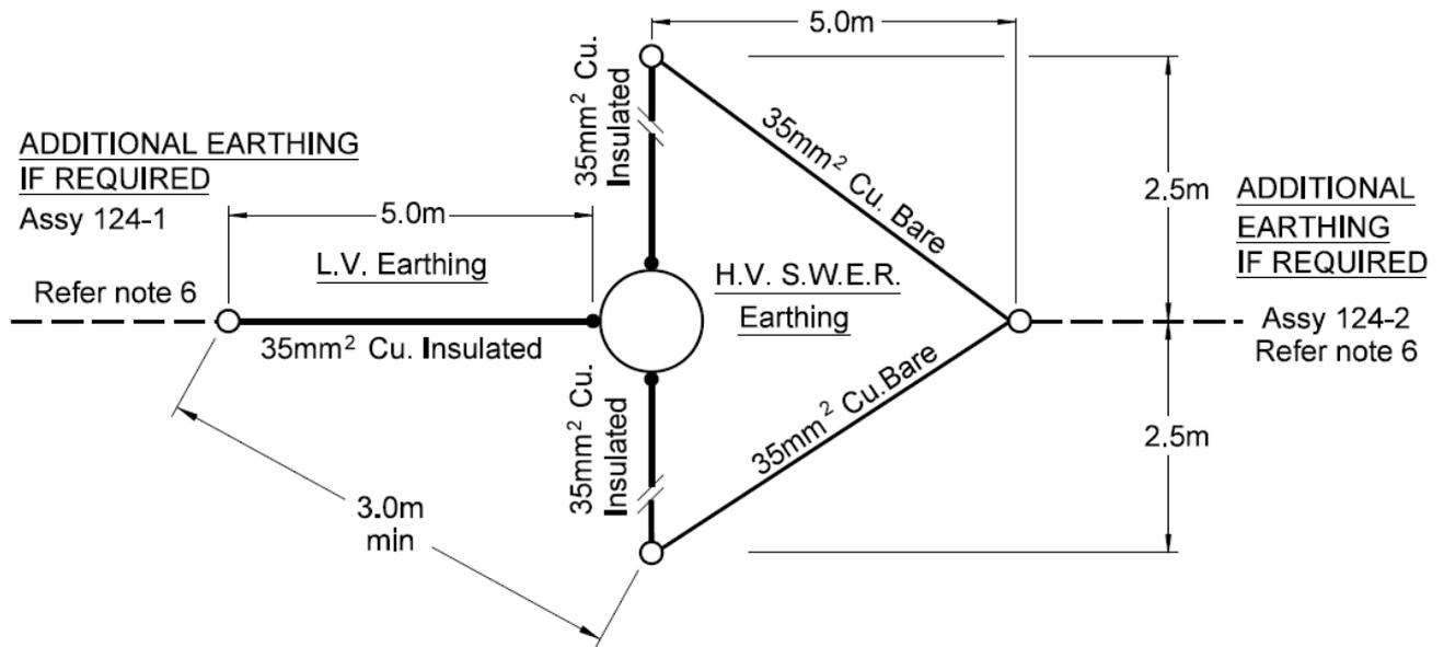
**Figure 47: SWER Isolator/Transformer Earth on a Wood Pole, Deep Drilled (Distribution Network Standards 2018)**
