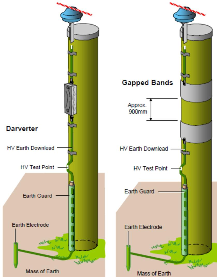
Figure 51: Darverters and Gapped Bands (Ergon Energy 2017)
