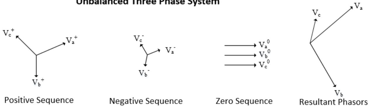
**Figure 24: Three Phase Sequence Voltages Balanced and Unbalanced**
