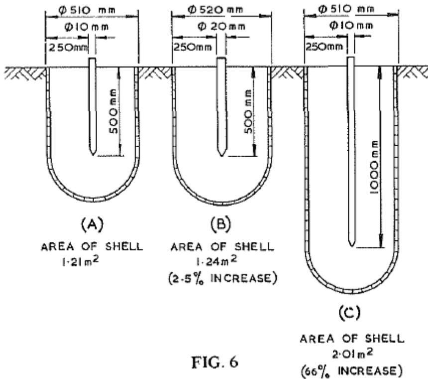
Figure 7: Shell Hemispheres around Electrodes (The Electricity Authority of New South Wales 1975)
