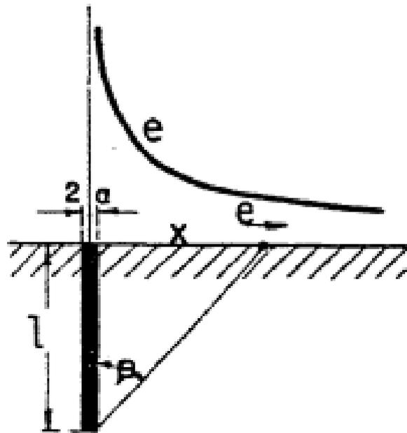
**Figure 41: Dimensions of a Driven Rod and the Field Strength on the Surrounding Surface (Rudenberg 1945)**
