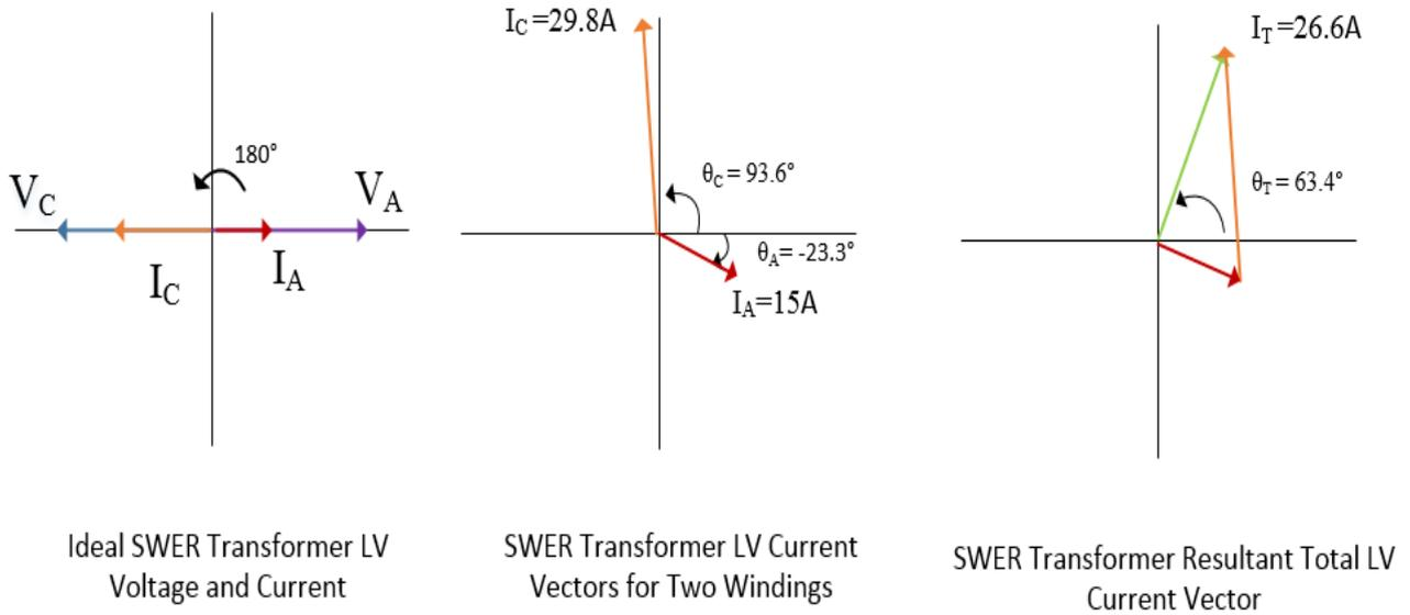
Figure 87: SWER Distribution Transformer LV Voltage and Current Vectors
