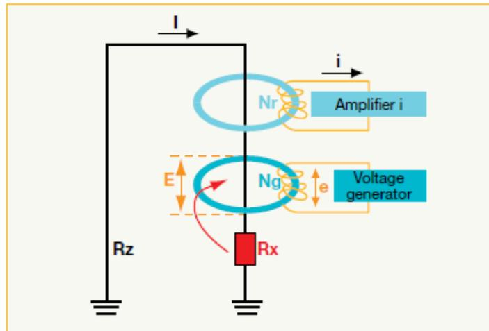
Figure 16: Stake-less Clamp-On Method Diagram (Megger 2010)
