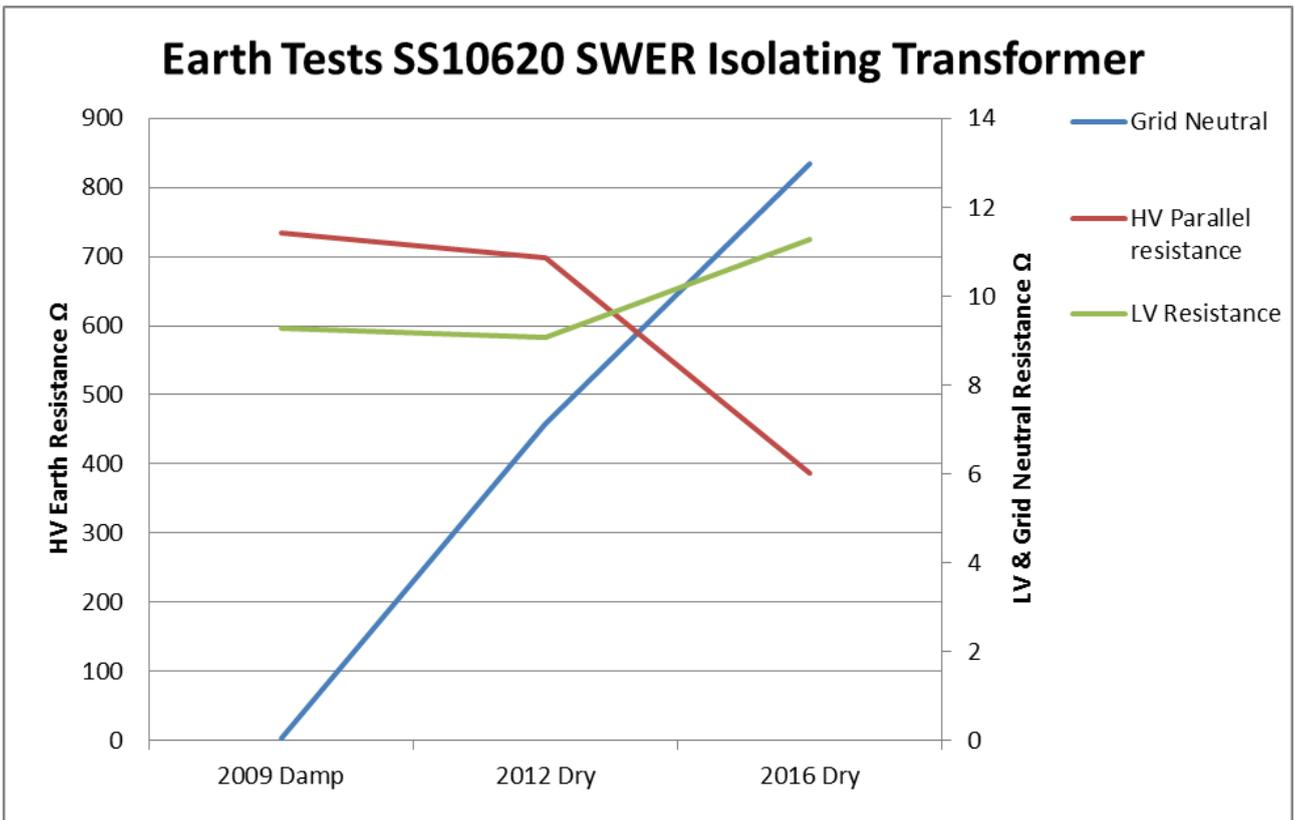
Figure 69: SS10620 SWER Isolating Transformer Historical Earth Tests
