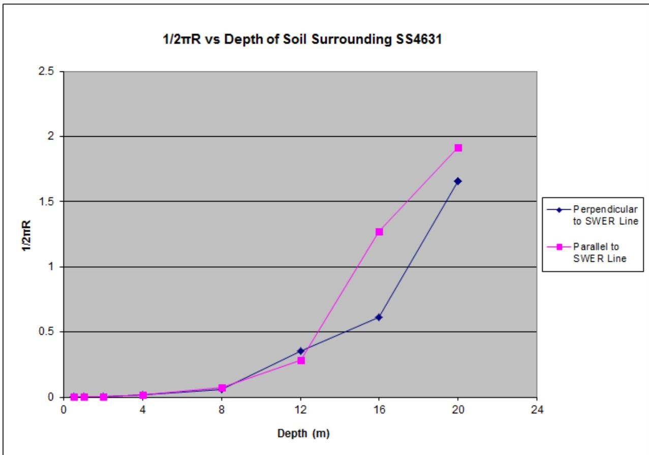
Figure 75: SS4631 Soil Resistivity Inverse Slope Results 17th January 2019
