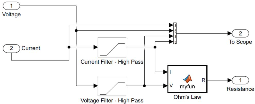
**Figure 100: Two Clamp Model High Pass Filter and Ohm's Law Function**
