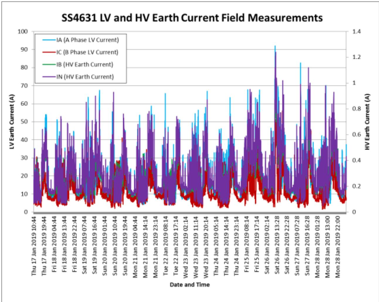
**Figure 78: PowerMonic PM45 Analyser Raw Current Data for SS4631**
