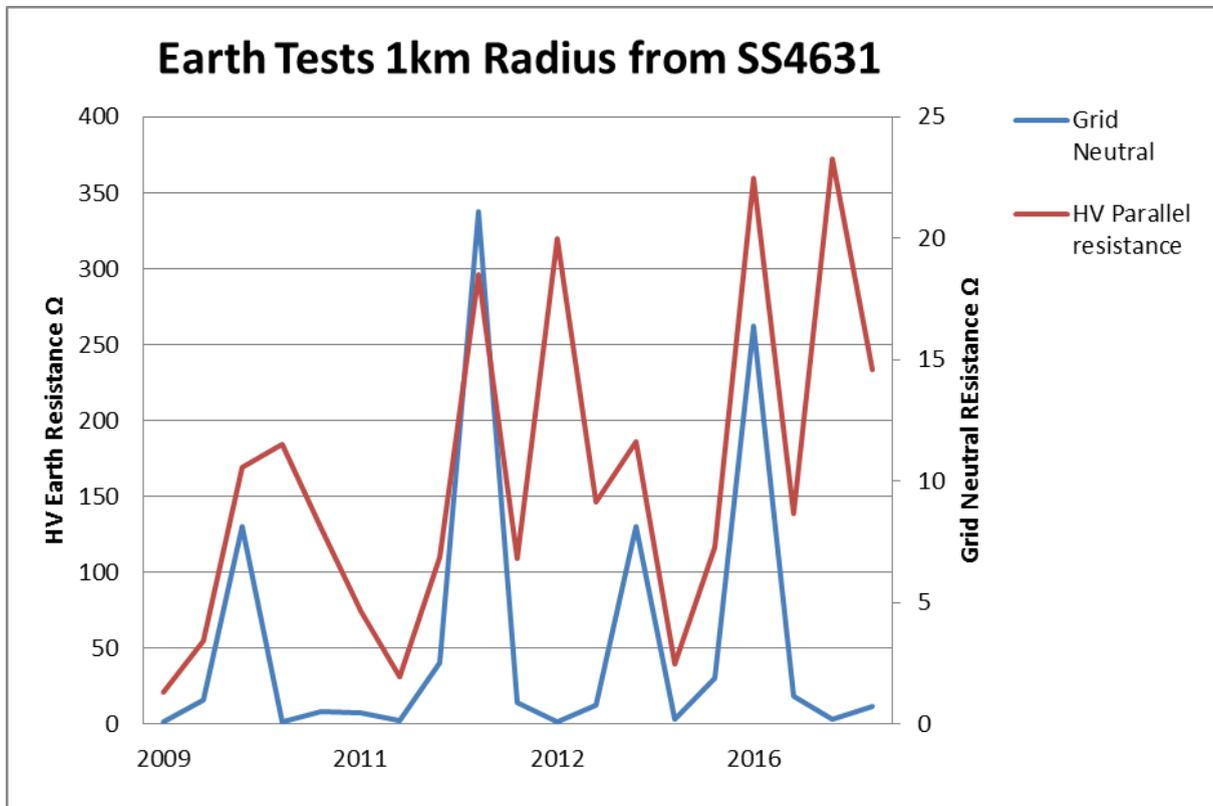
Figure 62: Earth Test History from 2009 to 2016 for SWER Distribution Transformers in a 1km Radius from SS4631
