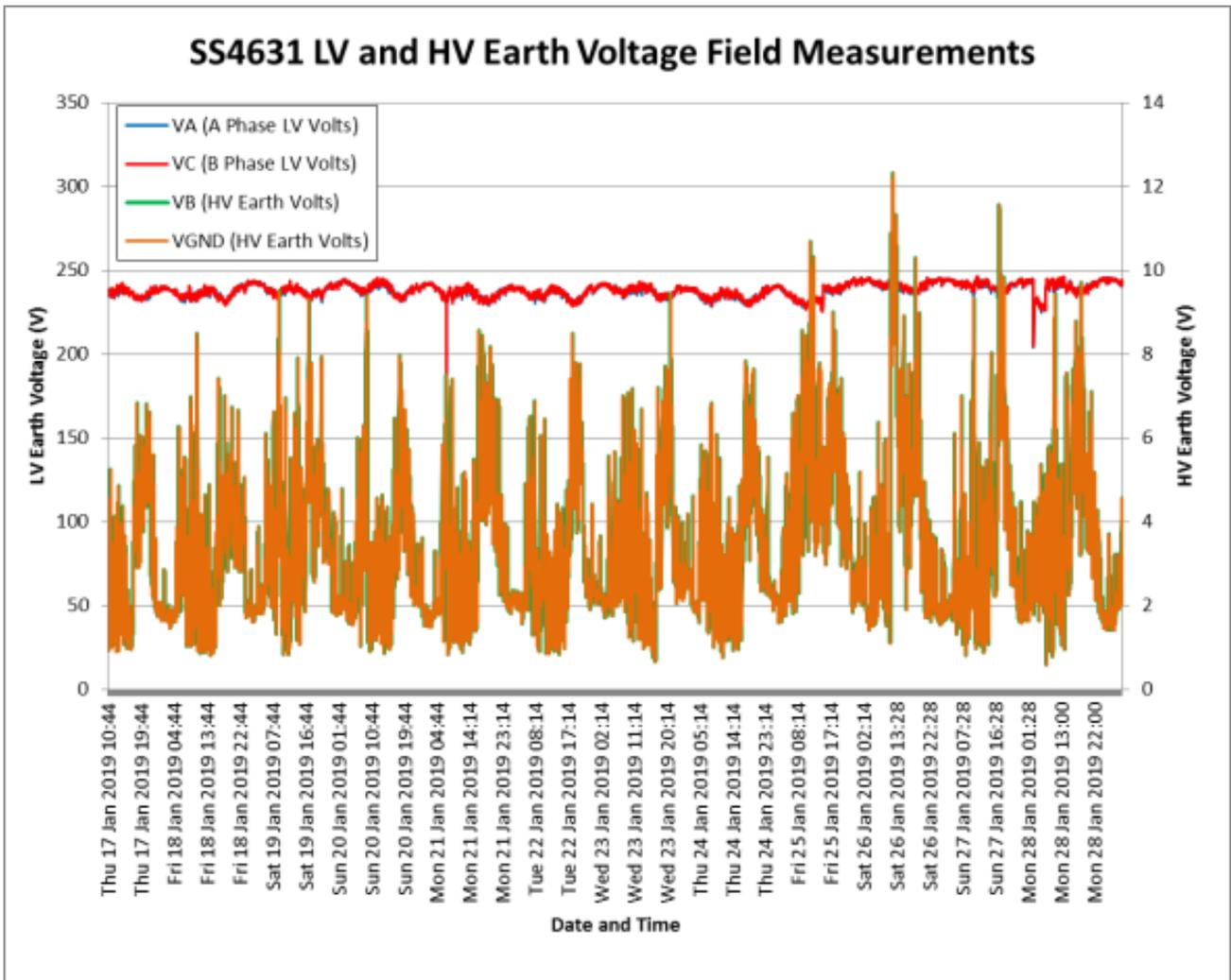
**Figure 79: PowerMonic PM45 Analyser Raw Voltage Data for SS4631**
