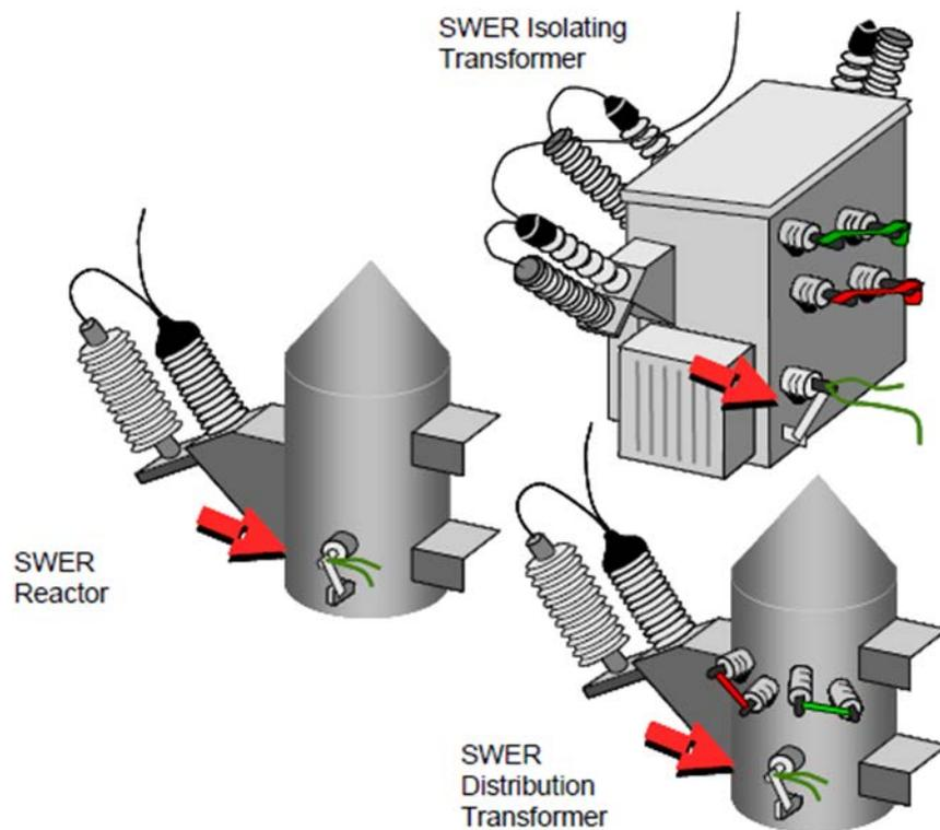
**Figure 53: Earth Return Terminal on SWER Transformers and Reactors (Ergon Energy 2017)**
