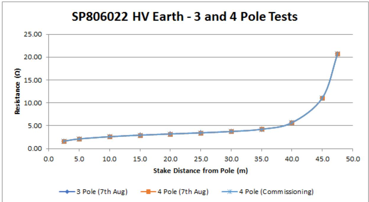
Figure 117: SP806022 HV Earth – 3 and 4 Pole Tests
