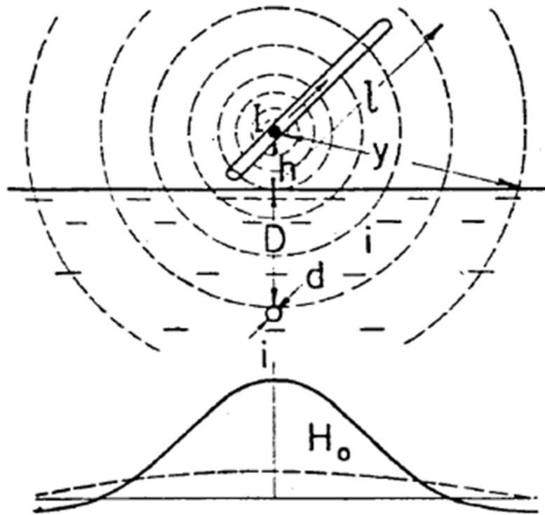
**Figure 39: Distribution of Ground-Return Currents Under AC Transmission Lines (Rudenberg 1945)**
