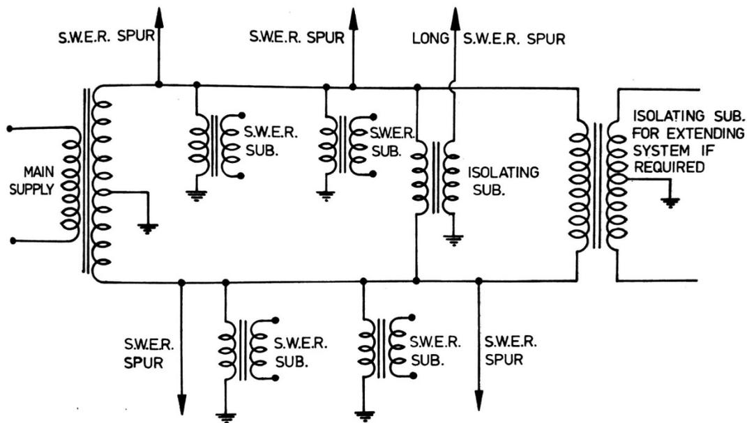
Figure 26: Duplex SWER System (The Electricity Authority of New South Wales 1978)
