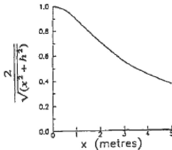
Figure 44: Normalised Surface Potential above a Spherical Electrode (Birtwhistle & Pearl 1997)
