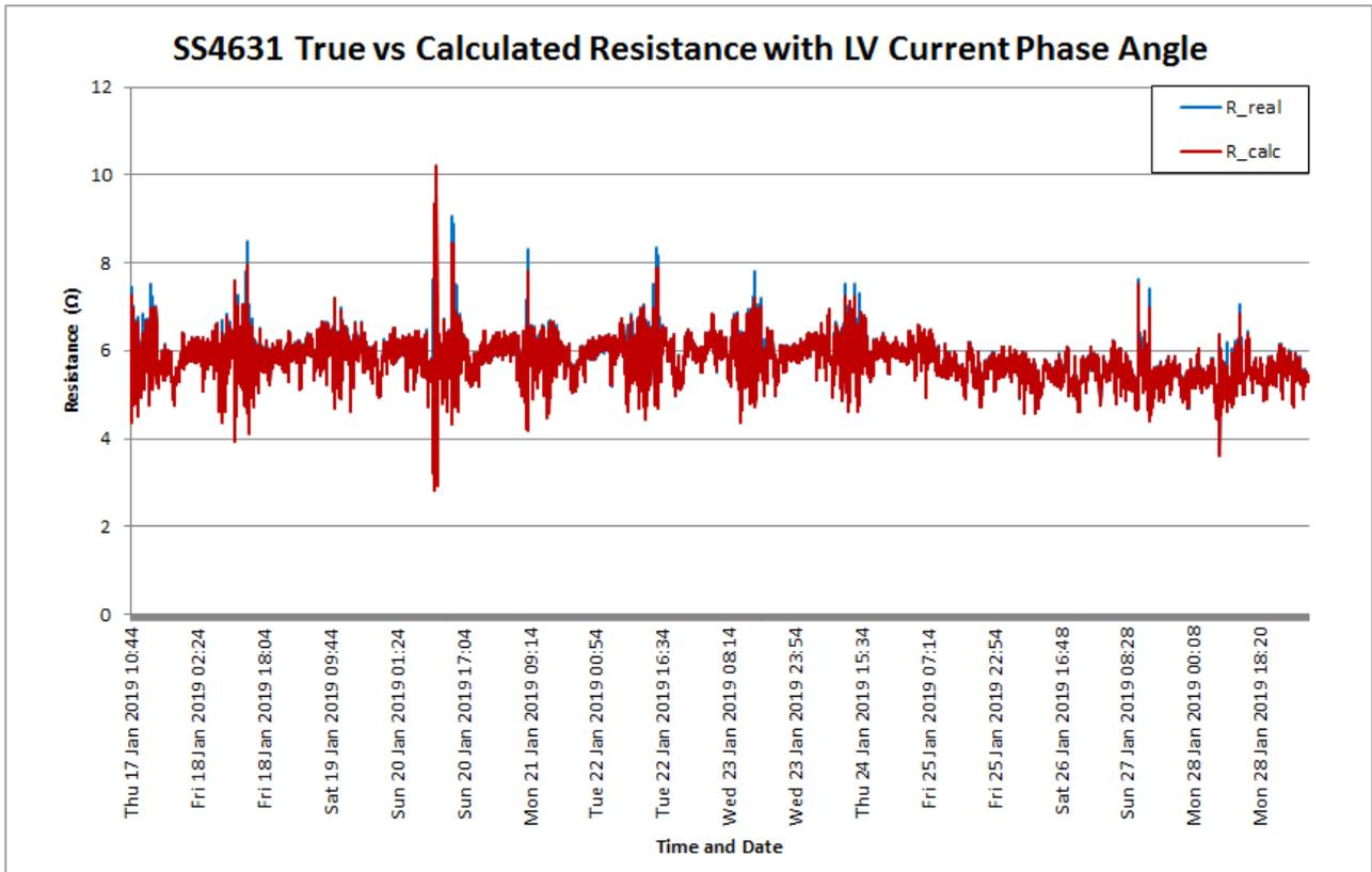
Figure 91: SS4631 True HV Earth Resistance vs Calculated HV Earth Resistance over 11 days with Phase Angle
