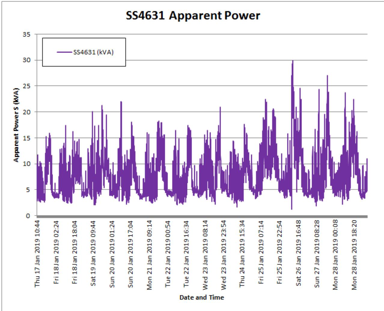
Figure 95: Apparent Power Calculations for SS4631 Field Test Data
