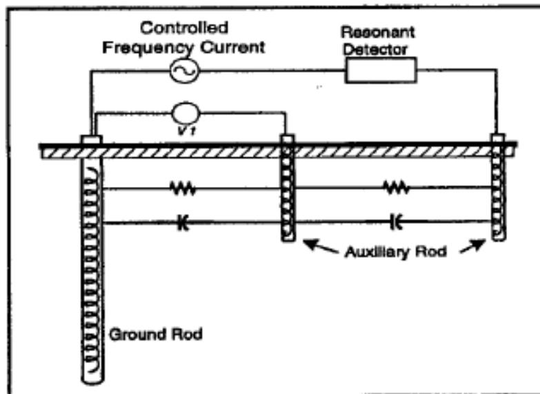
**Figure 18: Field Measurement Arrangement, Based on Modified Fall-of-Potential Method (Jambak, Ahmad, & Baker 2000)**
