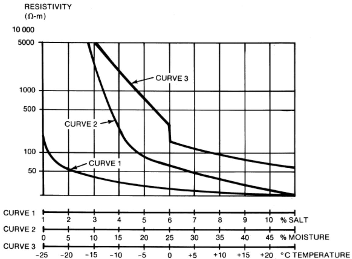
**Figure 4: Effect of Moisture, Temperature and Salt Upon Soil Resistivity (ANSI/IEEE 1984)**
