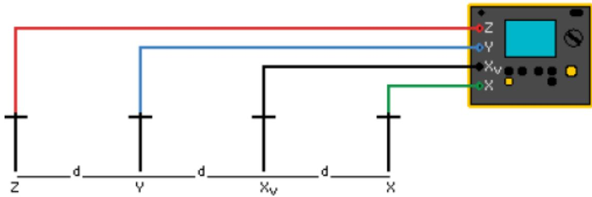
**Figure 58: Wenner Soil Resistivity Test Method (Ergon Energy 2017)**
