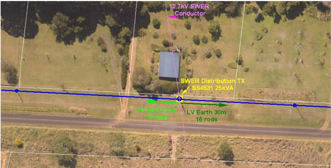
Figure 59: Aerial View of Earthing Configuration for SWER Distribution Transformer SS4631
