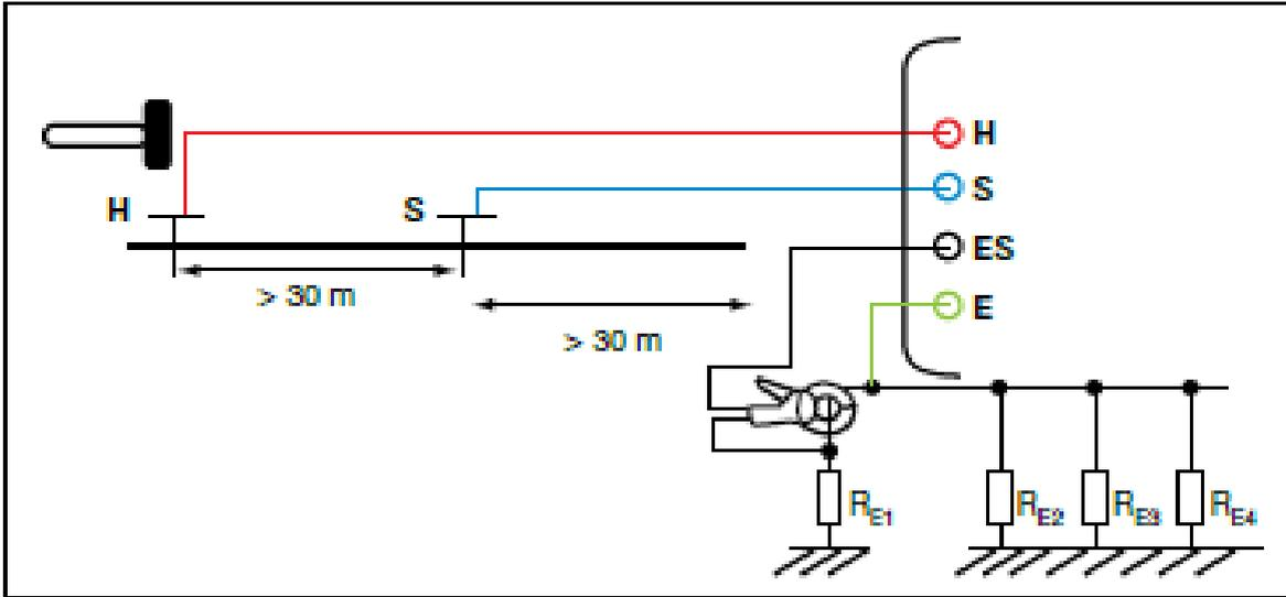
Figure 14: Selective 4-Pole Earth Resistance Measurement Method (Arnoux 2010)
