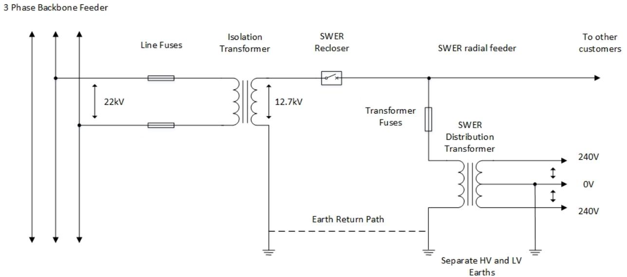
**Figure 25: Isolated SWER System Diagram (The Electricity Authority of New South Wales 1978)**
