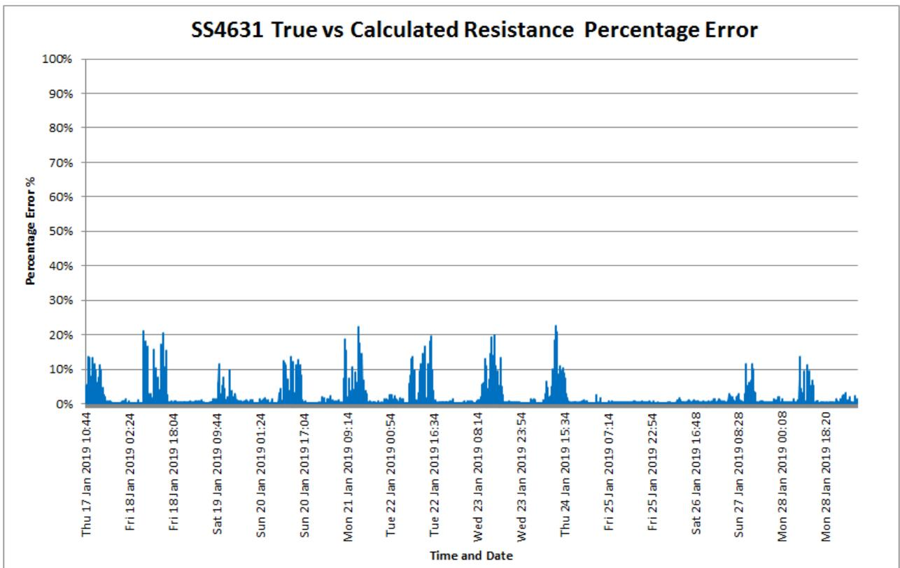
Figure 94: SS4631 True HV Earth Resistance vs Calculated HV Earth Resistance Error Plot for 20<sup>th</sup> January 2019
