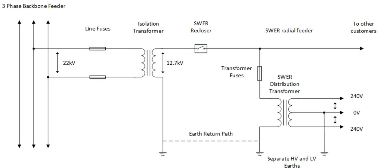
**Figure 2: Isolated SWER Network Configuration (The Electricity Authority of New South Wales 1978)**
