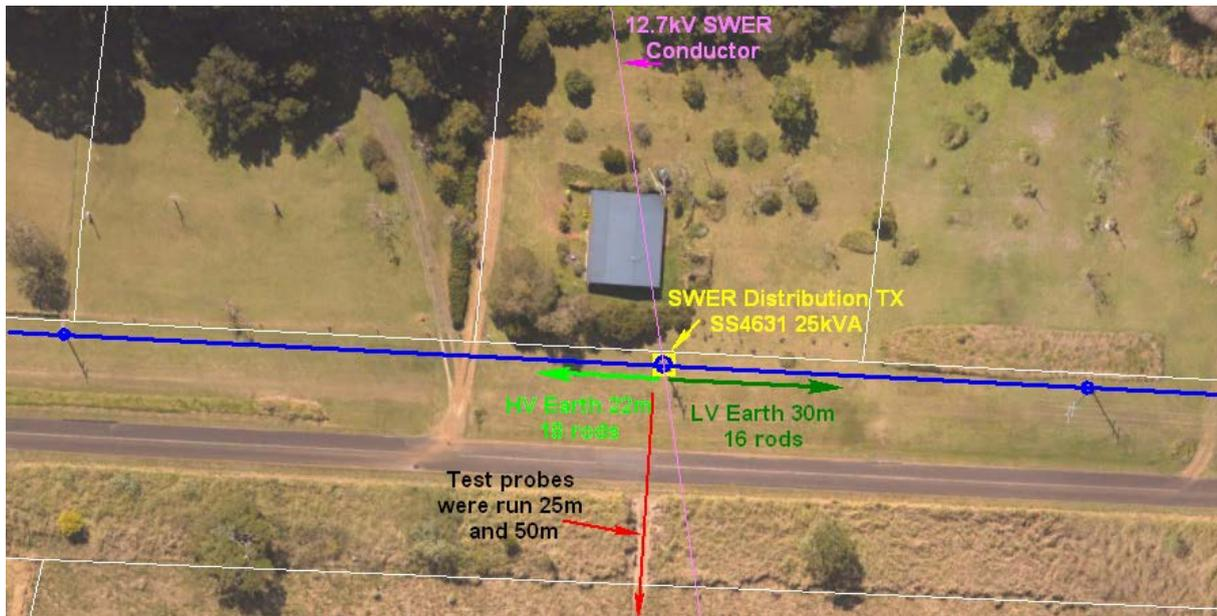
**Figure 72: SS4631 Earth Test Probes Arrangement**
