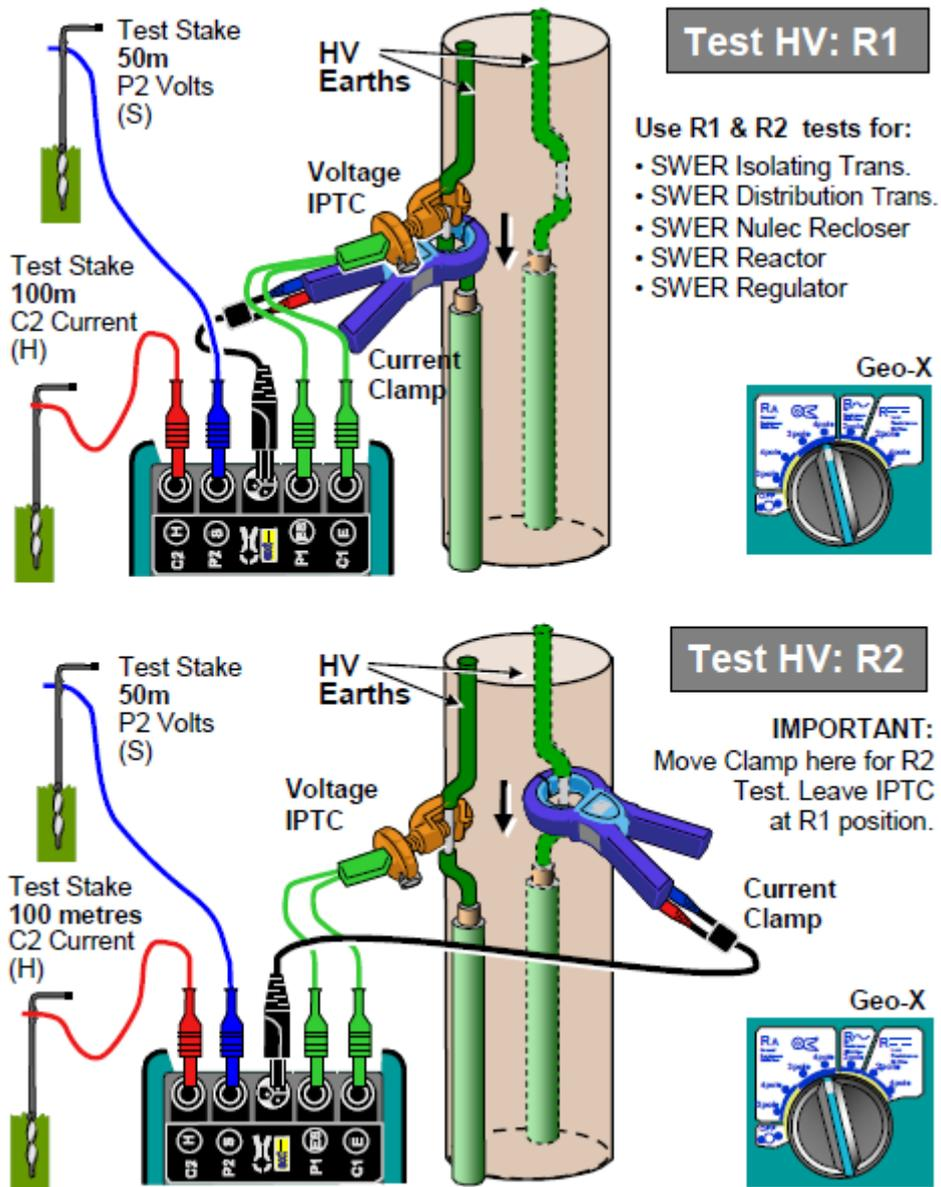
Figure 54: 4 Pole Selective SWER HV Earth Test Method (Ergon Energy 2017)
