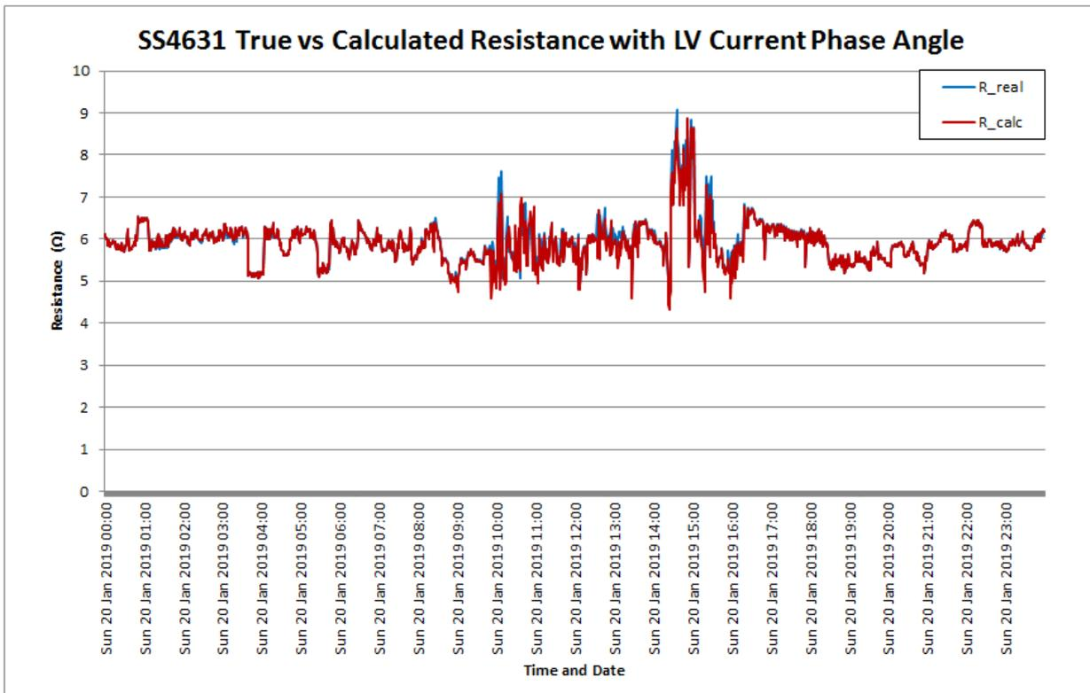
Figure 92: SS4631 True HV Earth Resistance vs Calculated HV Earth Resistance for 20<sup>th</sup> January 2019 with Current Phase Angle
