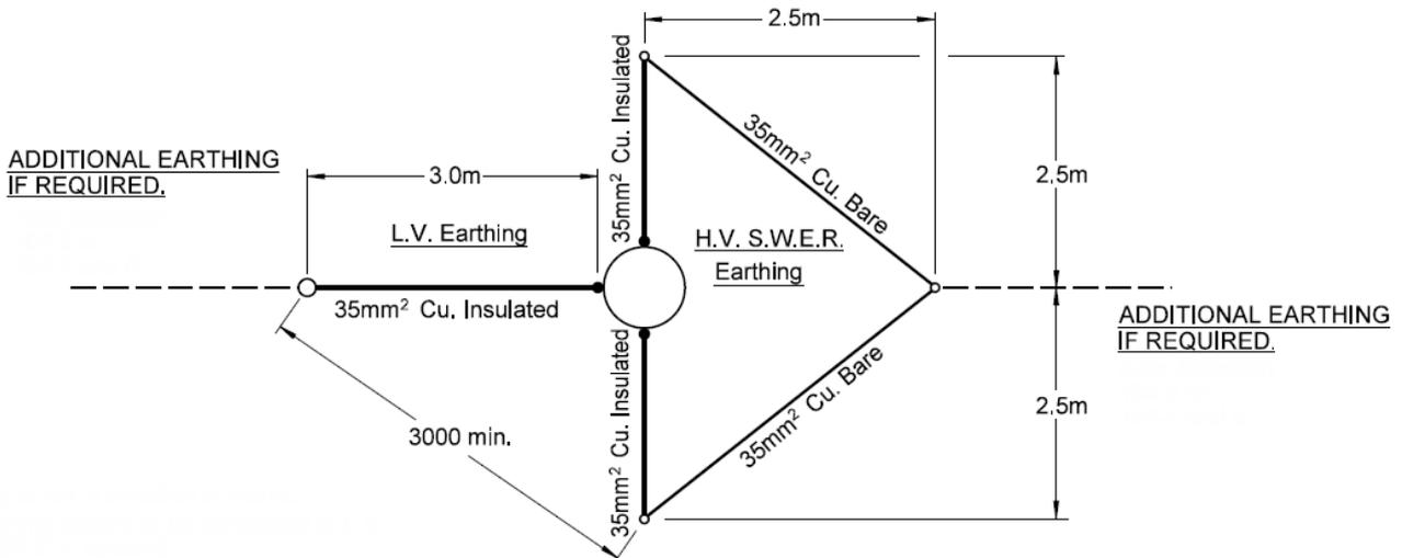
Figure 115: Standard SWER Distribution Earth Configuration
