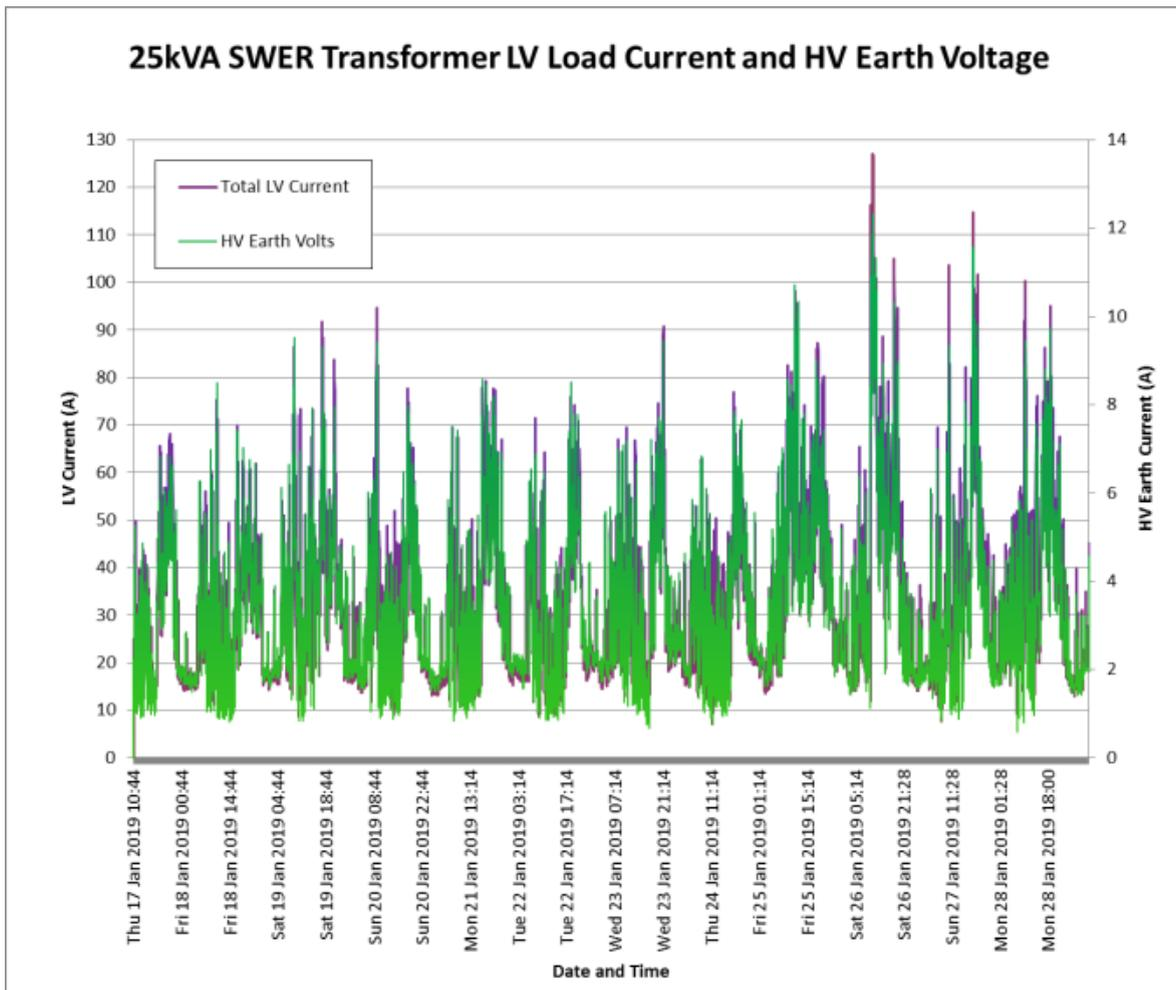
Figure 81: PowerMonic PM45 Analyser Total LV Load Current vs HV Earth Voltage for SS4631
