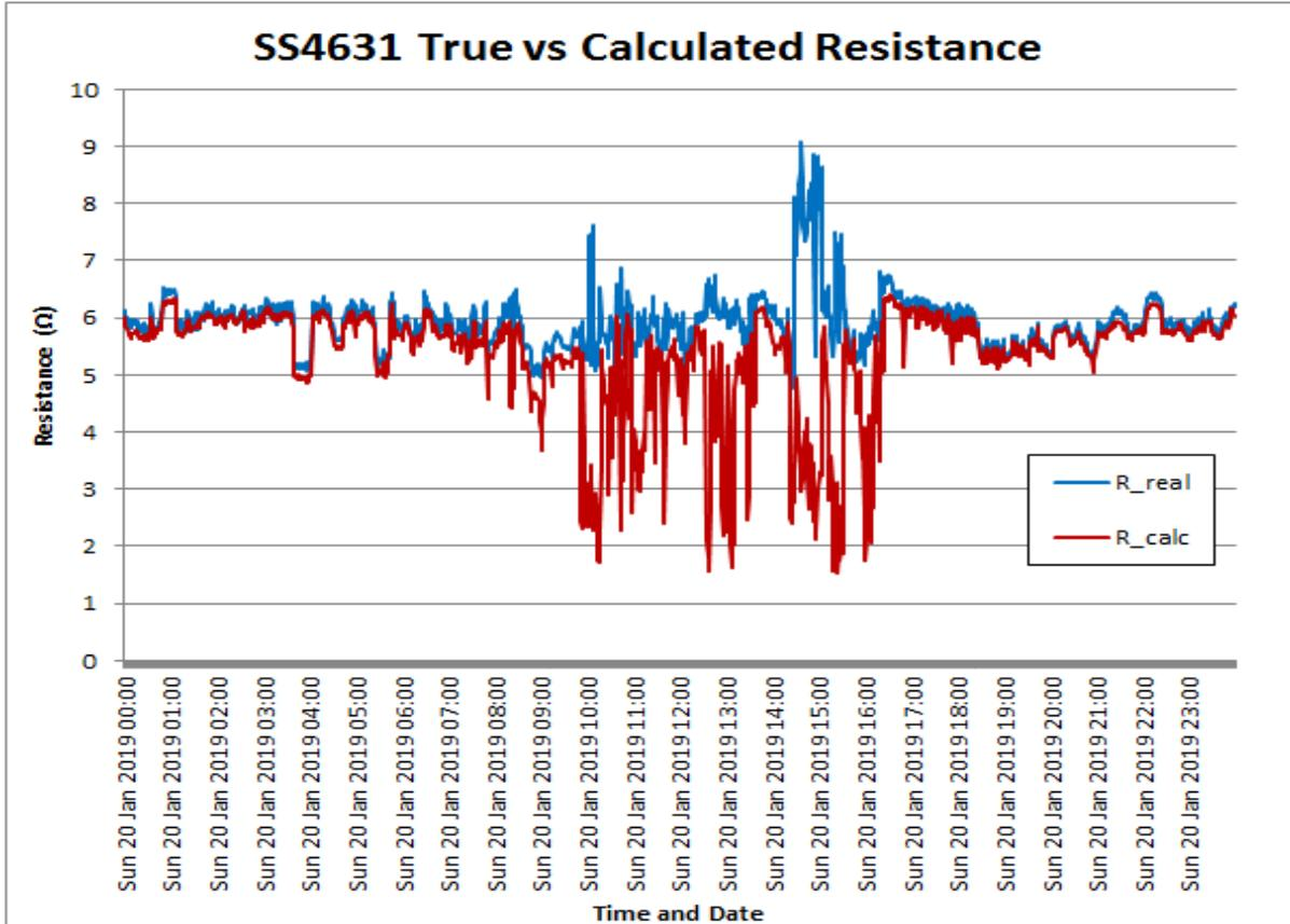
**Figure 85: SS4631 True HV Earth Resistance vs Calculated HV Earth Resistance for 20<sup>th</sup> January 2019**
