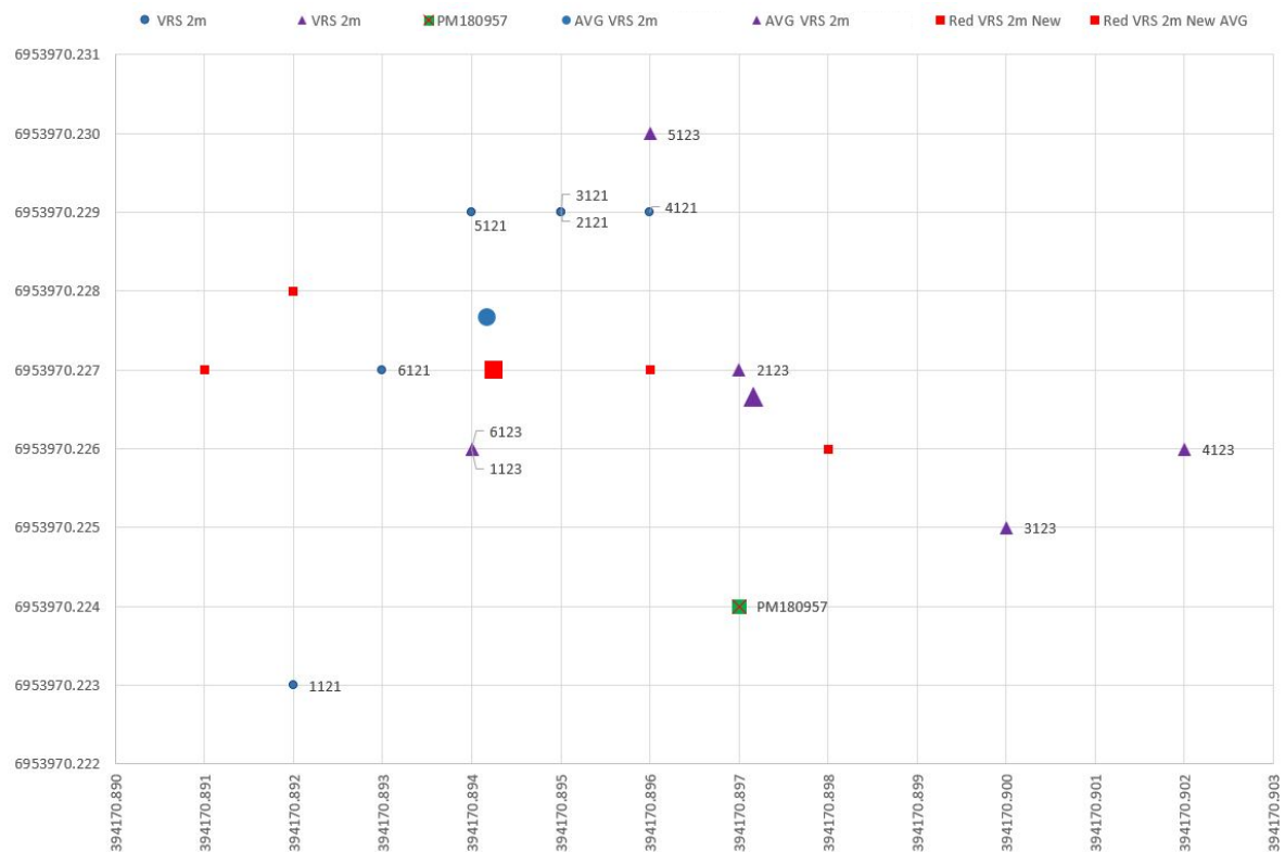
Figure 4.4: Scatter graph displaying the new red network VRS corrections and 120 epochs of data displayed with original blue and purple data sets and coordinates of PM180957 for reference.
