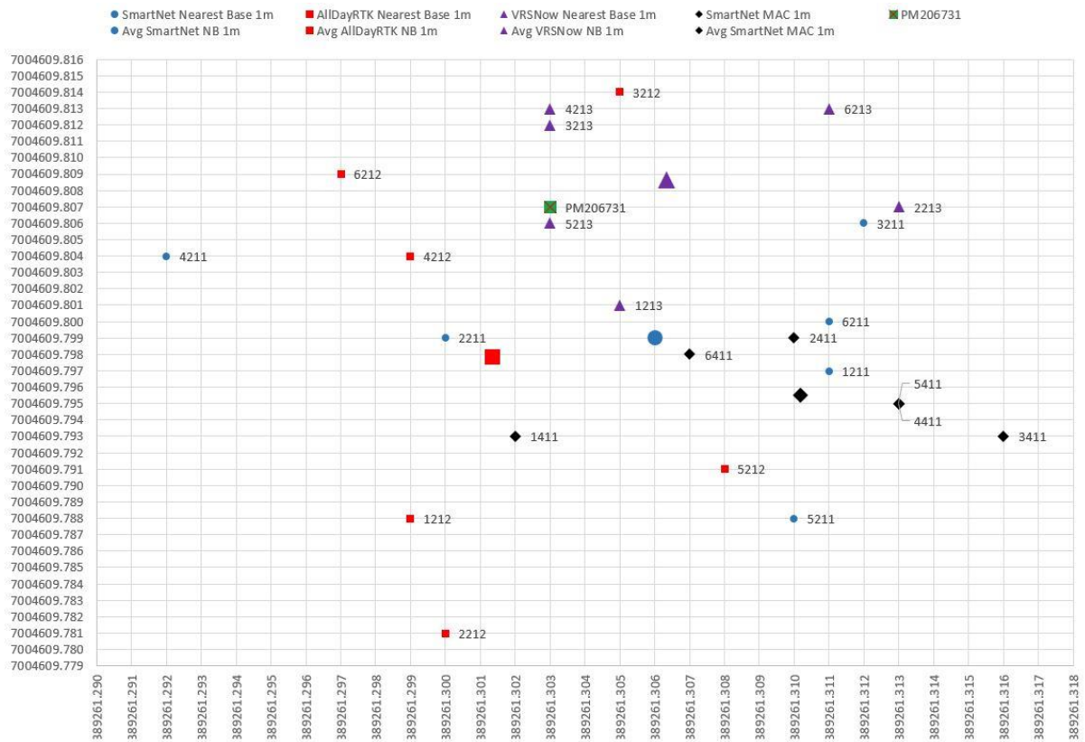
Figure 4.20: Scatter graph displaying MAC and Nearest Base corrections, all sampled with 60 epochs of data displayed with coordinates of PM206731 for reference. Larger icons represent the average of the 6 rounds of observations.
