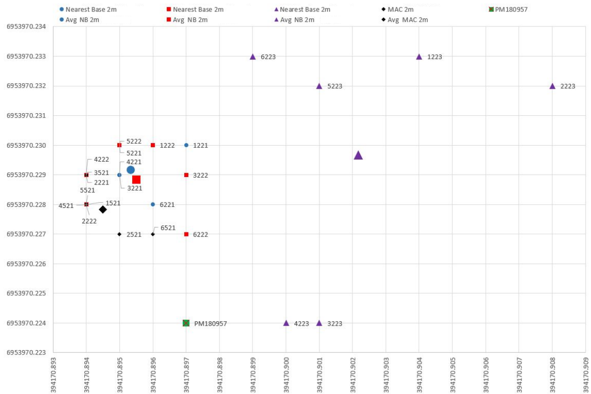
Figure 4.14: Scatter graph displaying MAC and Nearest Base corrections, all sampled with 120 epochs of data displayed with coordinates of PM180957 for reference. Larger icons represent the average of the 6 rounds of observations.
