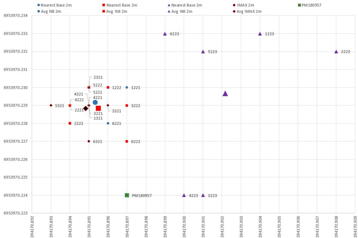
Figure 4.10: Scatter graph displaying IMAX and Nearest Base corrections, all sampled with 120 epochs of data displayed with coordinates of PM180957 for reference. Larger icons represent the average of the 6 rounds of observations.
