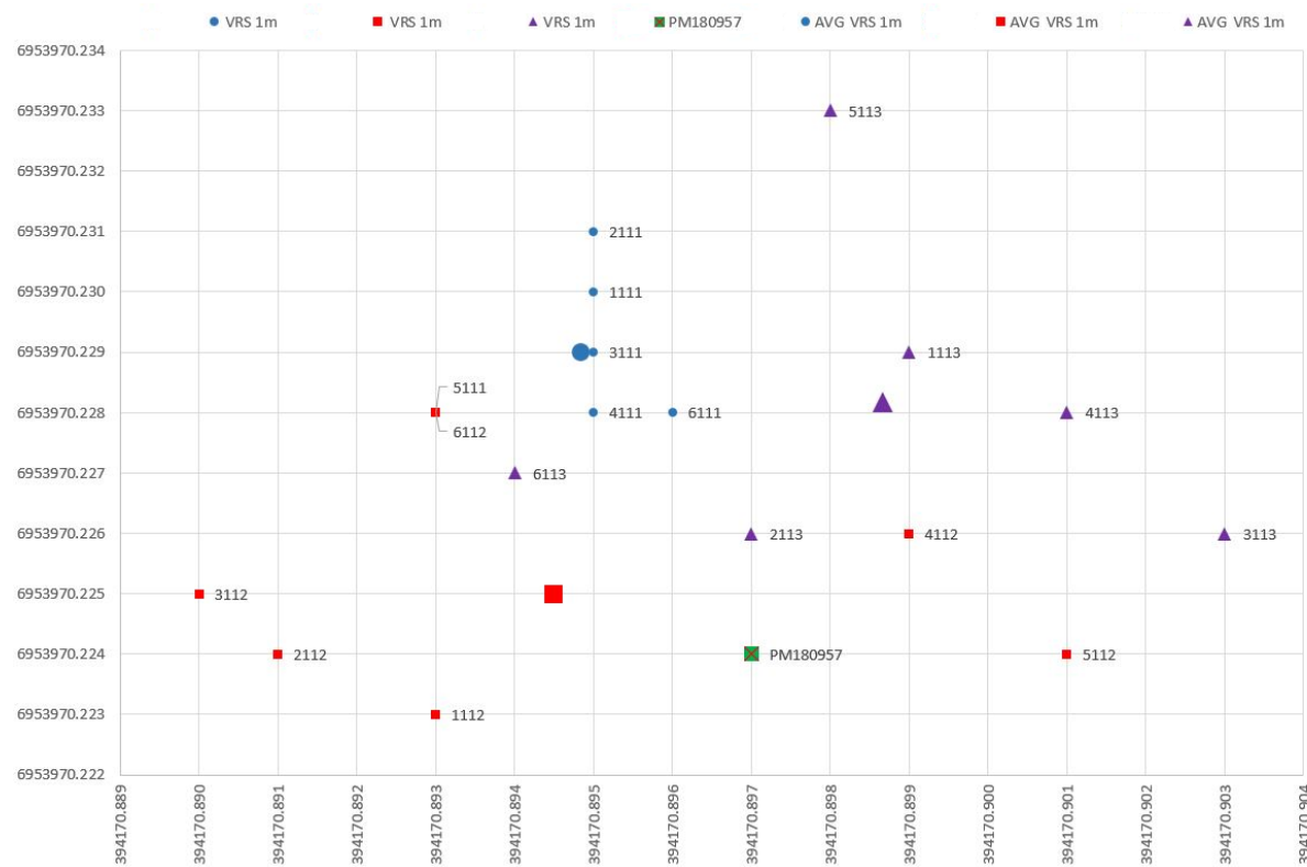
Figure 4.2: Scatter graph displaying VRS corrections and 60 epochs of data displayed with coordinates of PM180957 for reference. Larger icon represents the average of the 6 rounds of observations.
