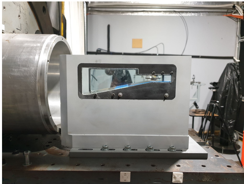
Figure 7.1: Side view of initial model mounted in TUSQ hypersonic wind tunnel
