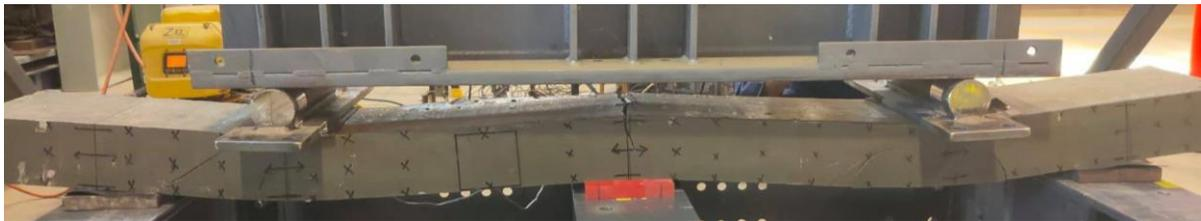
*Figure 6-2: Observed deflection at maximum applied load for the polymer concrete sleeper*
