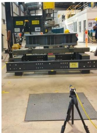
*Figure 6-1: The destructive test setup and the DIC device in front of load cell*
