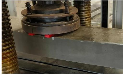
Figure 5-3: No cracks were developed in the polymer concrete sleeper during non-destructive testing
