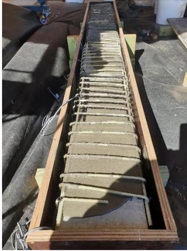
*Figure 4-5: The concrete core inside the GFRP reinforcement cage before the polymer concrete was poured*
