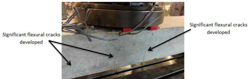
*Figure 5-2: Portland concrete sleeper developed flexural cracks during non-destructive testing*
