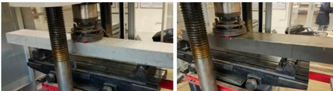
*Figure 5-1: Portland concrete sleeper under loading (left) and polymer concrete sleeper under loading (right)*
