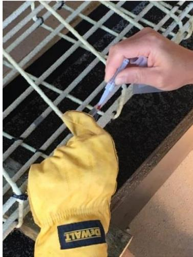
*Figure 4-3: Attaching strain gauges to the GFRP bars using super glue*
