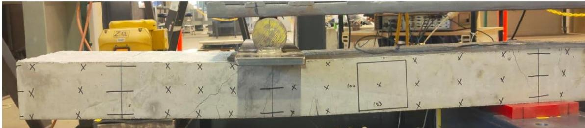
*Figure 6-3: Observed deflection at maximum applied load for the Portland concrete sleeper*
