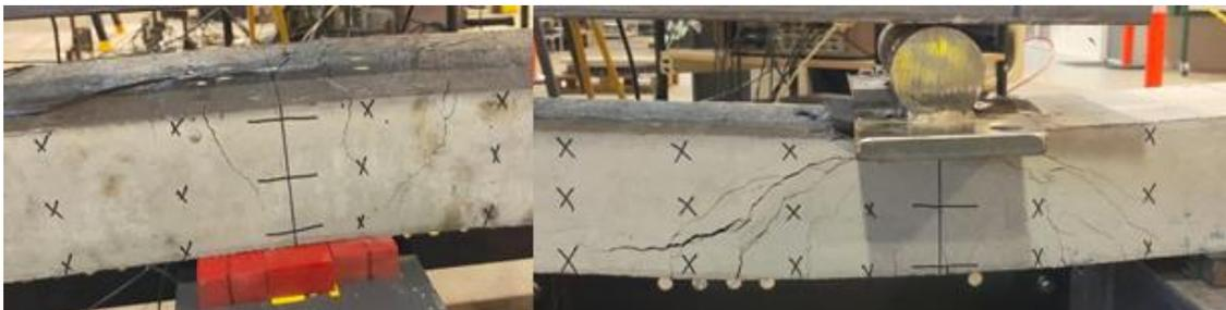
*Figure 6-4: Cracking observed in the Portland concrete sleeper at the middle support and the rail seat*
