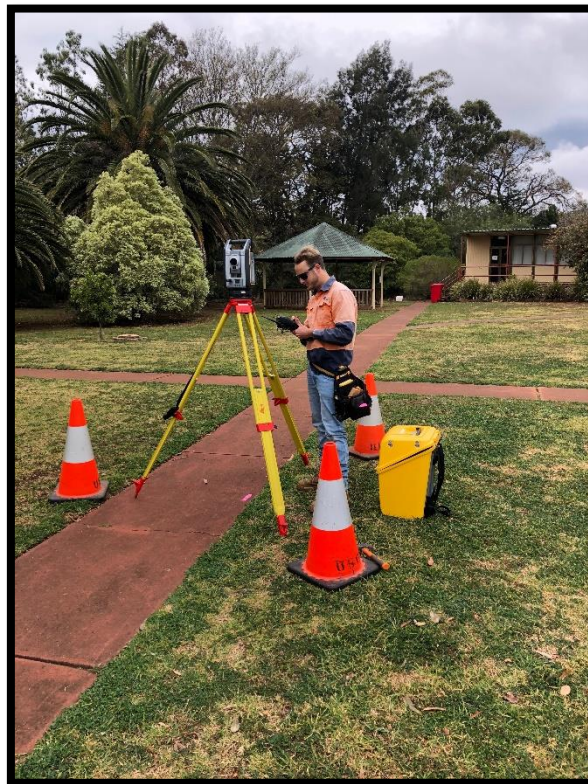
Figure 17 Traverse work being completed around Concannon
