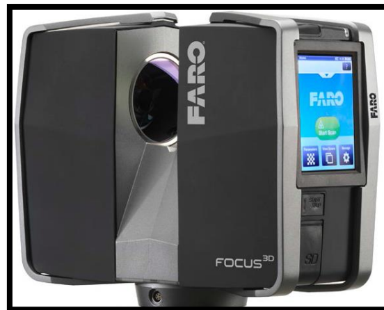
Figure 5 Faro Focus 3D S Series 120 (FARO, 2018)
