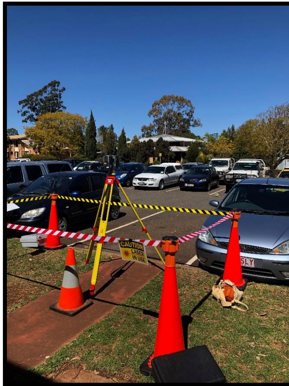
Figure 22 Laser Scanning work being completed around Concannon
