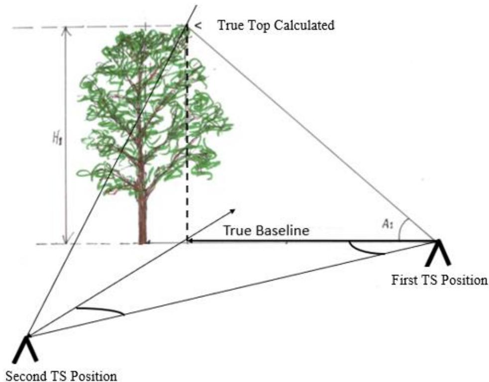
Figure 3.8: Measuring true height with two total stations, adapted from Koutar, Philippona & Spraggon (2018)
