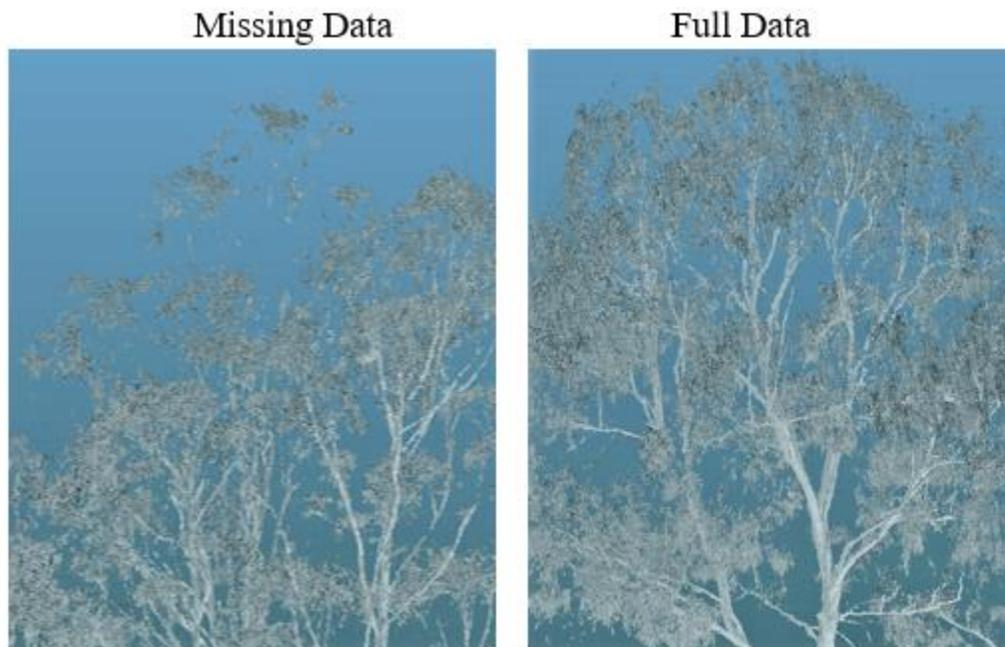
*Figure 4.11: Missing data in TLS scans*
