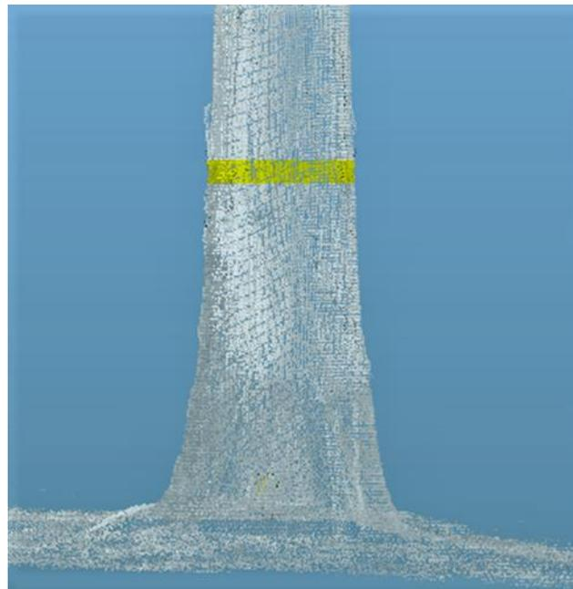
*Figure 3.4: Selection of points on tree stem of height 1.35-1.45m*
