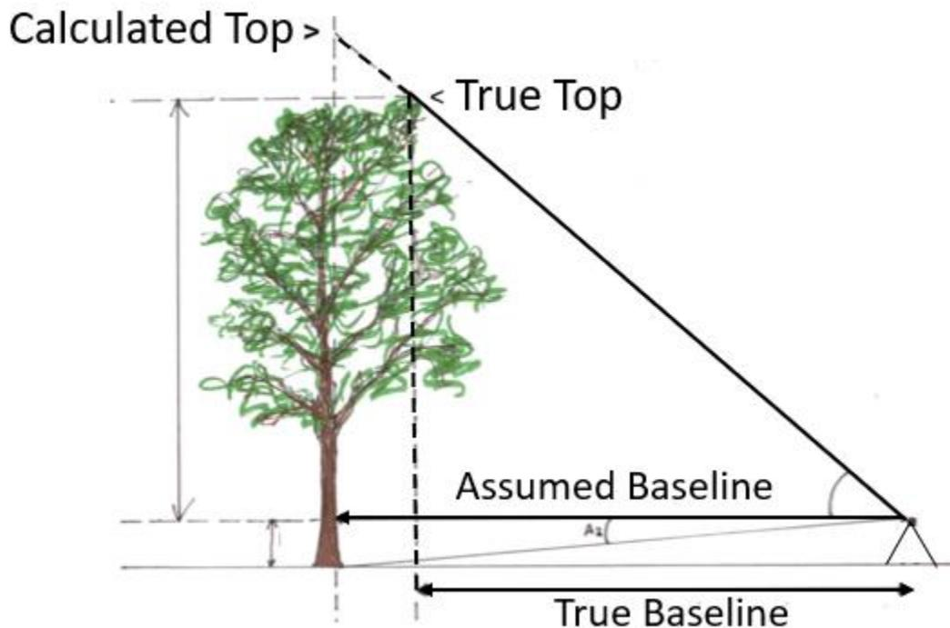
Figure 3.7: Height error with single TS setup (Koutar, Philippona & Spraggon 2018)
