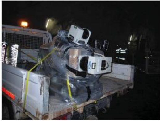
Figure 11: Scanner mount (Zlot & Bosse 2014, p.764).
