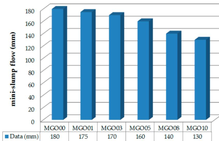
Figure 5.2: Mini slump test results (Liulei & Dong 2017)
