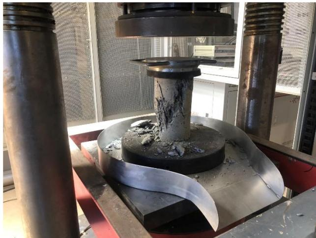
Figure 4.11: Compression test sample
