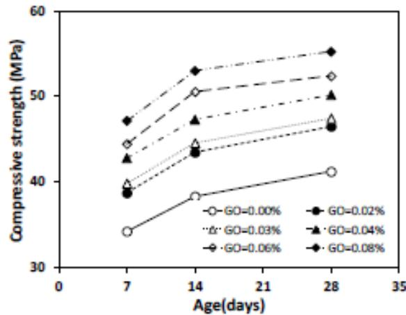
Figure 2.5: Compressive strength of concrete at different ages. Yu-You et al. (2019)
