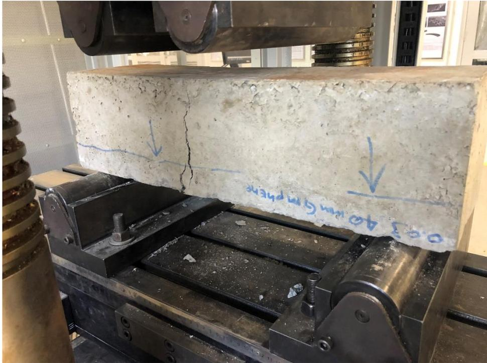
Figure 5.7: Flexural test sample after rapture load
