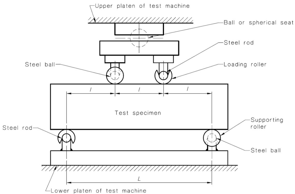
Figure 4.8: Diagrammatic view of a suitable flexure testing apparatus
