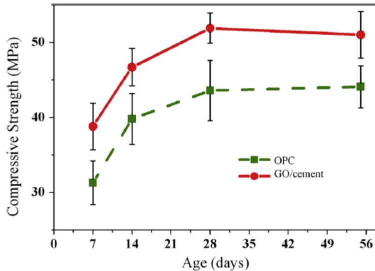
Figure 2.1: Compressive strength of Graphene Oxide cement compare to Ordinary Portland Cement. (Pan et al. 2015)
