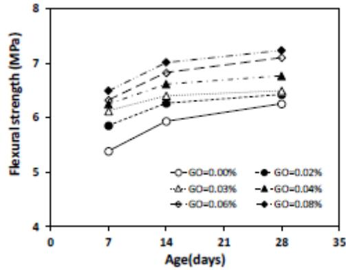
Figure 2.6: Flexural strength of concrete at different ages. (Yu-You et al. 2019)
