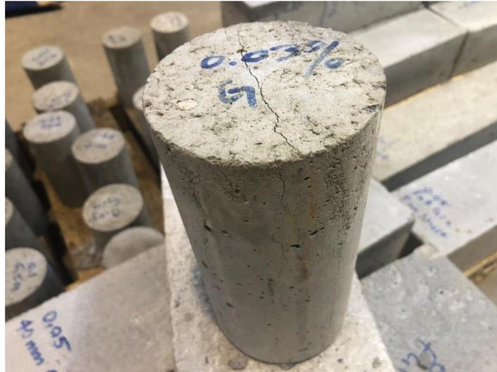
Figure 5.11: Indirect tensile test sample after rapture load
