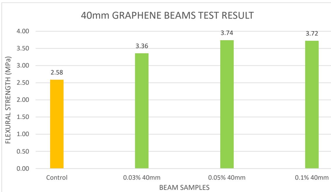
Figure 5.3: Flexural results for 40mm graphene beams
