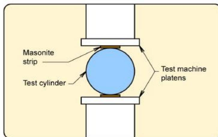
Figure 4.12: Indirect Tensile test
