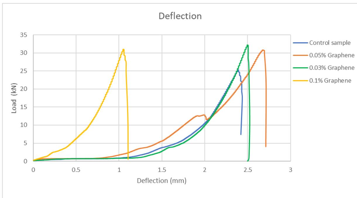
Figure 5.6: Deflections for flexural tests
