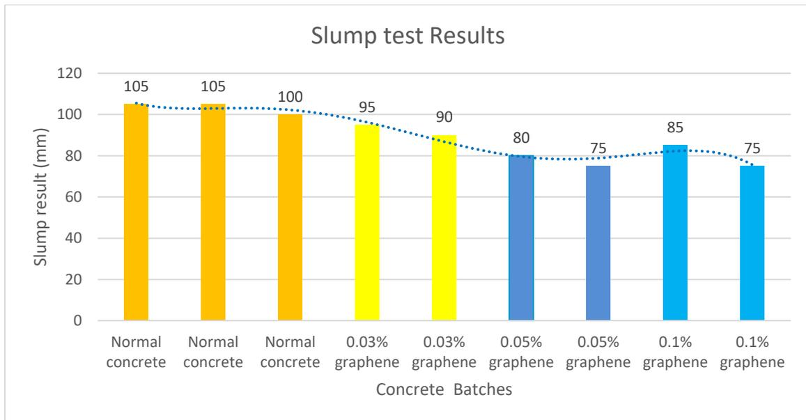
Figure 5.1: Slump test result graph
