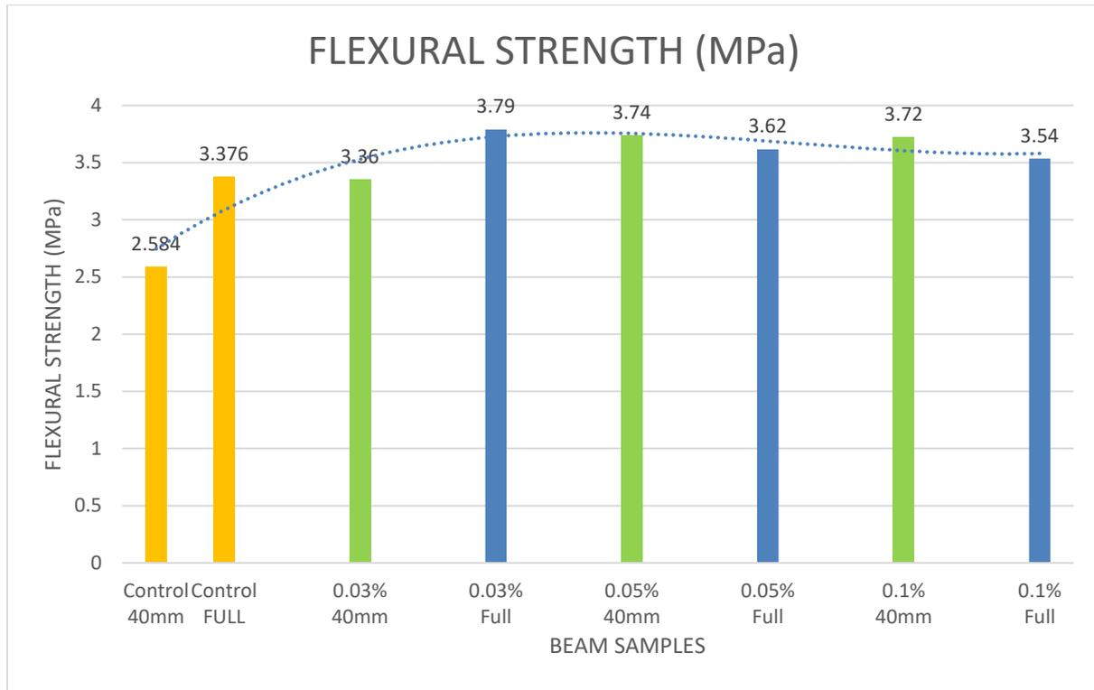
Figure 5.5: Flexural results for full and 40mm graphene beams
