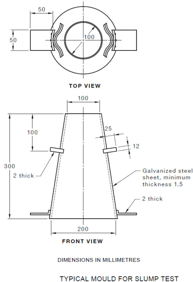
Figure 3.2: Typical mould for slump test. (AS 1012.3.1:2014)
