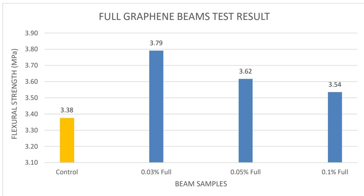
Figure 5.4: Flexural results for full graphene beams
