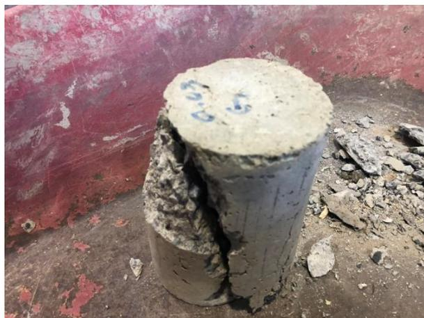
Figure 5.9: Compressive strength sample after rapture load
