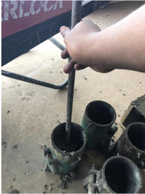
Figure 4.7: Cylinder moulding picture
