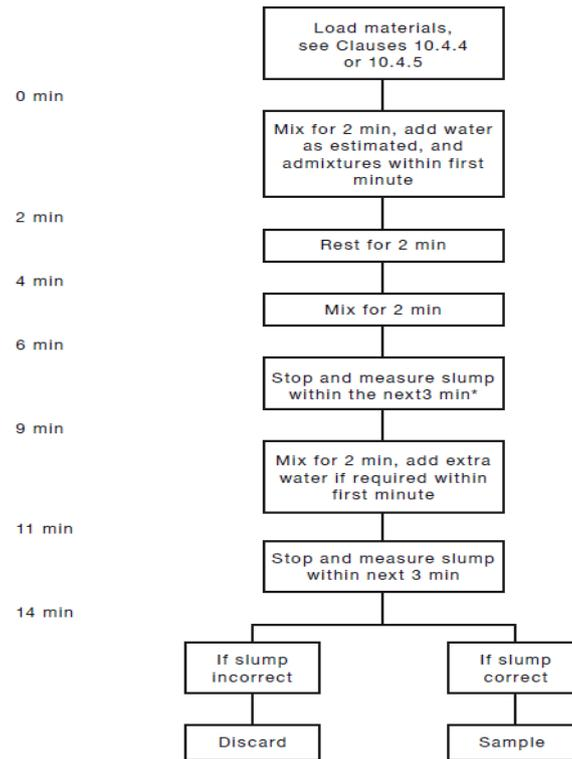
\* The concrete used in the slump test needs to be returned to the mixer.
