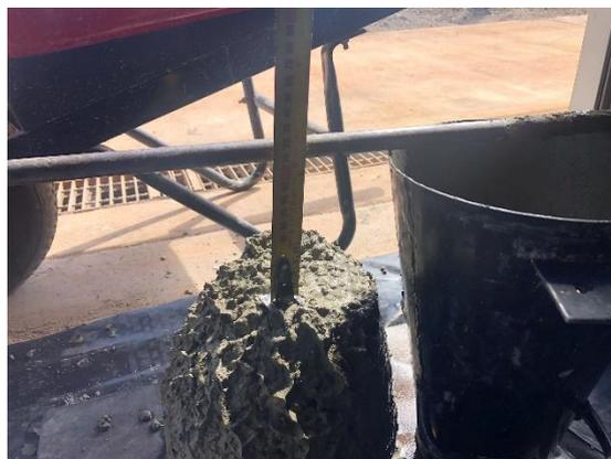
Figure 4.5: Slump test picture
