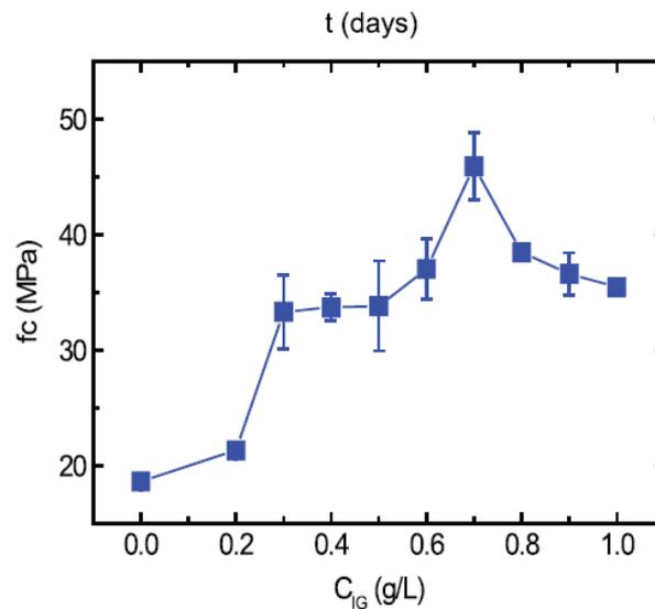
Figure 2.4: Compressive strength of Graphene reinforced concrete. (Dimov et al. 2018)
