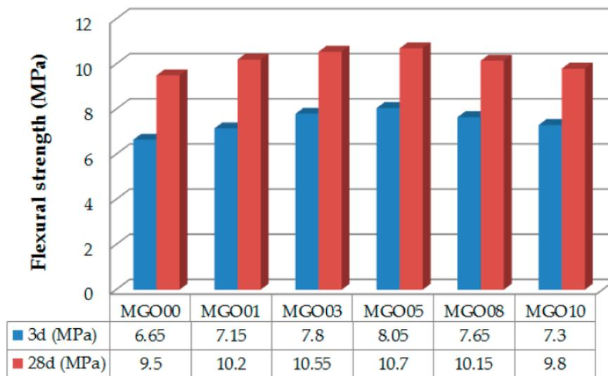
Figure 2.2: Flexural strength for 3 and 28 days (Liulei & Dong 2017)
