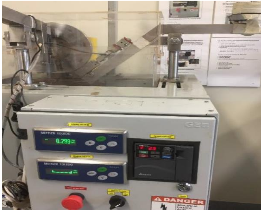
Figure 2.16. Multi-functional tribo-test machine (Alshammari et al., 2018)
