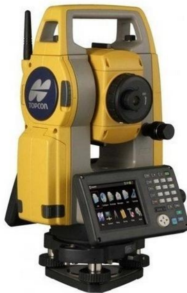
Figure 3.2 Topcon ES-105N Total Station (Shreeji Instruments, 2019)
