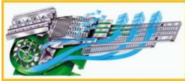
Figure 2.10: Diagram of the John Deere Cleaning System ( [John Deere Australia Web Site, 2005,] )
