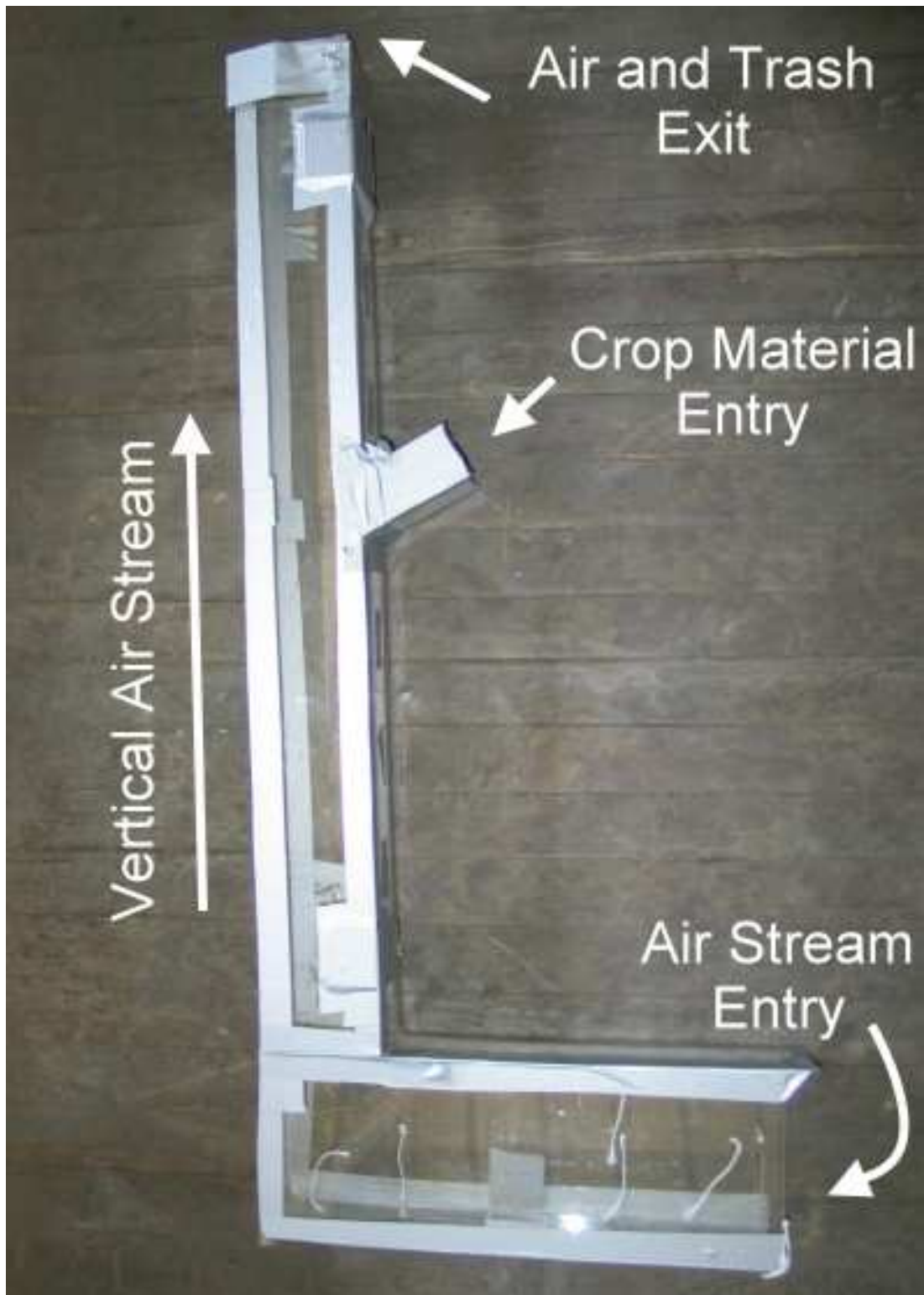
Figure 5.3: Prototype of the Sorting Chamber
